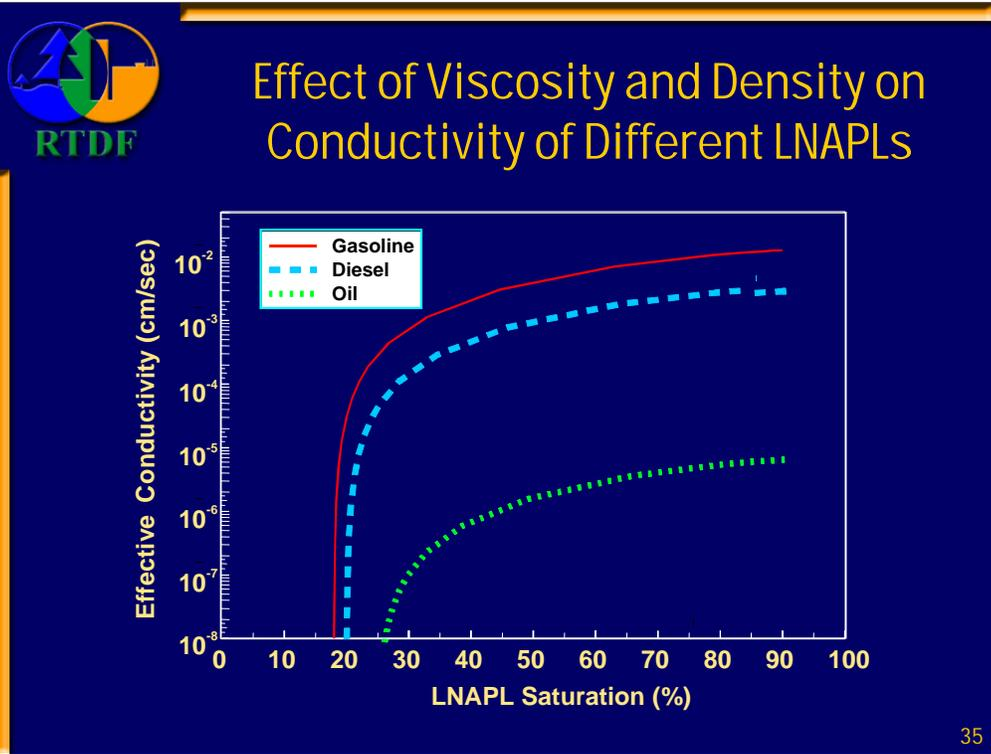
This figure illustrates how the density and viscosity of different LNAPLs affect their conductivity. Note that there are order-of-magnitude changes in conductivity as LNAPL saturation decreases.
