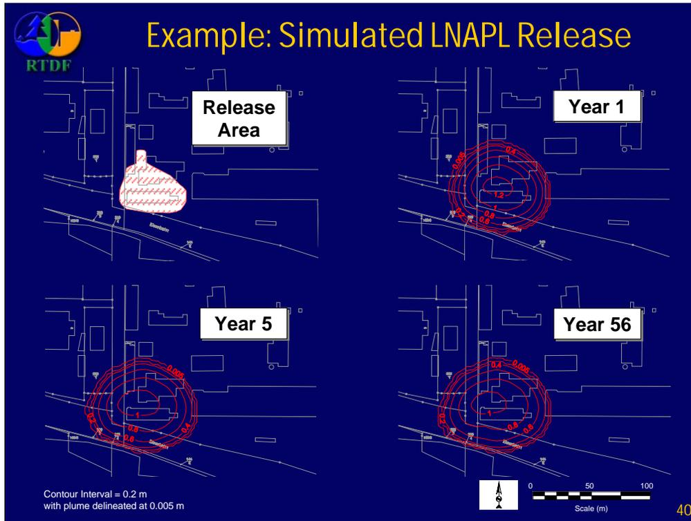
This figure shows the simulated migration of a plume of about 1,500 m<sup>3</sup> of LNAPL over 56 years. The images represent predicted well-product thickness measurements. While growth in the plume from release to Year 1 is clear, the plume appears to grow only slightly over the next 56 years.
