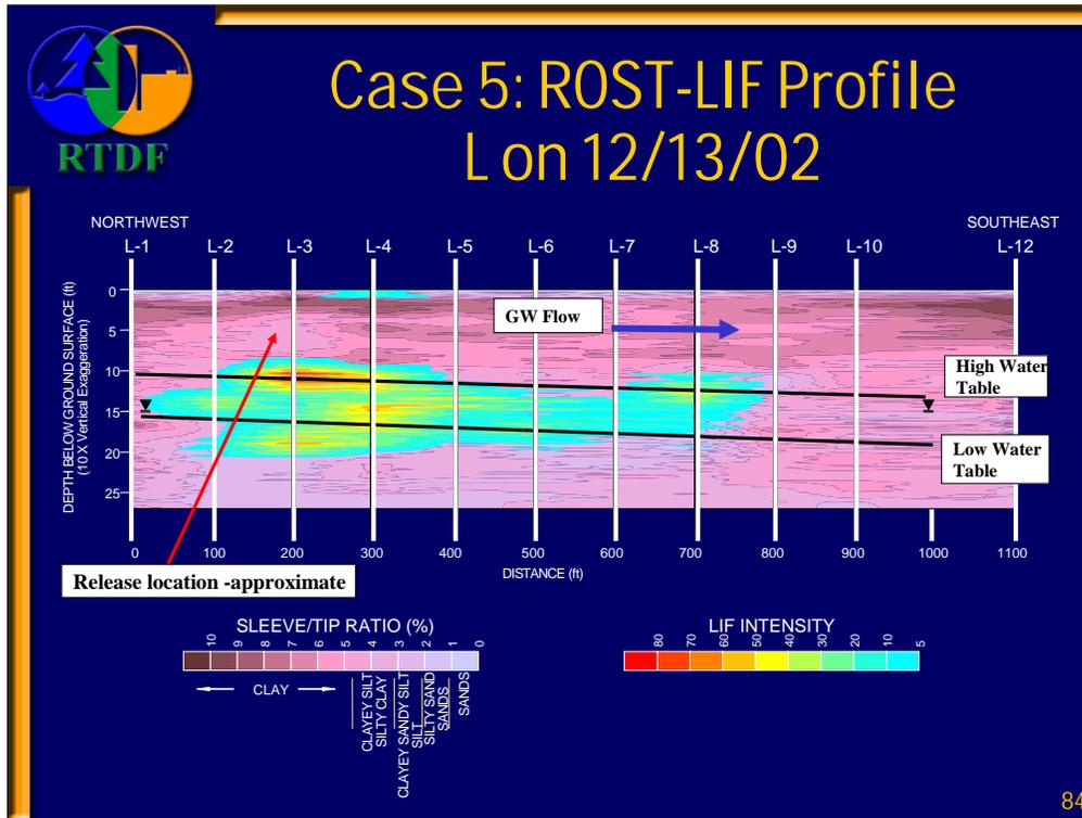
A profile of the release impacts as assessed using ROST/LIF are shown on this cross-section. It is superimposed over the geologic setting approximately two years after the release. Generally, the figure shows that higher saturations remain in the area near the release (in red and yellow) with thinner “fingering” occurring as the LNAPL migrated from the release area.
