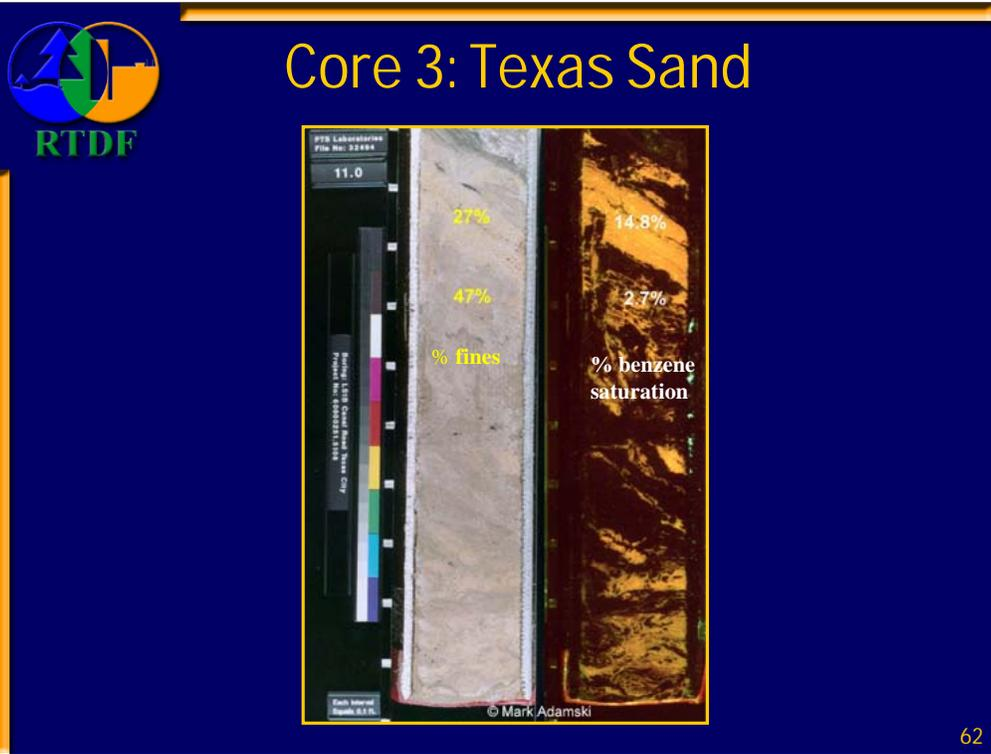
This photo shows a heterogeneous sand in Texas. The natural light photo shows significant heterogeneity, and the percent of fines has been indicated on the photo. In the right UV photo, the LNAPL, indicated by the light color, is present on the coarser grained materials.
