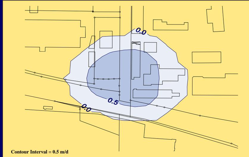
This slide shows the conductivity of the LNAPL. Note that there is LNAPL conductivity in the center, where LNAPL saturation is greater than residual saturation (and thus relative permeability is greater than zero). However, no conductivity is apparent at the edge where LNAPL saturation is less than or equal to residual saturation. Thus, a well at the center of the plume would be more likely to contain LNAPL that is recoverable than a well near the edge of the plume.
