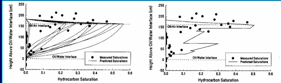
Predicted LNAPL saturations using capillary characteristic curve applied across entire LNAPL well thickness
