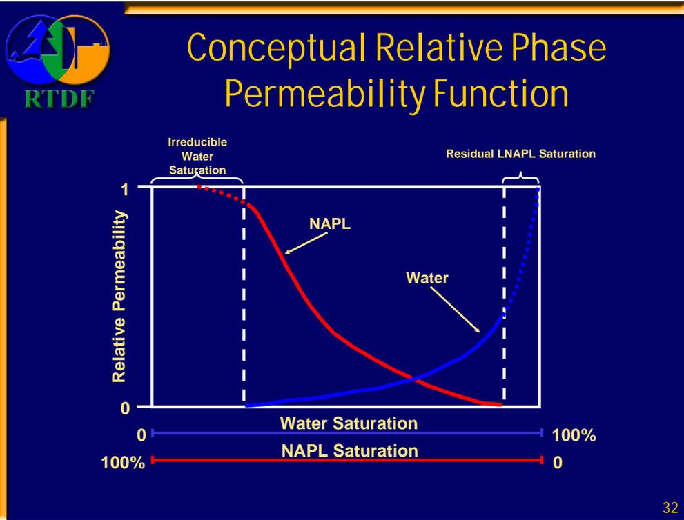
This figure shows conceptual relative permeability curves of the water (wetting) and the LNAPL (non-wetting) phases in a porous media as a function of their saturation. Perhaps it is easiest to understand these curves from the basis of the experiment that is run in order to measure the relative permeability. Remember: Relative permeability is a function of the saturation of the phase in the porous media.
