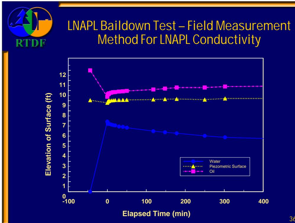
One way to check a LNAPL relative permeability estimate is with a **baildown test**. An LNAPL baildown test is performed and analyzed in much the same way as a water baildown test, but there are some important differences. First, instead of the water being evacuated from the well, only the LNAPL is removed. In practice, this is hard to do. We often try to do it with a vacuum truck rather than a bailer.
