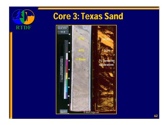
This photo shows a heterogeneous sand in Texas. The natural light photo shows significant heterogeneity, and the percent of fines has been indicated on the photo. In the right UV photo, the LNAPL, indicated by the light color, is present on the coarser grained materials.
