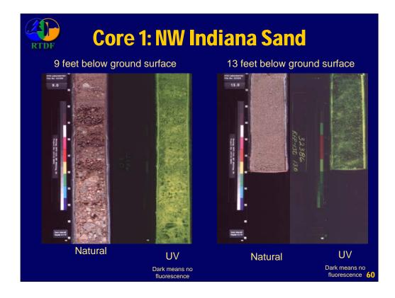
At this site, typical boring logs indicate a medium sand to about 17 feet below ground surface. The natural light photo on the left, at 9 feet below ground surface, shows that there is considerable gravel at that depth. However, over a substantial portion of the 17 feet, the core appears to be rather homogeneous like the natural light photo on the right, at 13 feet below ground surface.
