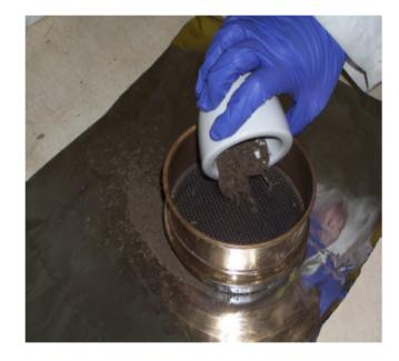
← Entire portion <2 mm subjected to grinding, then subsampling is conducted using a MSttechniquesinn the laboratory Care for cross contamination
