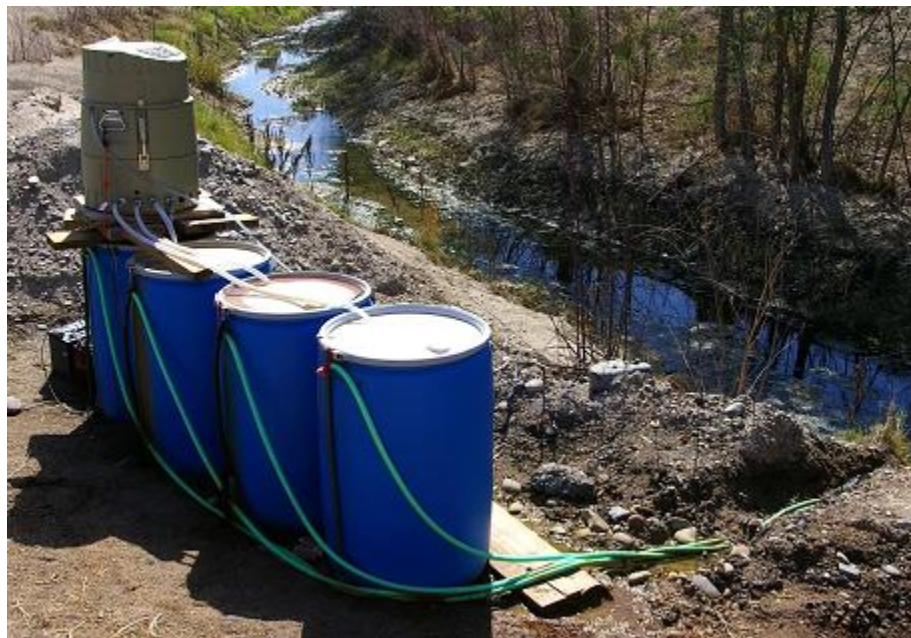
FIGURE 5-7 Passive Biochemical Reactor Test Source: Pahler et al., 2007
