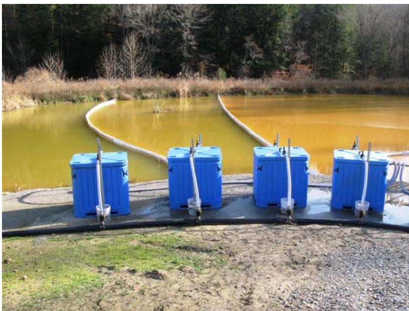
FIGURE 5-5 ZVI Pilot Test using Iron-Impregnated Foam as ZVI Media Source: Patriot Coal
