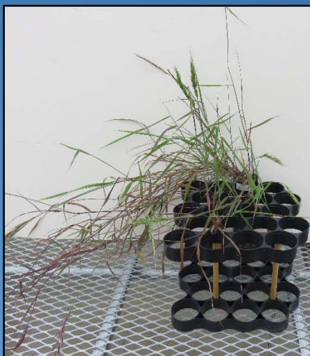
Soil + Lime + Biosolids + 1% Biochar
