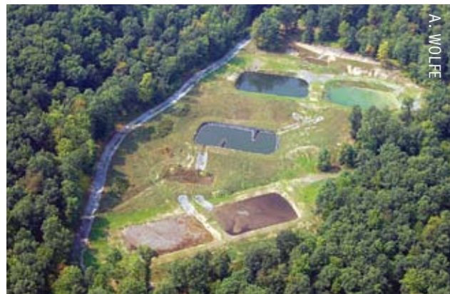
Middle Branch passive treatment system
