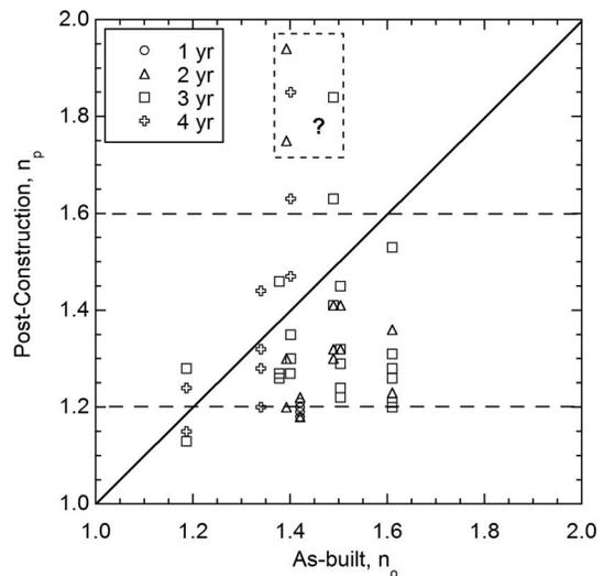
**Fig. 10.** Postconstruction  $n$  parameter ( $n_p$ ) versus  $n$  in the as-built condition ( $n_o$ ). Outliers (“?”) for sites in Albany, Ga. (Table 4), Boardman, Ore. (Table 5), and Polson, Mont. (Table 6).
