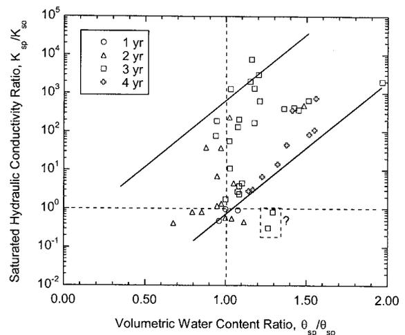
**Fig. 7.** Ratio of postconstruction saturated hydraulic conductivity relative to as-built saturated hydraulic conductivity ( $K_{sp}/K_{s0}$ ) versus ratio of postconstruction saturated volumetric water to as-built saturated volumetric water content ( $\theta_{sp}/\theta_{s0}$ ). Trend lines drawn by eye. Outliers (“?”) are for site in Helena, Mont. (Table 5).
