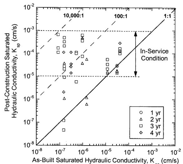
**Fig. 4.** Postconstruction saturated hydraulic conductivity ( $K_{sp}$ ) versus as-built saturated hydraulic conductivity ( $K_{s0}$ ). The band labeled “in service” indicates range for soils after 2–4 years of exposure to site environmental conditions.
