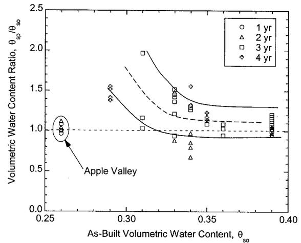
**Fig. 6.** Ratio of postconstruction saturated volumetric water content to as-built saturated volumetric water content ( $\theta_{sp}/\theta_{s0}$ ) versus as-built saturated volumetric water content ( $\theta_{s0}$ ). Trend lines drawn by eye.
