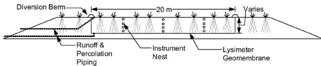
**Fig. 1.** Typical cross section of ACAP test section along the centerline. The lysimeter is 10 m × 20 m. The top deck of the test section is 30 m long and 20 m wide.
