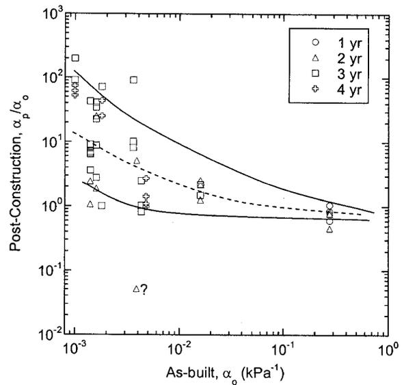
**Fig. 9.** Ratio of postconstruction  $\alpha$  relative to  $\alpha$  in as-built condition ( $\alpha_p/\alpha_o$ ) versus  $\alpha$  in as-built condition ( $\alpha_o$ ). Trend lines drawn by eye. Outlier (“?”) for site in Albany, Ga. (Table 4).
