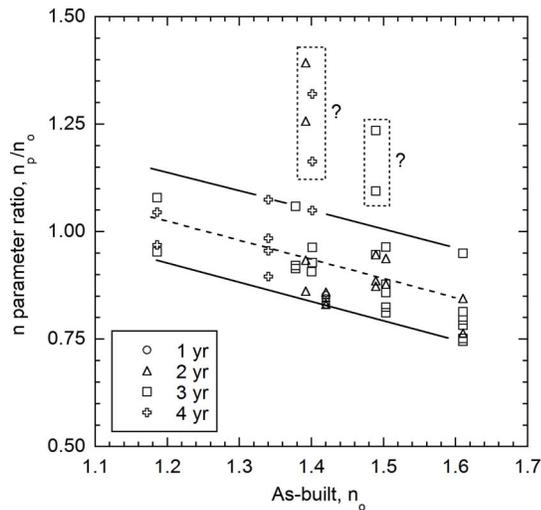
**Fig. 11.** Ratio of postconstruction  $n$  to as-built  $n$  ( $n_p/n_0$ ) versus as-built  $n$  ( $n_0$ ). Trend lines drawn by eye. Outliers (“?”) for sites in Albany, Ga. (Table 4), Boardman, Ore. (Table 5), and Polson, Mont. (Table 6).
