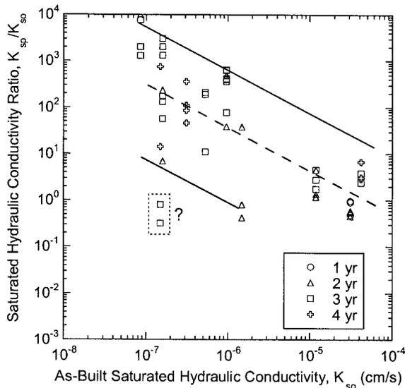
**Fig. 5.** Ratio of postconstruction saturated hydraulic conductivity relative to as-built saturated hydraulic conductivity ( $K_{sp}/K_{s0}$ ) versus as-built saturated hydraulic conductivity ( $K_{s0}$ ). Trend lines drawn by eye. Outliers (“?”) are for site in Helena, Mont. (Table 5).
