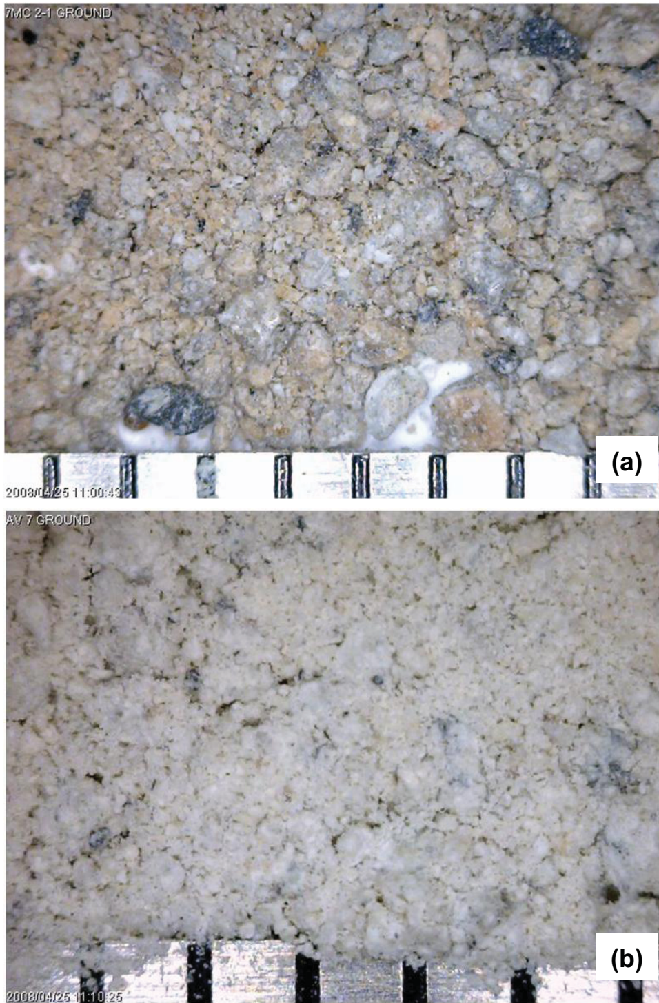
Fig. N. 5. Ground bentonite passing No. 20 sieve from Site E (a) and Site A (b).
