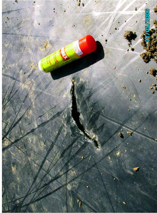
Fig. A.53 Close-up of unintentional hole from installation found via geophysical investigation.
