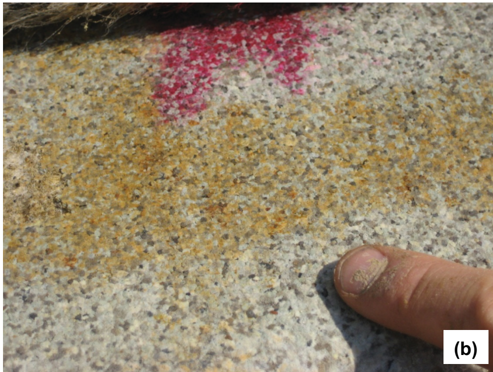
Fig. M. 15. GCL overlap: (a) match point along marks on original product and (b) close up showing hydrated bentonite granules in the overlap.
