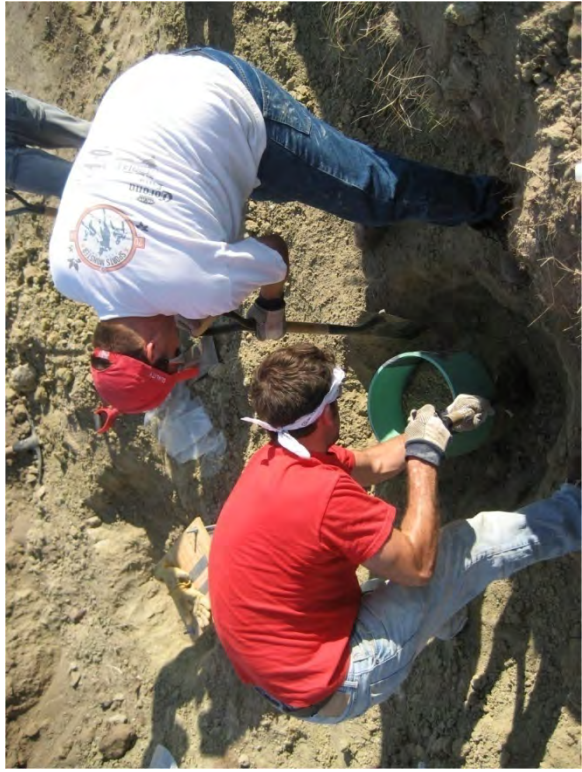
Fig. A.14. Filling SDRI, inner cap visible.
