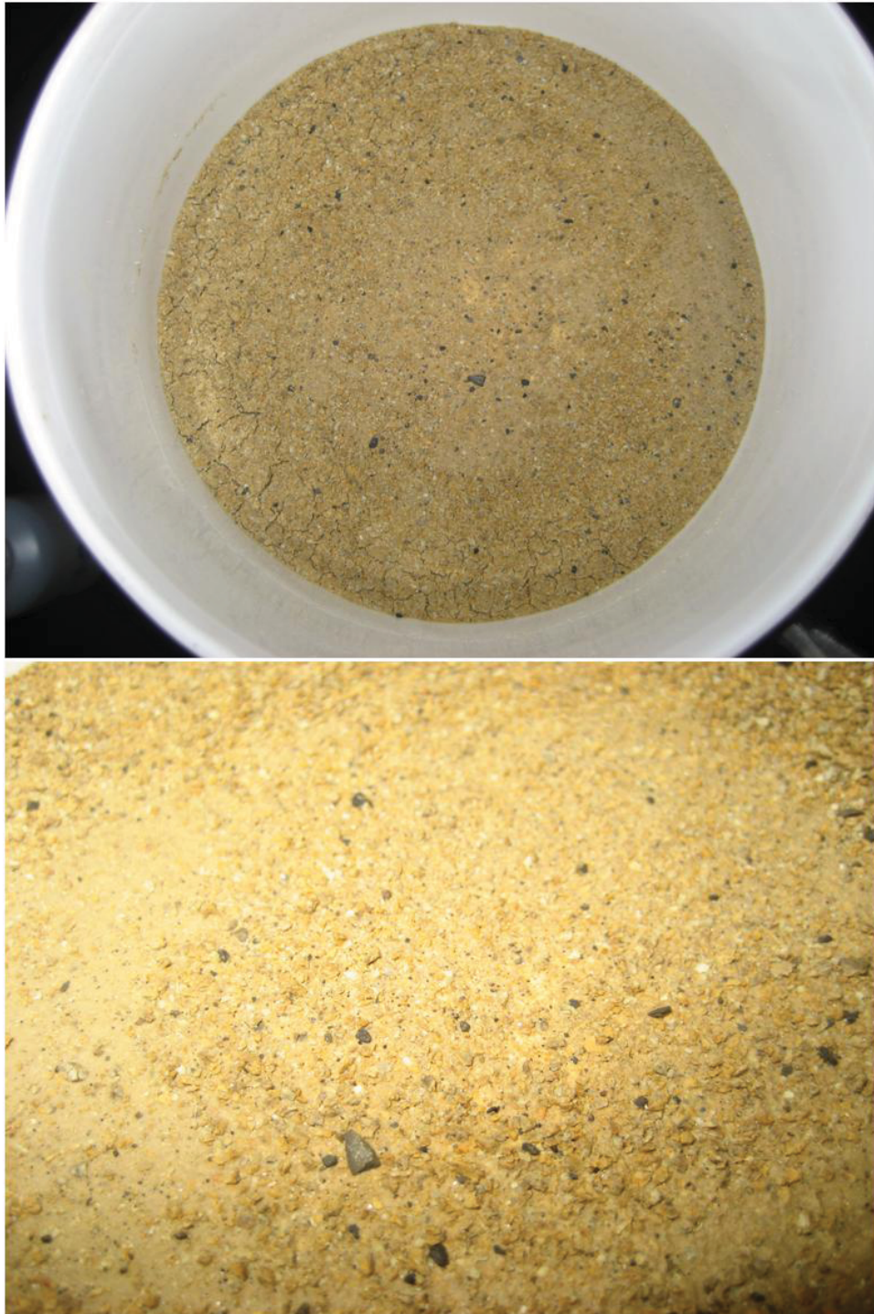
Fig. N. 6. Bentonite from Site E TP1 during bound cation testing. Dark material is visible through the specimen.
