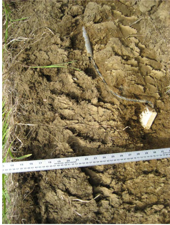
Fig. A.47. Conventional cover profile (soil above GM).
