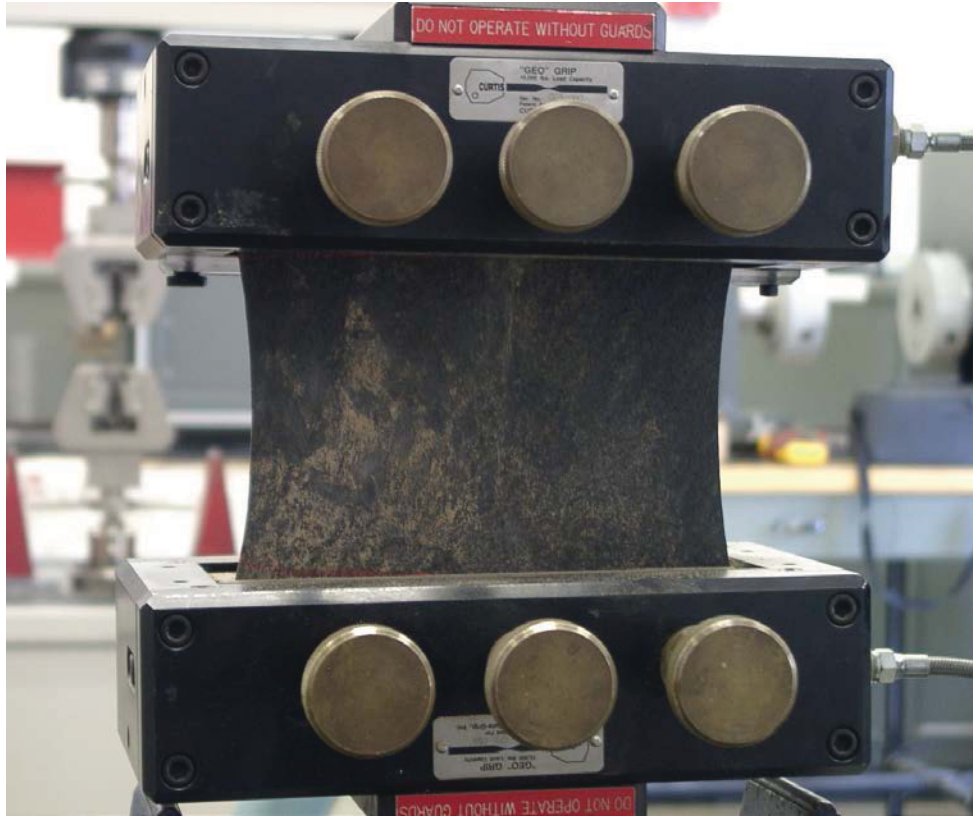
Fig. Q2. Close up of a wide-strip tensile testing of GM.
