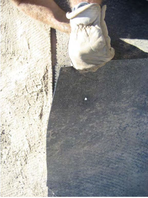
Fig A.6. Constructed defect in GM.
