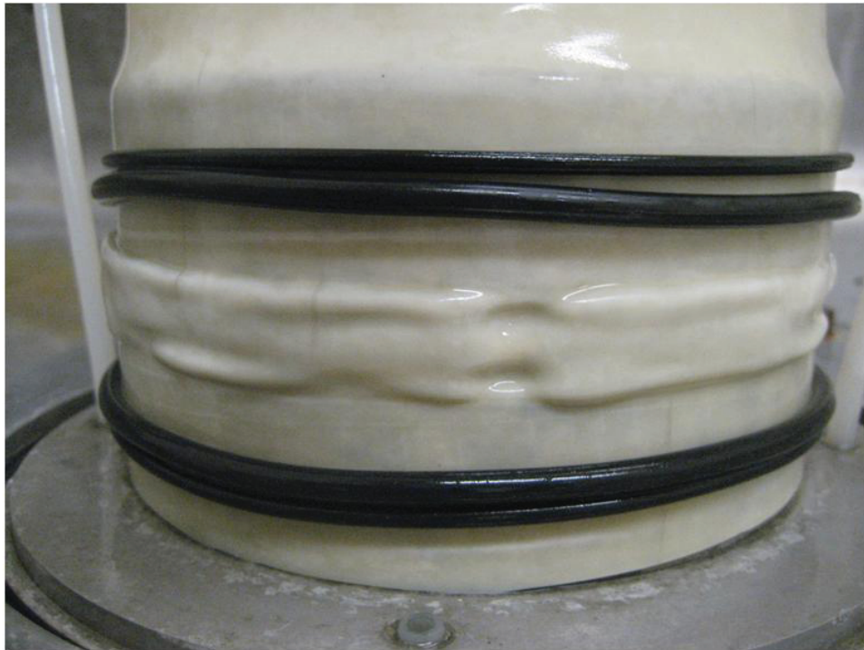
Fig. O. 4. Latex membrane over internal bentonite paste gap after application of effective stress, permeation, and disassembly.
