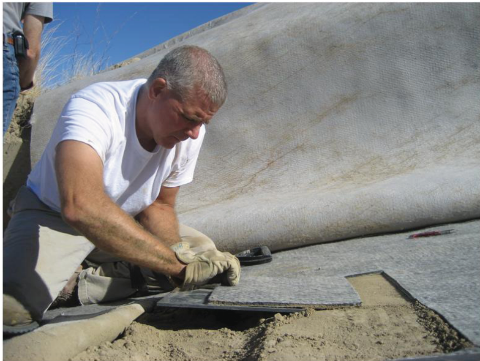
Fig. M. 6. Sliding rigid PVC plate under GCL sample during exhumation.
