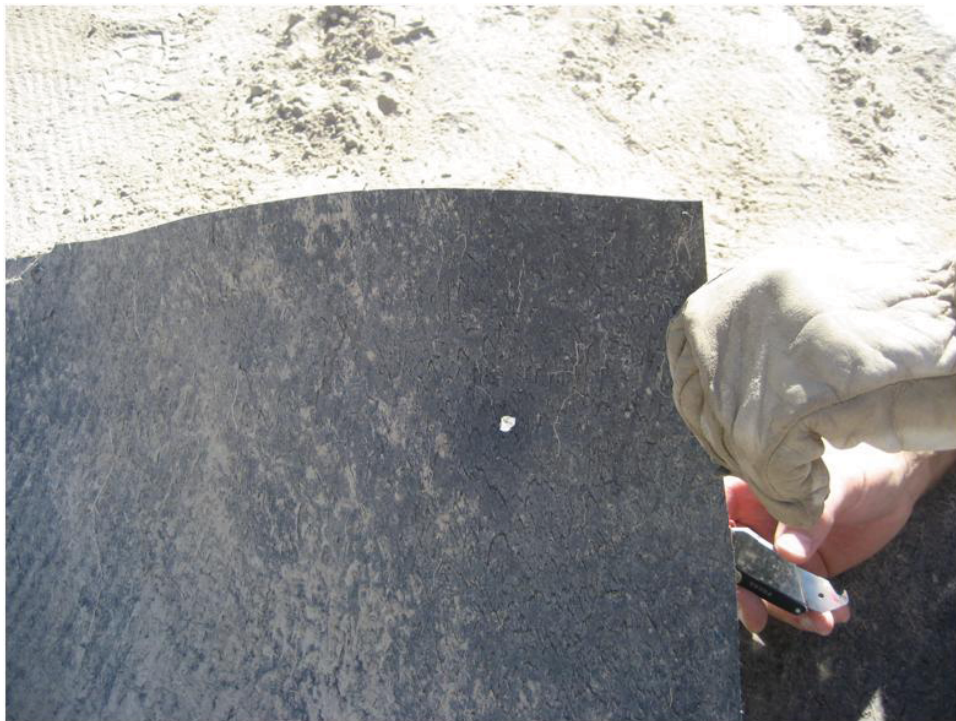
Fig. M. 4. Installed whole in lysimeters GM exposed during exhumation.
