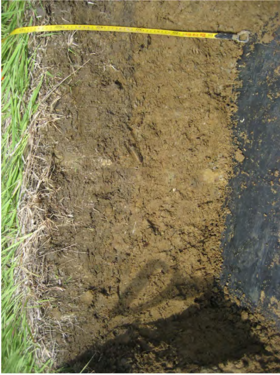
Fig. A.47. Conventional cover profile (soil above GM).
