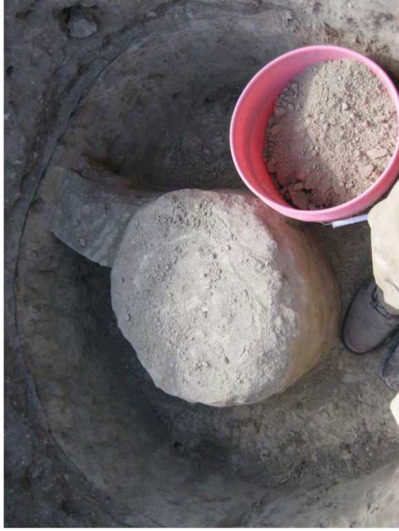
Fig. A.29. Installation of SDRI seating trenches.
