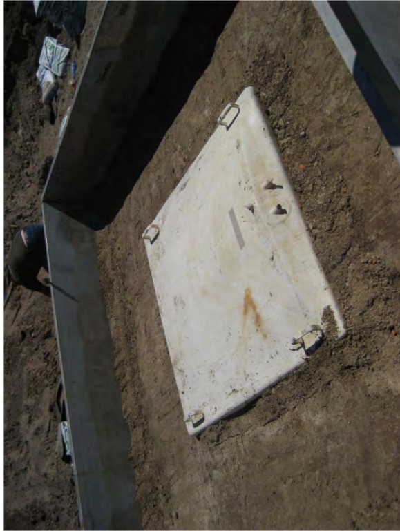
Fig. A.28. Installing SDRI under GM into CCL.
