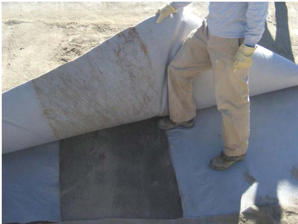
Fig. M. 2. Rooting observed at GDL-GM interface but not at GDL overlaps.
