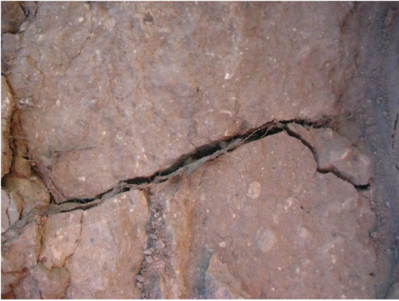
Fig. A.36. Failure along vertical root planes during trenching.
