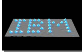
Writing with atoms. D.M. Eigler, E.K. Schweizer. Positioning single atoms with a scanning tunneling microscope. Nature 344, 10 524-526 (1990).
