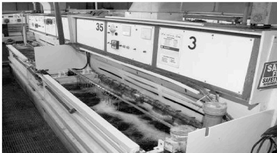
Cu, In, Ga, Se sequentially electroplated onto solar panels
