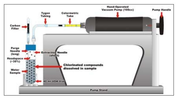
The colorimetric detector tubes are constructed of glass and printed with calibration scales to facilitate measurement of the linear extent of the color change reaction that occurs within the tube. To conduct the method, a standard 40-milliliter (ml) volatile organic analysis (VOA) vial is filled with the groundwater sample to approximately 70% capacity (leaving a 30% headspace) and tightly capped. The sample vial is then heated to approximately 40° Celsius in a water bath.
