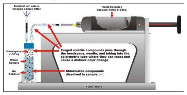
To analyze soil, sediment, or sludge samples using the Color-Tec method, approximately 25 to 35 grams of soil is placed into a VOA vial, followed by deionized water filled to approximately 70% capacity (leaving a 30% headspace) and tightly capped. The sample vial is then heated to approximately 40° Celsius in a warm water bath. The analysis procedure is the same as with water samples.
