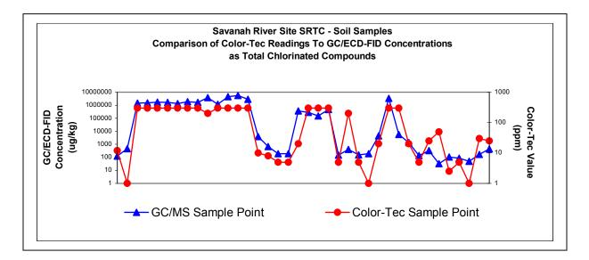
The colorimetric tubes detect the sum total of all chlorinated compounds present in the sample. This interference from the other chlorinated compounds makes the identification of a specific chlorinated compound within the sample impossible. This is Color-Tec results are compared to the sum of all chlorinated compounds detected by GC/MS in the sample.
