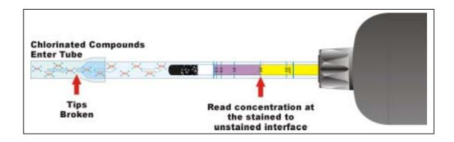
Gastec<sup>®</sup> provides tubes for identifying several specific chlorinated compounds including PCE, TCE, vinyl chloride, carbon tetrachloride, and methylene chloride. Because each of these tubes uses the same basic detection principle shown above, they will each react positively to all of the other chlorinated compounds.
