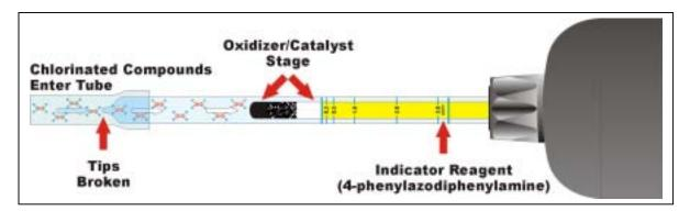
The colorimetric tubes and hand pumps used for E & E's Color-Tec method are manufactured by Gastec<sup>®</sup>, Inc. Each colorimetric tube contains a catalyst that decomposes chlorinated alkenes and alkanes, releasing hydrogen chloride, which discolors the reagent (4-phenylazodiphenylamine) in the tube. The reaction formula provided by Gastec<sup>®</sup>, Inc. for the PCE tube is as follows:
