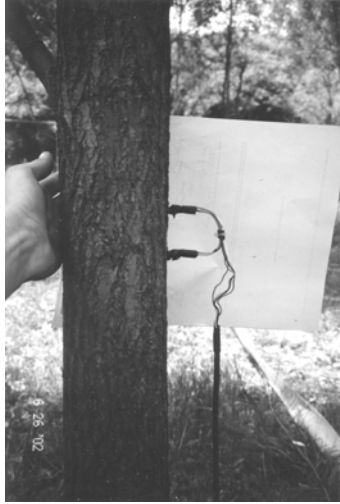
TDPs used to measure water use on a tree at the SRSNE site (Case Study 1)
