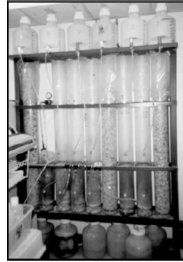
2-yr kinetic tests, Montana Tunnels, MT; Photo by A. Maest
