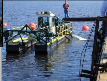
Manistique – outriggers used to control positioning of auger dredge
