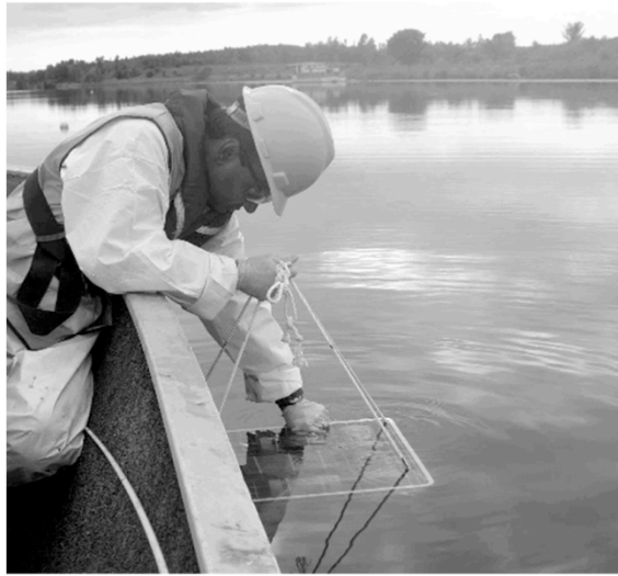
In-river deployment of field exposure cages with L. variegatus for baseline study (method adapted from Burton et al. 2005)
