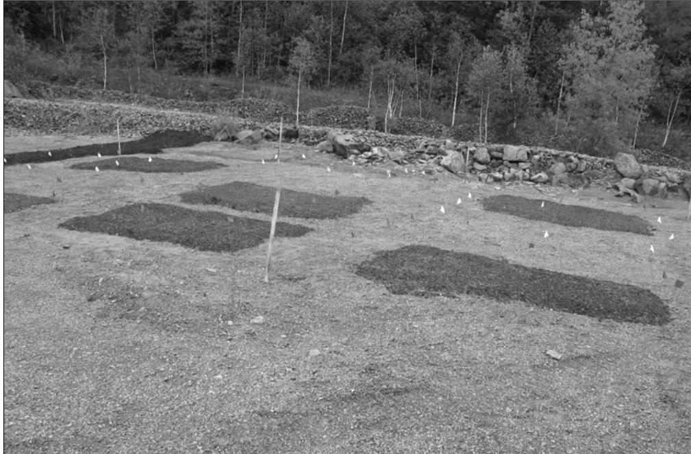
Test plots with two compost mixtures vs. Control (three replications in RCB) VAG site August 23, 2010.
