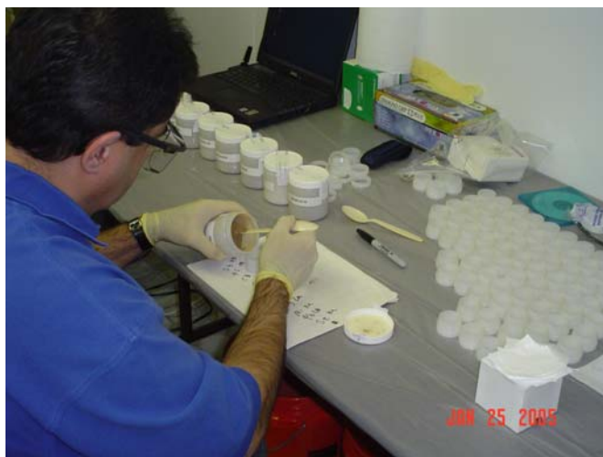
Figure 6-2. Rigaku technician filling a sample cup for analysis.
