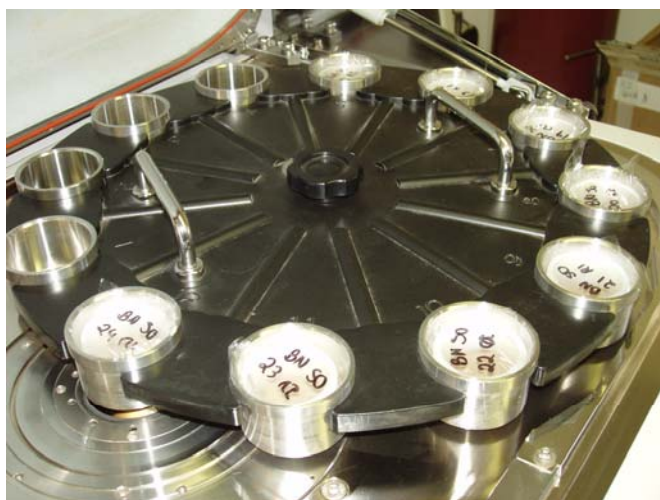
Figure 6.3. Samples placed into the 12-position sample changer awaiting analysis.
