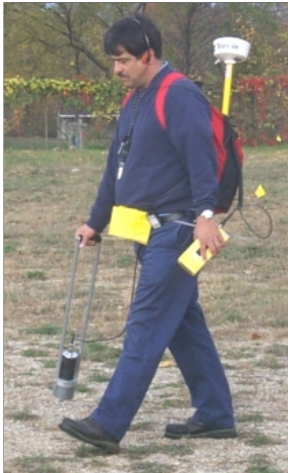
Figure 4. Gamma walkover equipment with GPS.
