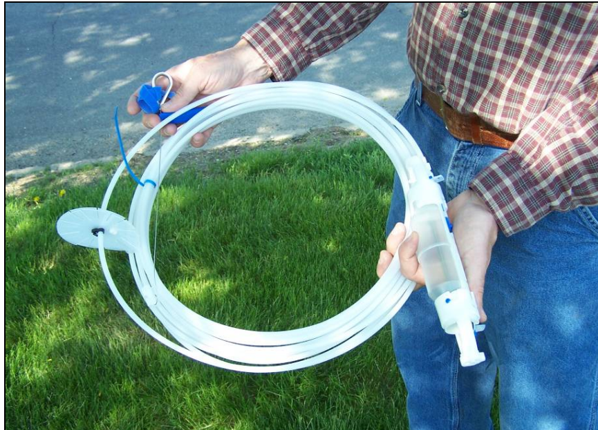
Figure 8. Photo of Snap Sampler, trigger line, and baffle.
