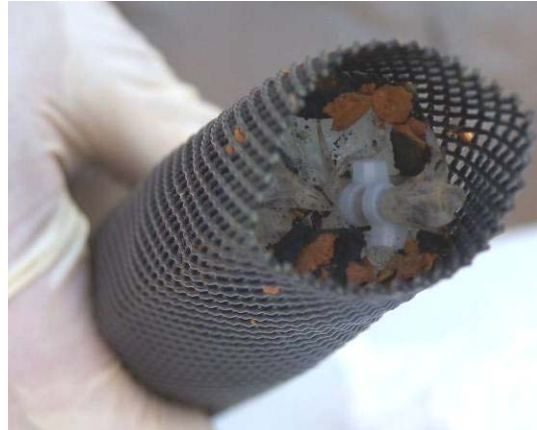
Figure 5-37. Top of RGC sampler showing deposits of large black and orange particles.
