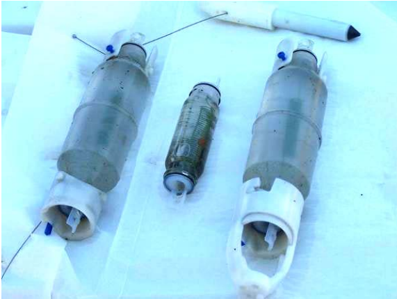
Figure 5-36. Photo of Snap Sampler samples showing black particles and piece of rusted casing (inside VOA vial).
