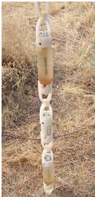
Figure 5-38. Snap Samplers containing an orange precipitate.
