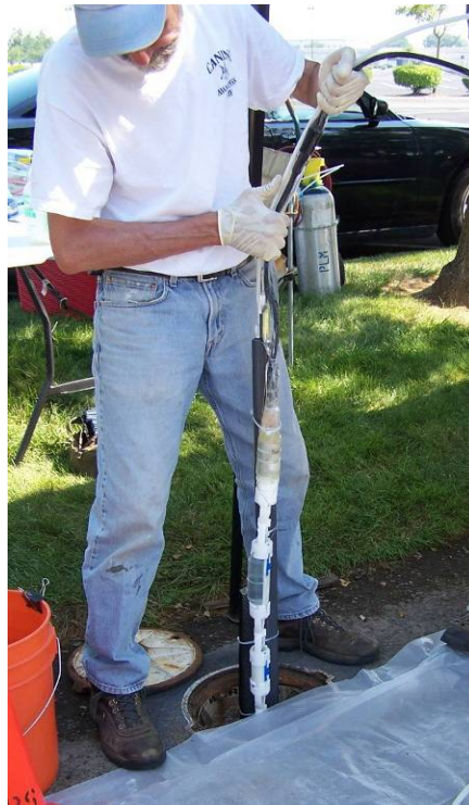
Figure 5-5. Tethered sampling equipment being placed in well.
