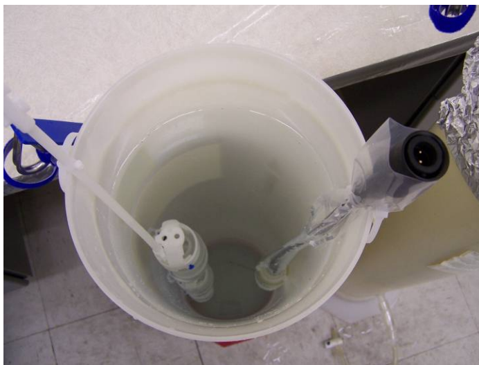
Figure B-1. Pipette cleaner with Snap Sampler string and shielded actuator line.
