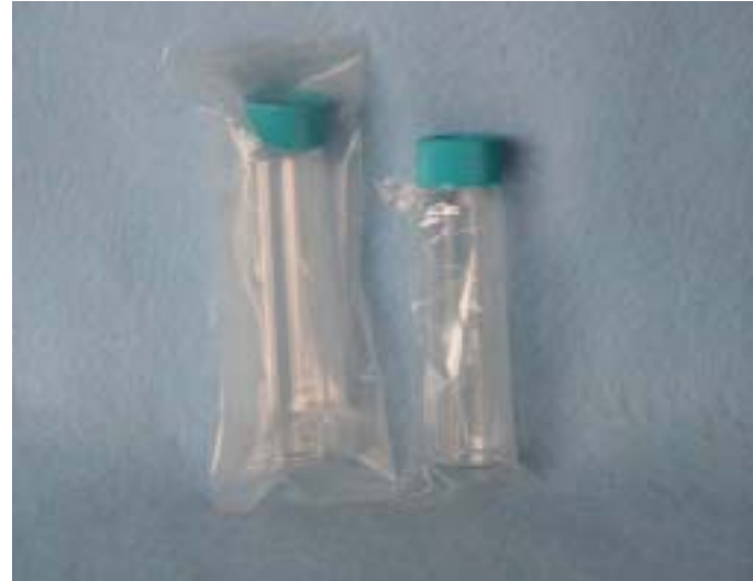
Figure 6-2. Commercially available samplers with VOA vial sealed inside two layers of LDPE membrane (Photo from EON, 2005)
