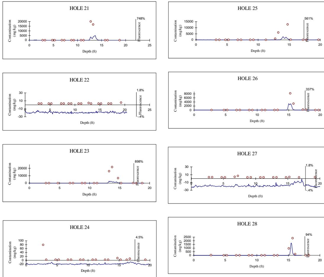
**Figure 6-2. Adjusted downhole results for Port Hueneme.** This figure provides a summary of all downhole results after adjustment for depth measurement inaccuracies due to sloughing that appears to have affected the measurements in the saturated zone at boring locations 23 and 28. Note that the vertical axes for the holes beyond the plume boundary, holes 22, 24, and 27, have a smaller scale than holes 21, 23, 25, 26, and 28, where contamination was detected.
