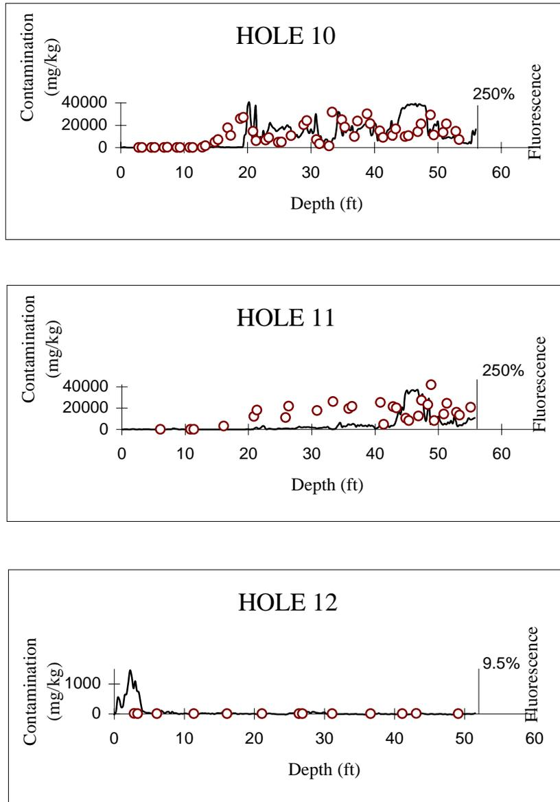
Figure 6-4. Downhole results for SNL Tank Farm.
