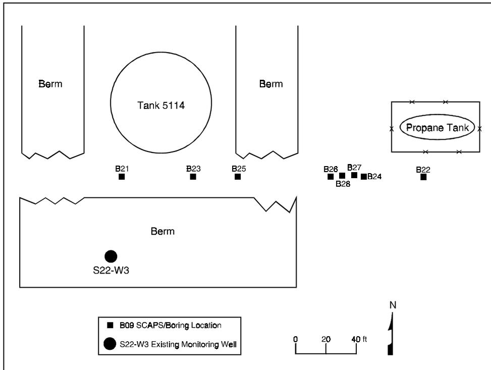
**Figure 5-2. Demonstration site and sampling locations, Port Hueneme.** B21-B28 are the locations of the HSA borings associated with the CPT pushes. For example, B21 is the boring associated with PHDR21, the initial ROST push.
