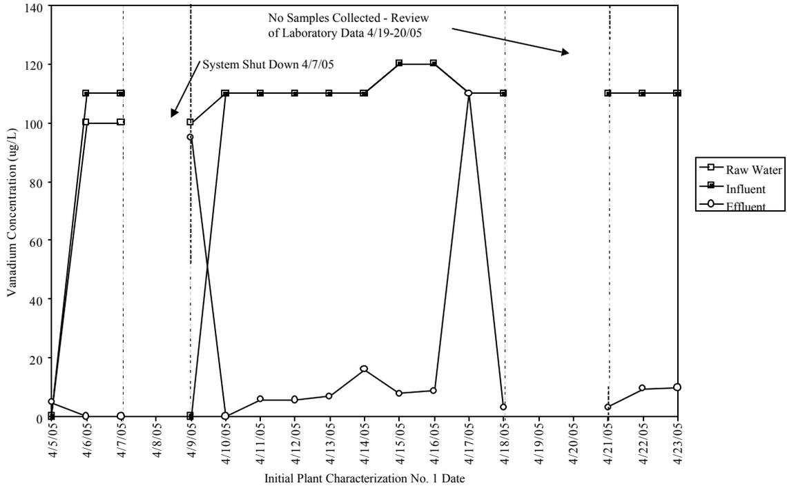
**Figure 4-2: Temporal plot of Initial Plant Characterization No. 1 raw, influent, and effluent water vanadium.**
