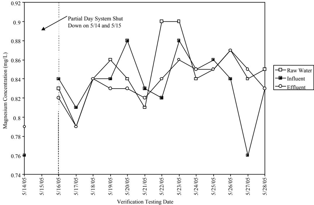
**Figure 4-25: Temporal plot of verification testing raw, influent, and effluent water magnesium.**
