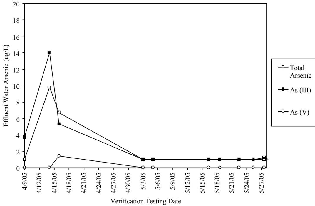
**Figure 4-28: Speciated arsenic effluent water results for Initial Plant Characterization through verification testing.**
