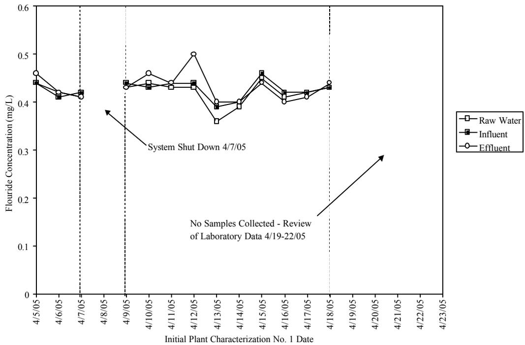
**Figure 4-6: Temporal plot of Initial Plant Characterization No. 1 of daily raw, influent, and effluent water fluoride.**
