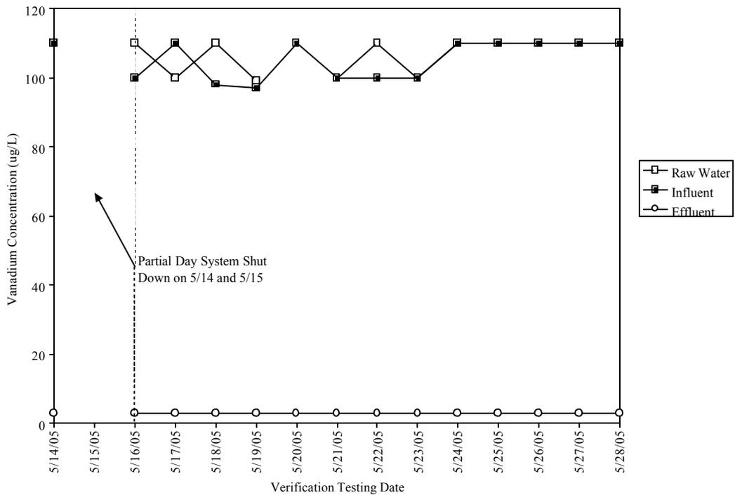
**Figure 4-14: Temporal plot of verification testing 24-hour composite raw, influent, and effluent water vanadium.**
