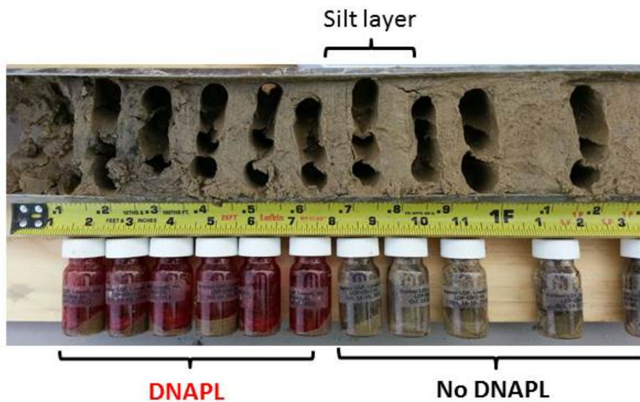
This photograph is a close-up of a core after the sampling process has been completed. Note the four subcore holes at each interval. The photograph also depicts positive shake test results for the DNAPL.
