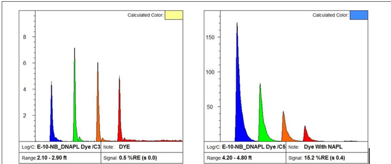
**Figure 3. Indicator dye waveform in carrier water (left) and solvated in chlorinated DNAPL (right).**
