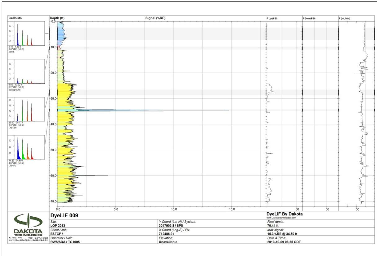
Figure 4. Example DyeLIF log depicting color coding of fluorescence response.
