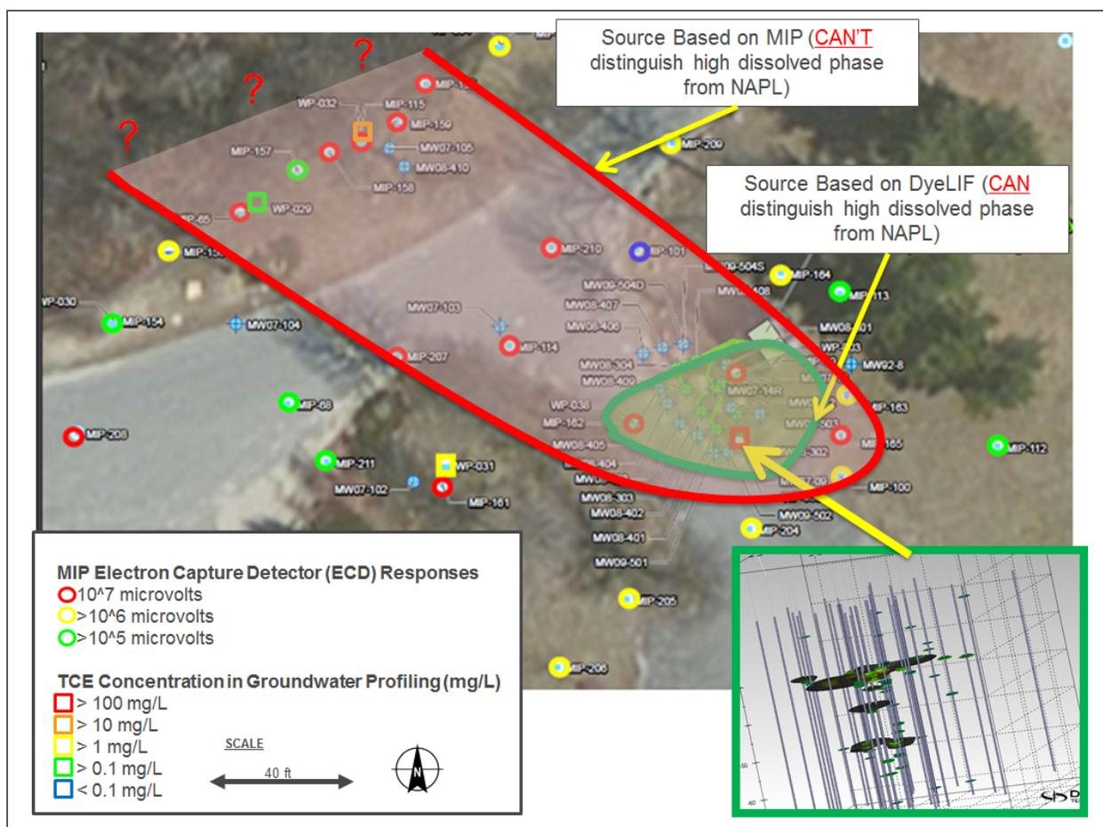
**Figure 14. Comparisons of DNAPL source zone delineation using DyeLIF and MIP with depth-discrete groundwater sampling.**
