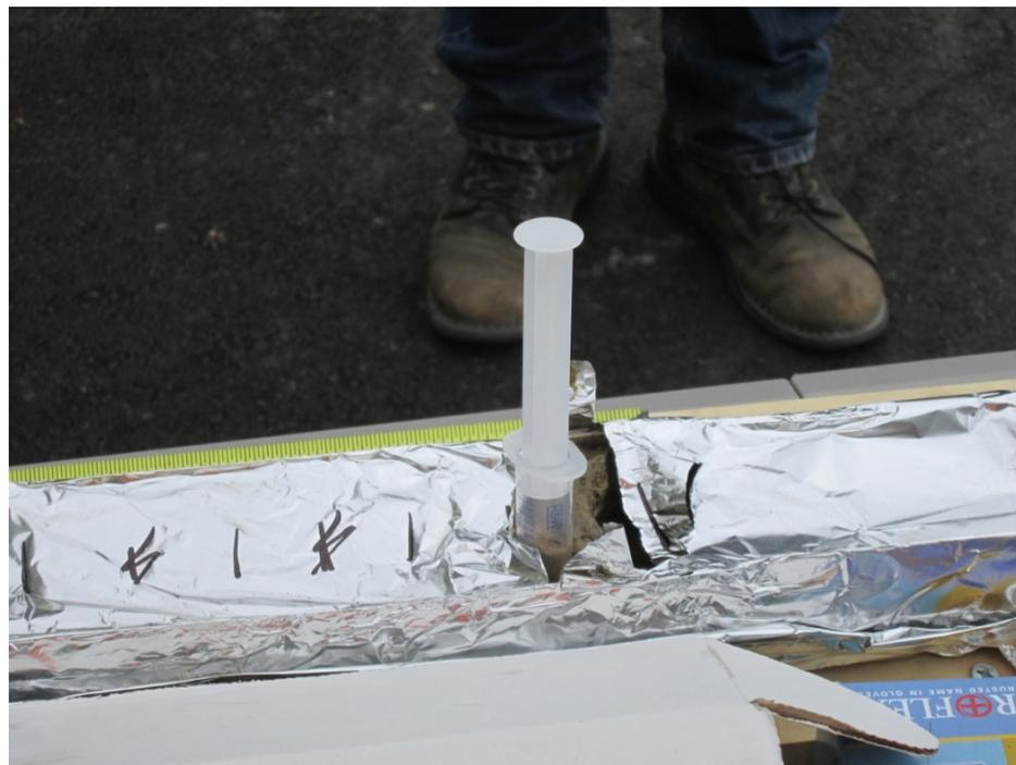
**Step 4.** A marker was used to demarcate the sampling intervals on the aluminum foil. When it was time to sample a particular interval, the foil was pulled back. Four subsamples were collected at each depth interval for laboratory analysis of VOCs, Oil-Red-O dye shake tests, DyeLIF screening, and moisture content.
