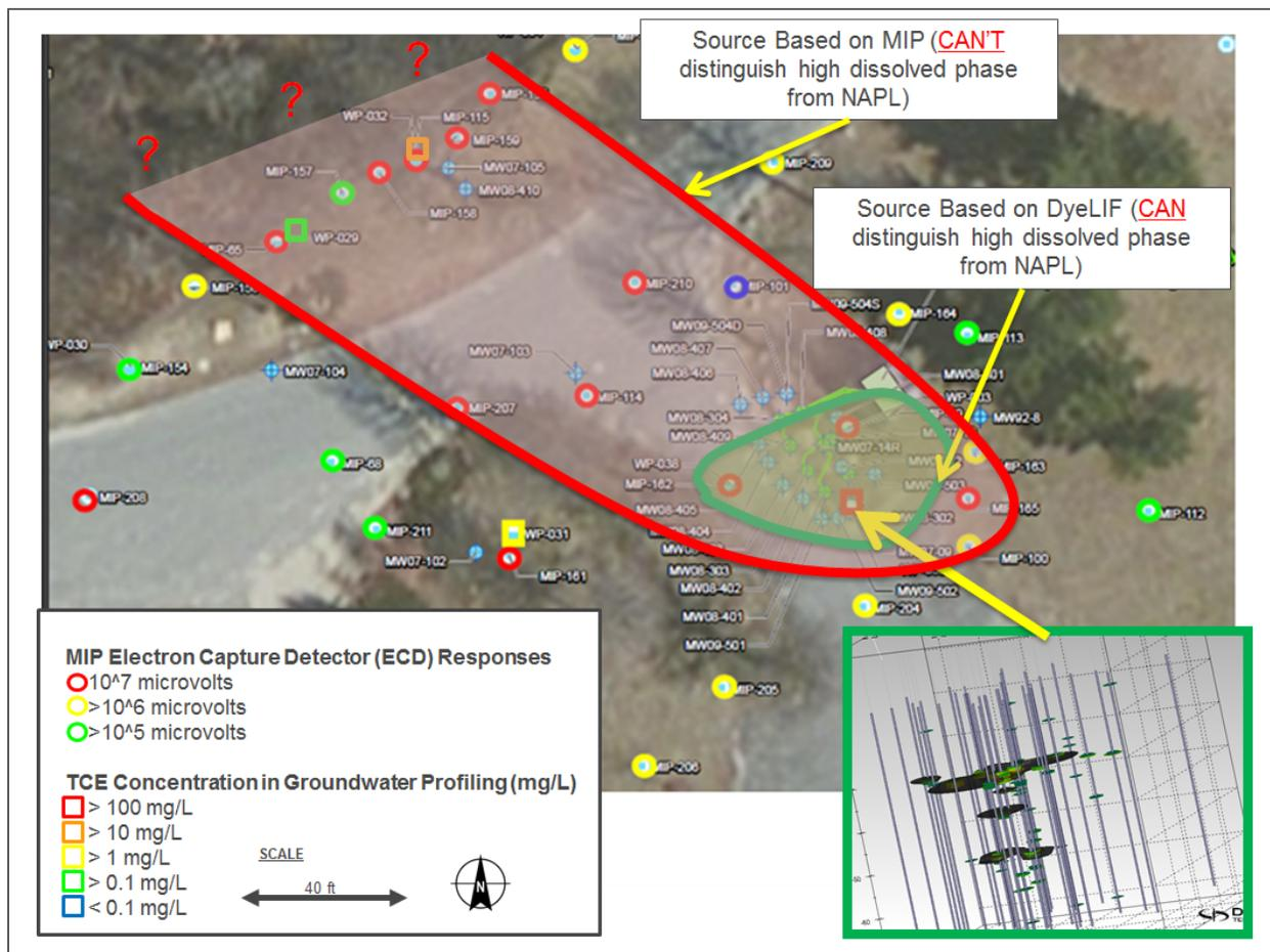
**Figure ES-2. Groundwater and MIP sampling results in the demonstration area. These results illustrate the challenge of delineating a DNAPL source zone with high-resolution characterization tools that cannot distinguish between high-concentration dissolved-phase contamination and DNAPL. DyeLIF detects only separate-phase NAPLs, which is advantageous for source zone assessments.**
