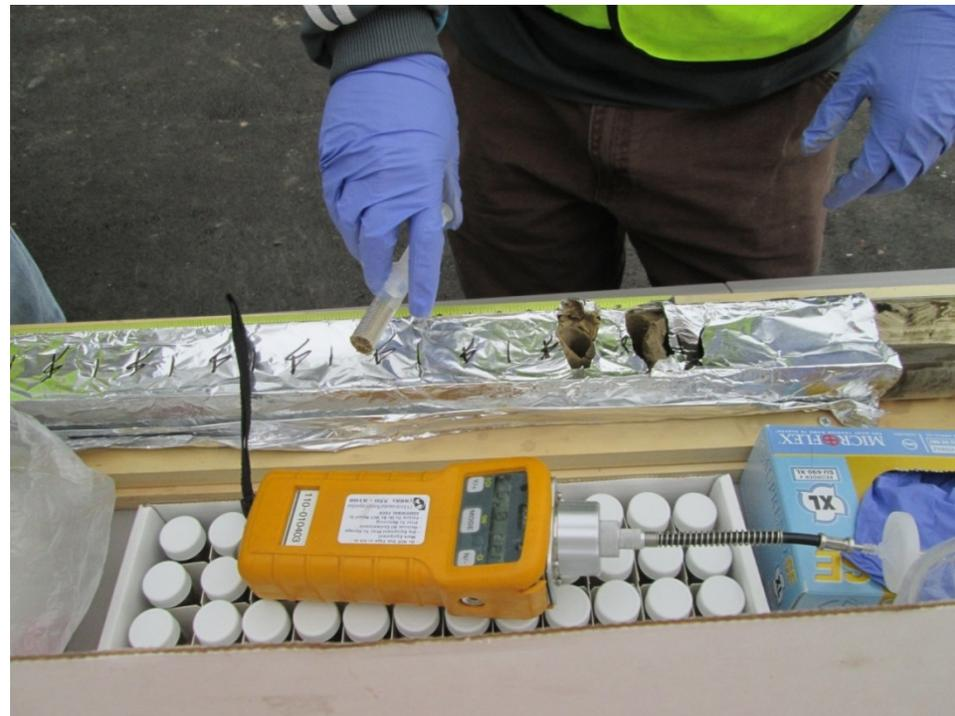
**Step 6.** After sampling is completed at one depth interval, foil from the next interval is peeled back and the process is repeated.
