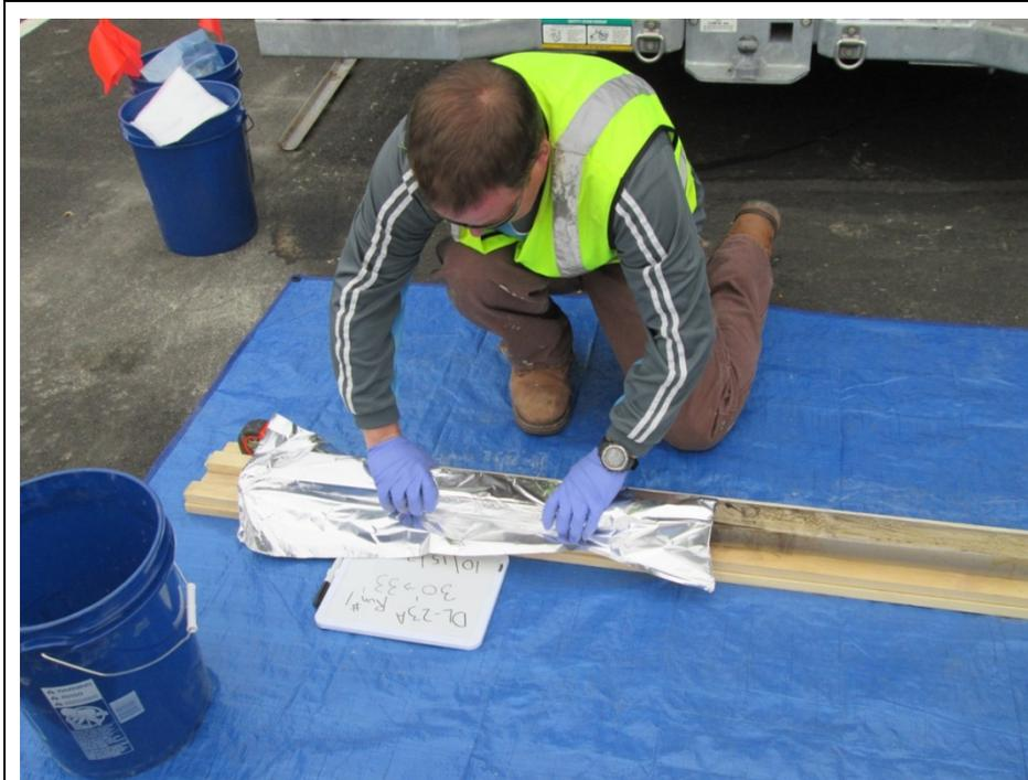
**Step 3.** After the core was photographed it was quickly covered with foil in order to minimize volatile losses.
