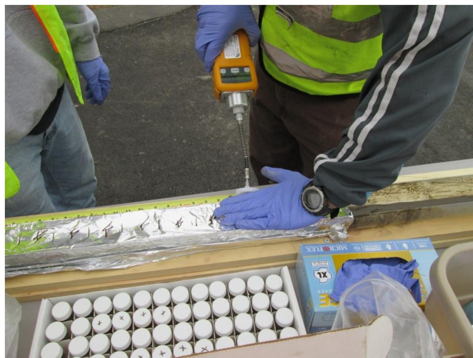
**Step 5.** After the subsamples are collected, a PID measurement is collected by placing the PID tip in one of the holes made by the subsampling and covering the whole with a plastic glove.
