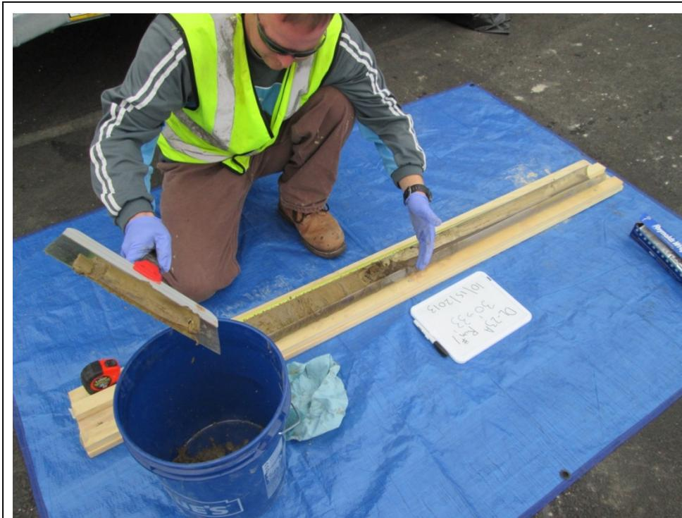
**Step 1.** After the ore is split open, a large drywall tapping knife was used to scrape off the top layer of soil.
