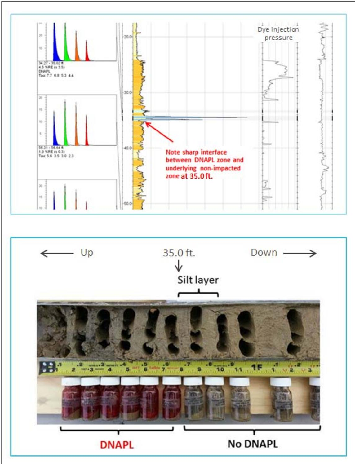
Figure 8. Example DyeLIF and soil boring logs showing no evidence of vertical DNAPL drag-down.
