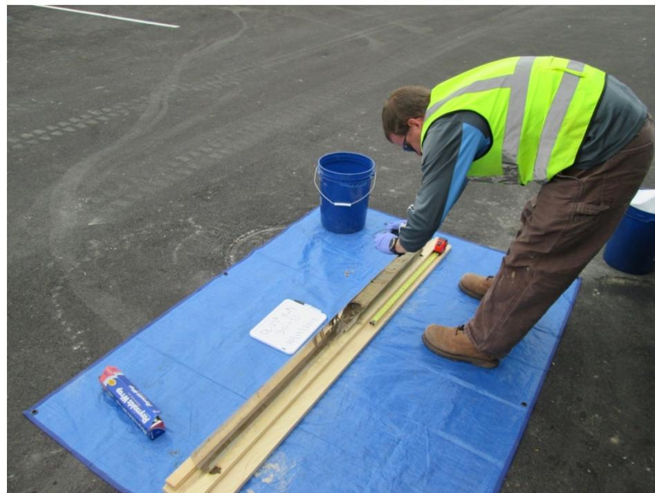
**Step 2.** A photograph of the core was taken. The dry-erase board shown indicates the location ID and core run
