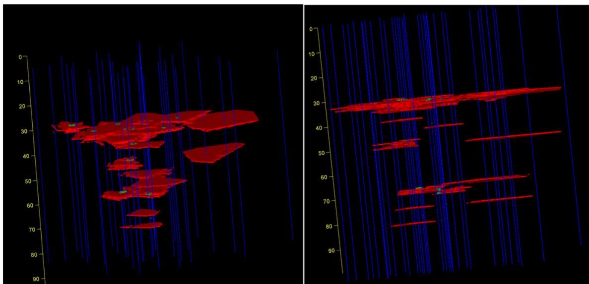
**Figure ES-1. Three-dimensional graphical depictions of the DNAPL source zone at demonstration site. This site assessment, performed in only four days using DyeLIF, provides the most detailed delineation of subsurface DNAPL ever made at a non-research field site.**
