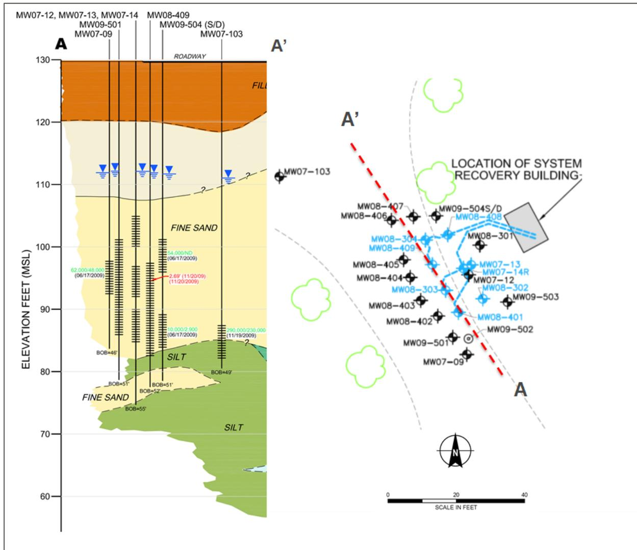
**Figure 10.** Cross-section through demonstration area (from GZA, 2011). Wells with current and/or historical DNAPL occurrence are shown as blue.
