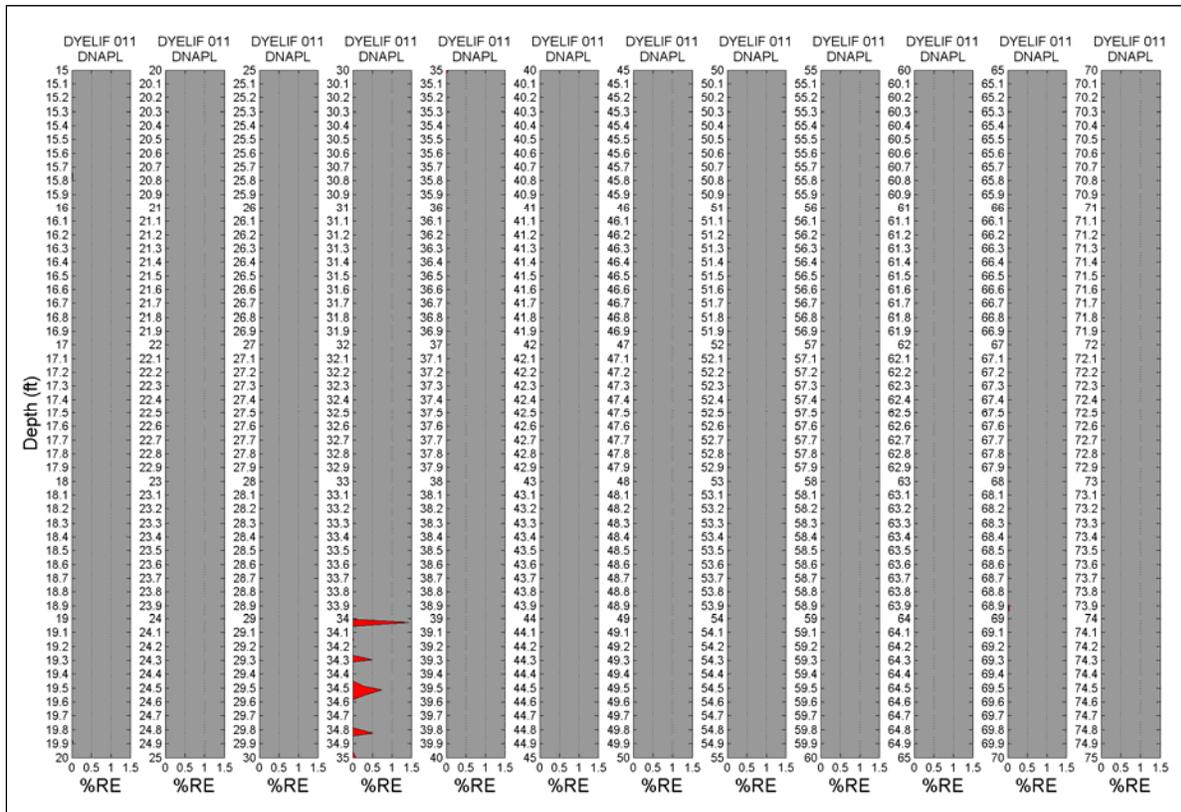
Figure 7. Multi-panel DNAPL graphic for location DL-11. Each panel corresponds to 5-feet of probing depth. This new data deliverable aids in identifying small (centimeter-scale) DNAPL zones.
