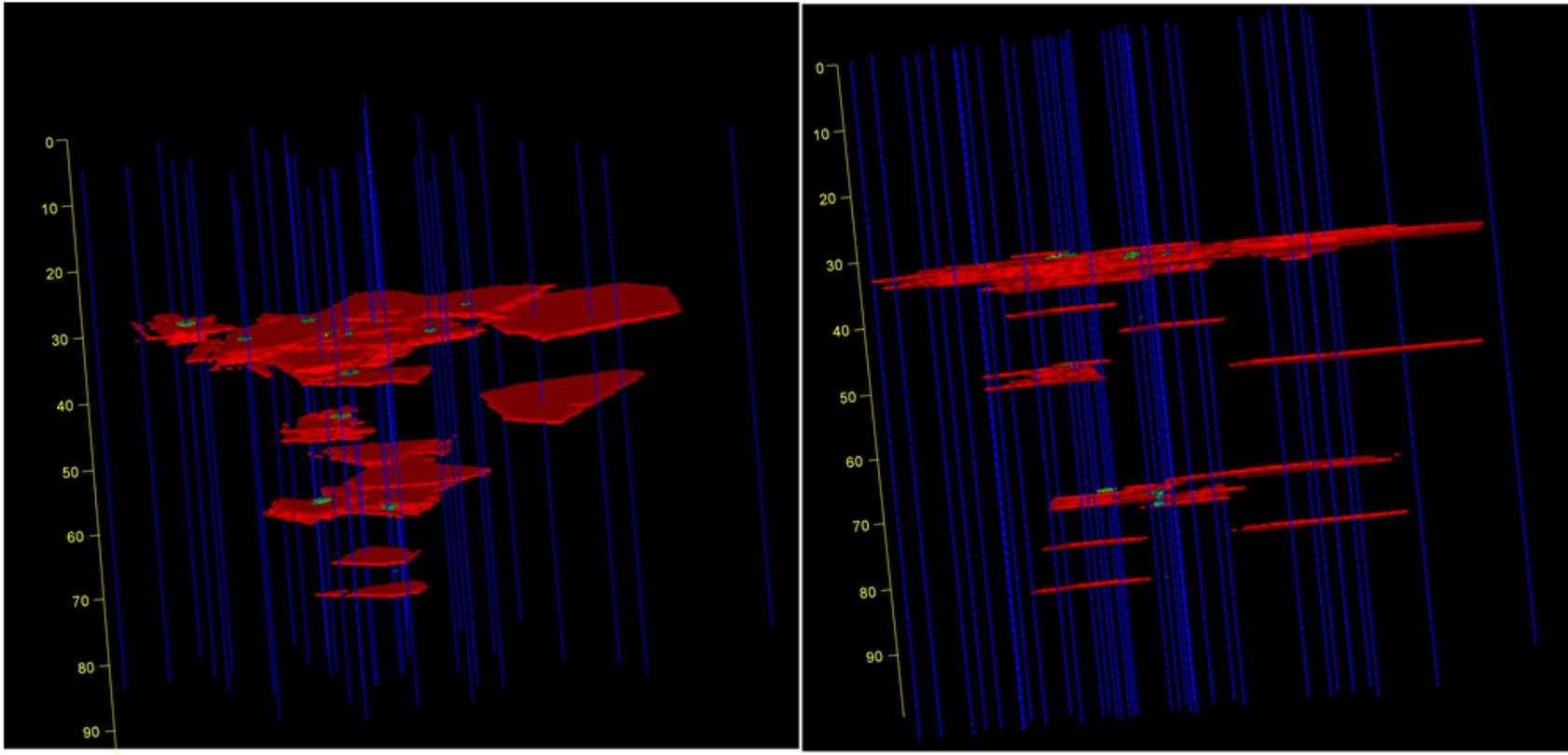
Figure 13. Three-dimensional graphical depiction of DNAPL source zone at demonstration site.
