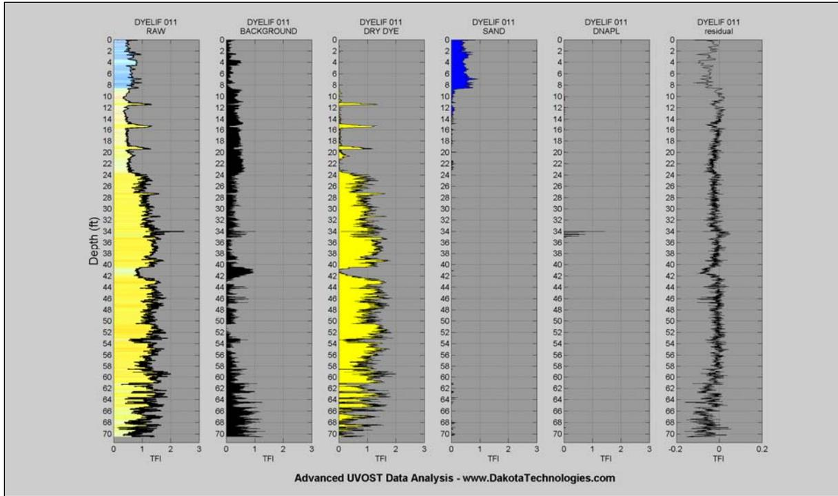
Figure 6. Strip logs showing the raw fluorescence plot along with the contributions of other waveforms in the Basis Set (instrument background, sand, non-solvated dye, DNAPL) for location DL-11.
