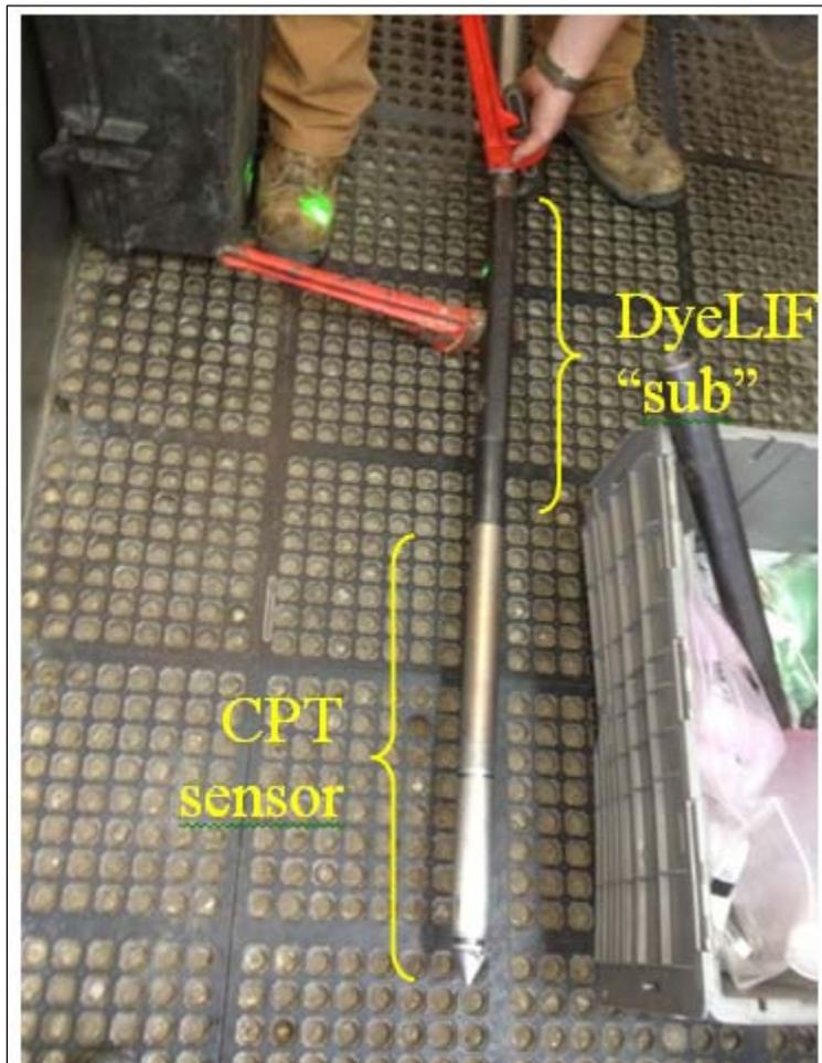
**Figure 2. CPT delivered version of DyeLIF. Refer to Figure 1 schematic for additional details on DyeLIF sub.**
