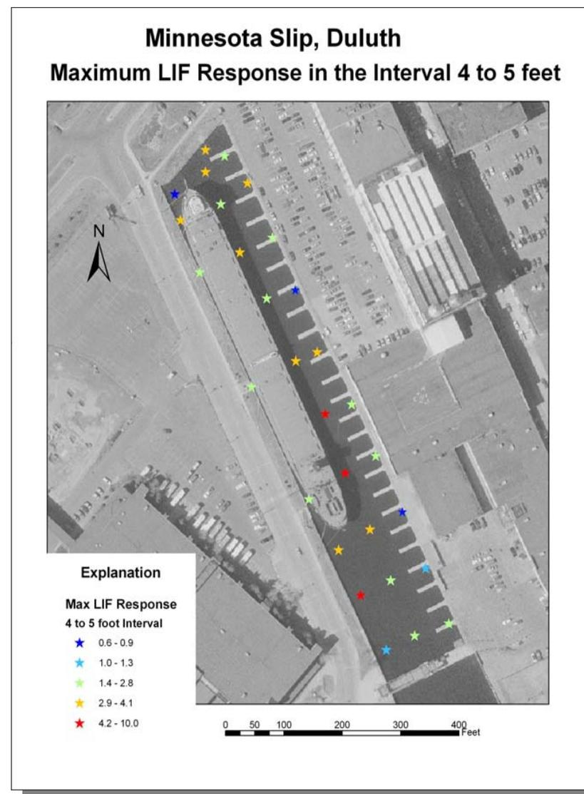
Figure 15: Maximum LIF Response Detected in Fourth and Fifth foot of Sediment.
