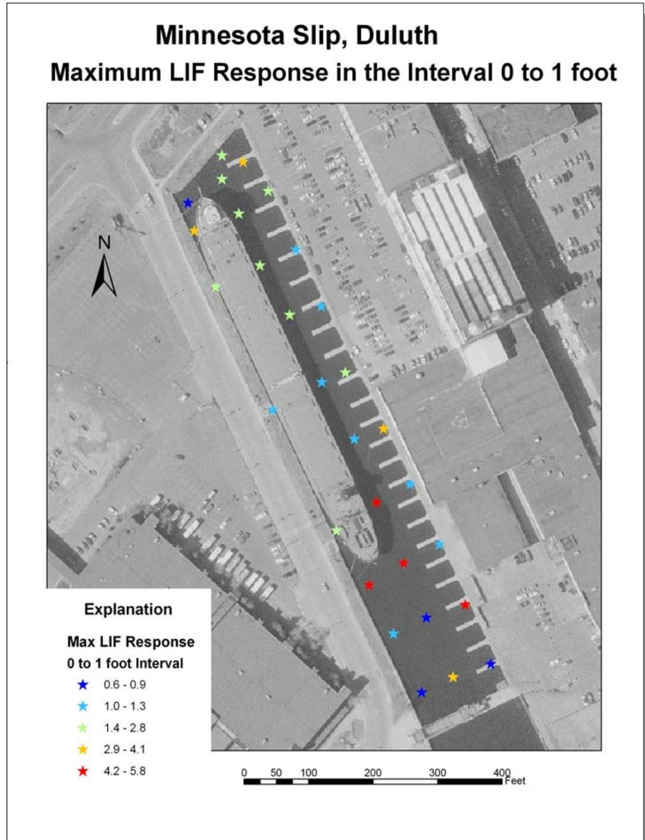
Figure 13: Maximum LIF Response Detected in Top Foot of Sediment
