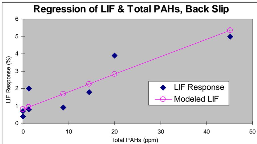
Figure 23: Regression Analysis of LIF Response and Total PAH Concentrations for Samples from the Back Slip.
