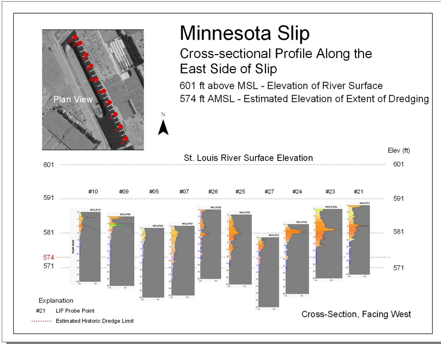
Figure 12: Cross-section Along the Eastern Wall of the Slip, Featuring LIF Response Records.
