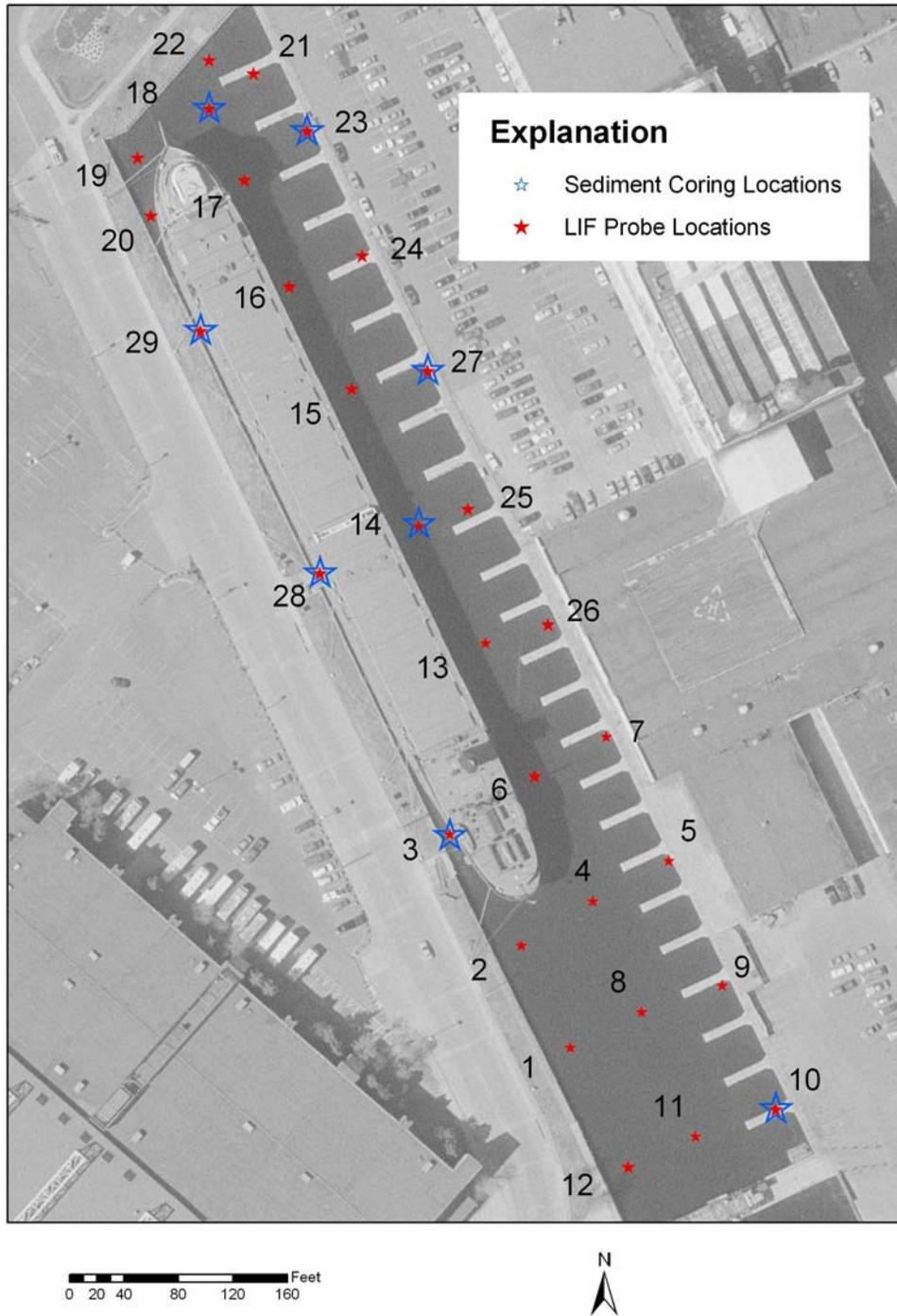
Figure 7: Location of LIF Probes and Sediment Cores.
