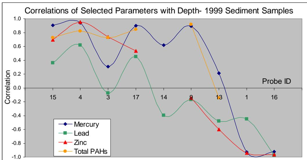
Figure 16: Correlation Between Increasing Sediment Depth and Parameter Concentration for selected cores.
