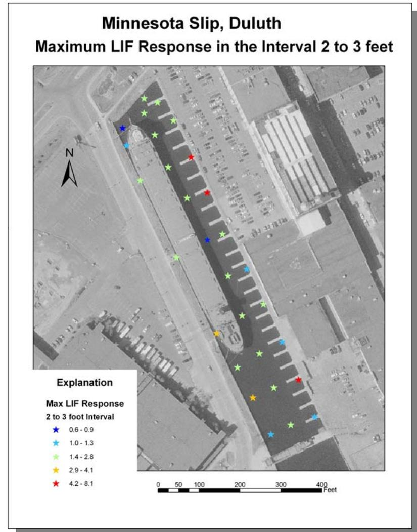
Figure 14: Maximum LIF Response Detected in Second and Third foot of Sediment.
