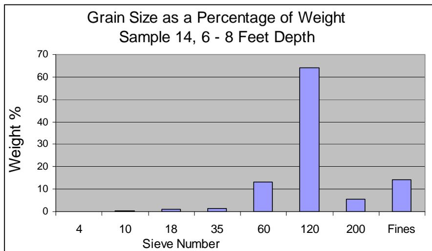
Figure 18: Grain Size Weight Distribution for Sample 14, 6 – 8 feet.
