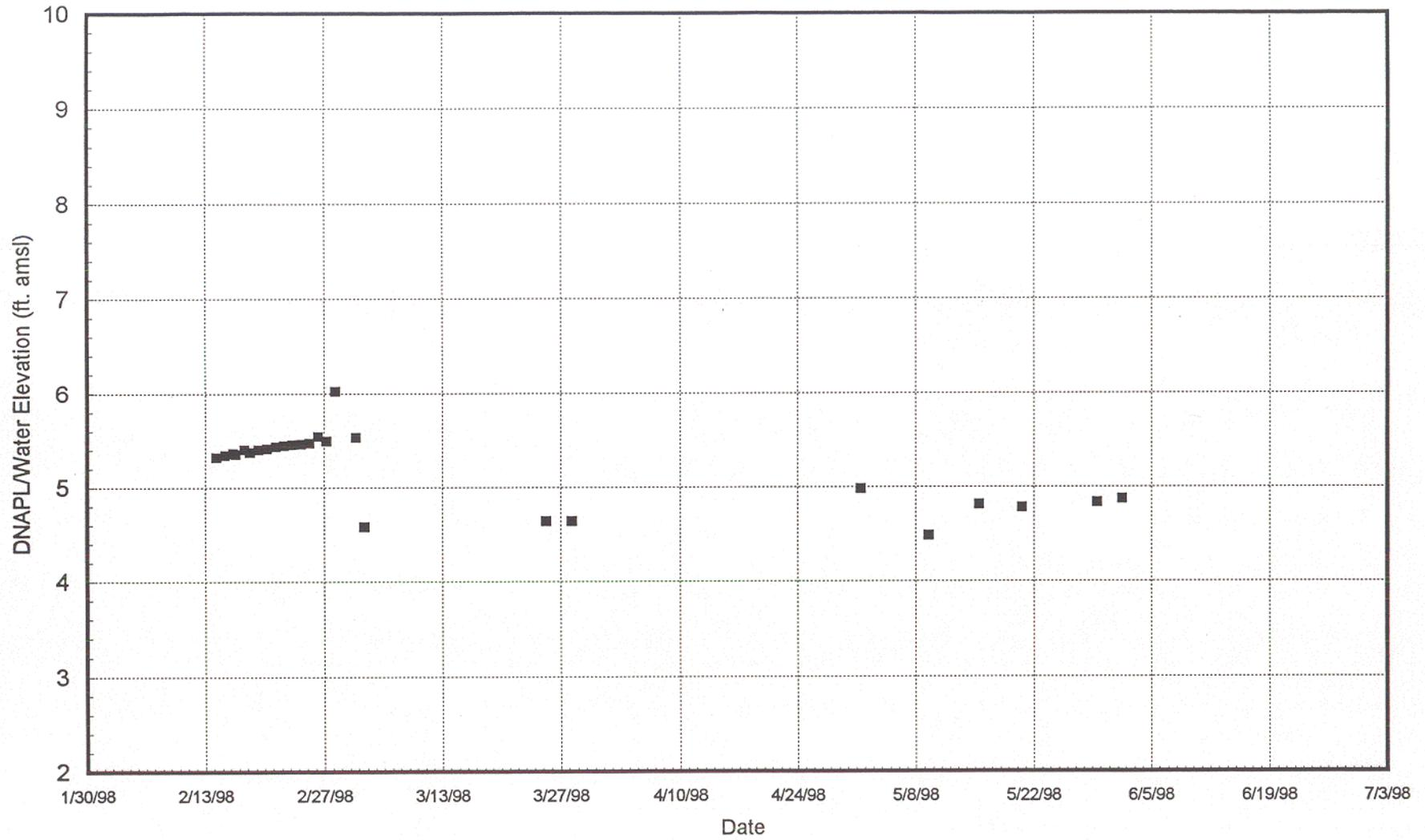
DNAPL/Water interface Elevation During Field Operations in Well EX02
