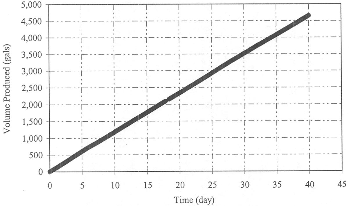
Figure M-30 Upper injection well IN03up cumulative volume injected as a function of time
