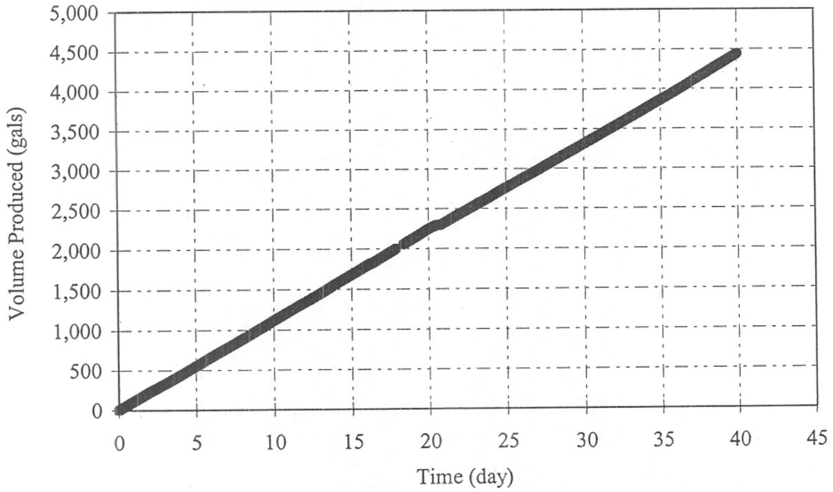
Figure M-26 Upper injection well IN01up cumulative volume injected as a function of time
