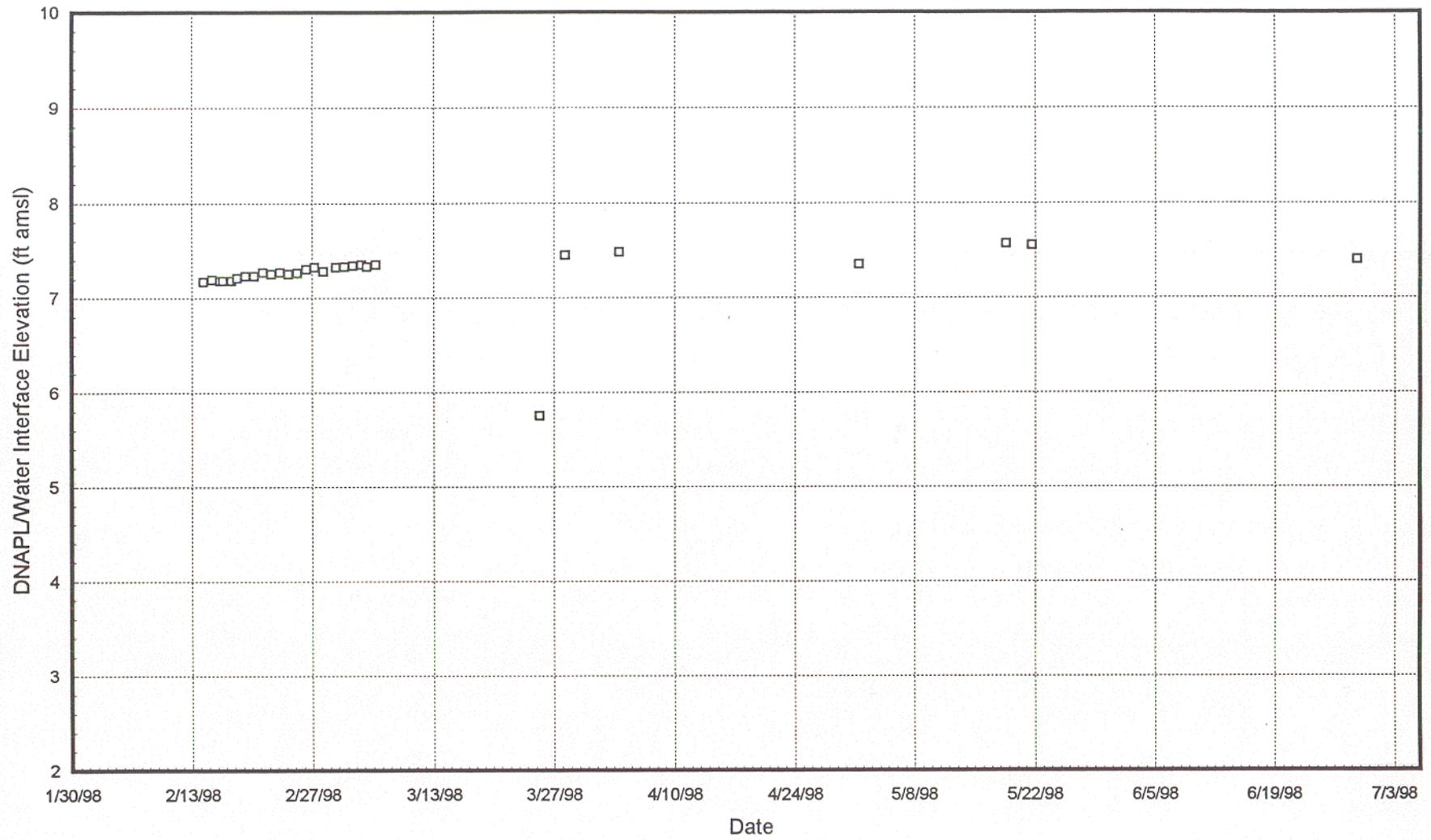
DNAPL/Water Interface Elevation During Field Operations in Well RW02
