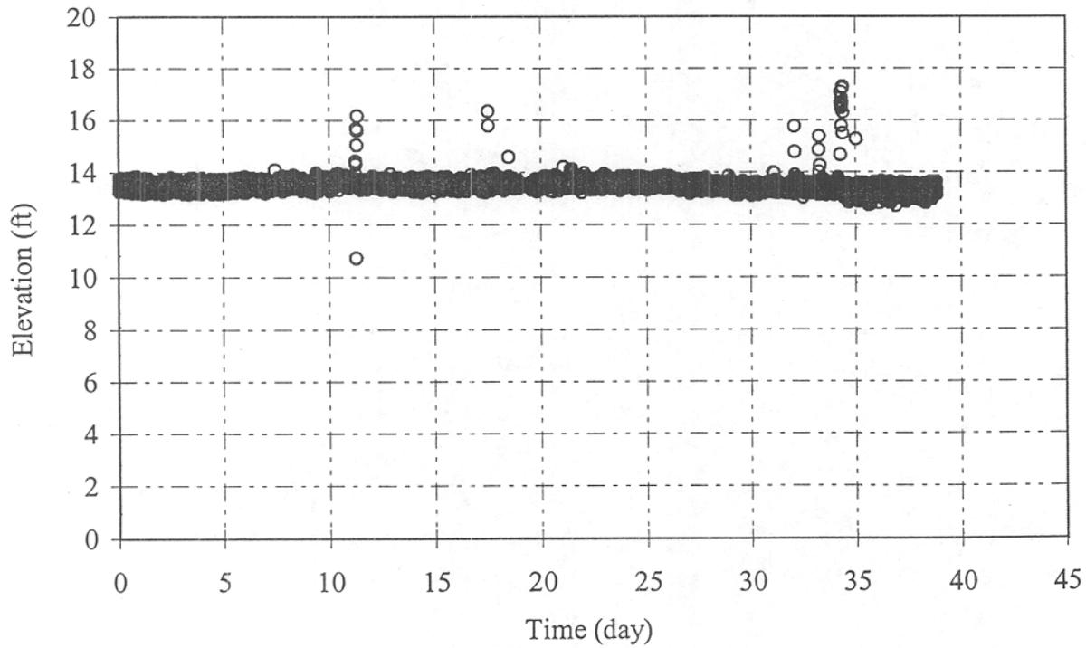
Figure M-37 Water level elevation at extraction well EX02 as a function of time
