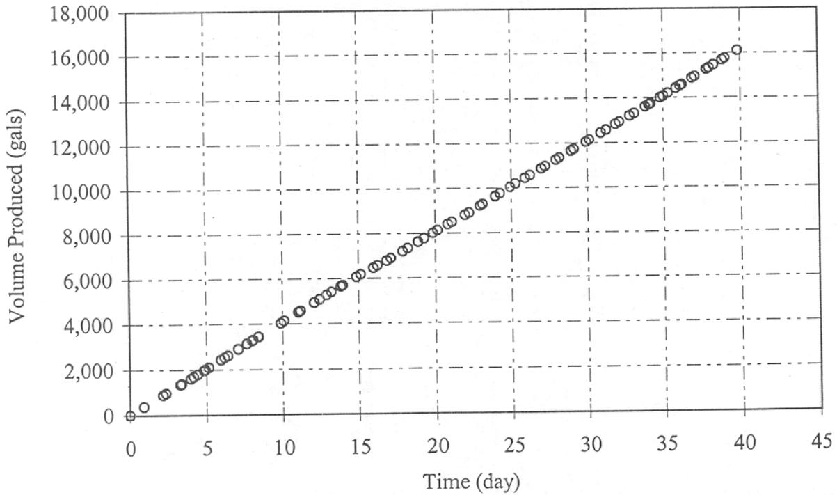
Figure M-6 Extraction well EX03 cumulative volume produced as a function of time
