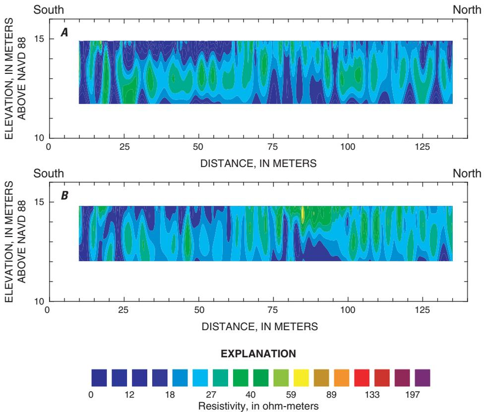
Figure 7. Sections showing inversion results of capacitively coupled resistivity data for (A) line 1 and (B) line 7.
