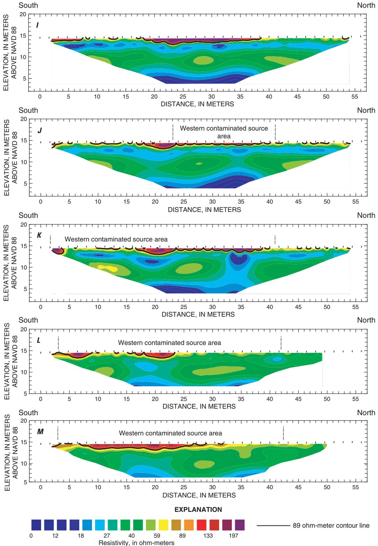
Figure 8. Sections showing inversion results of direct-current resistivity data for (I) line 11, (J) line 12, (K) line 13, (L) line 14, and (M) line 15.—Continued
