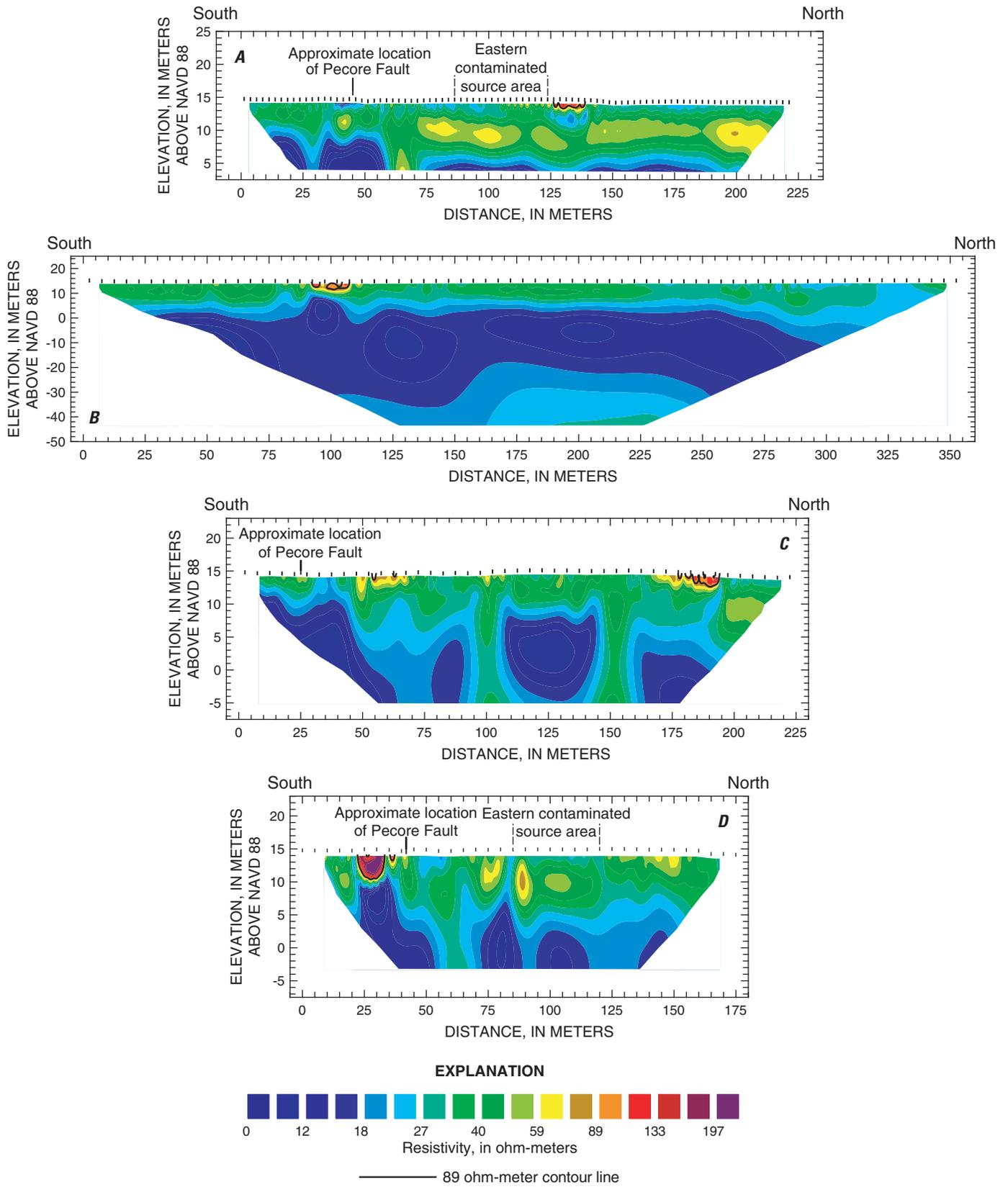
Figure 8. Sections showing inversion results of direct-current resistivity data for (A) line 1, (B) line 2, (C) line 3, and (D) line 5.
