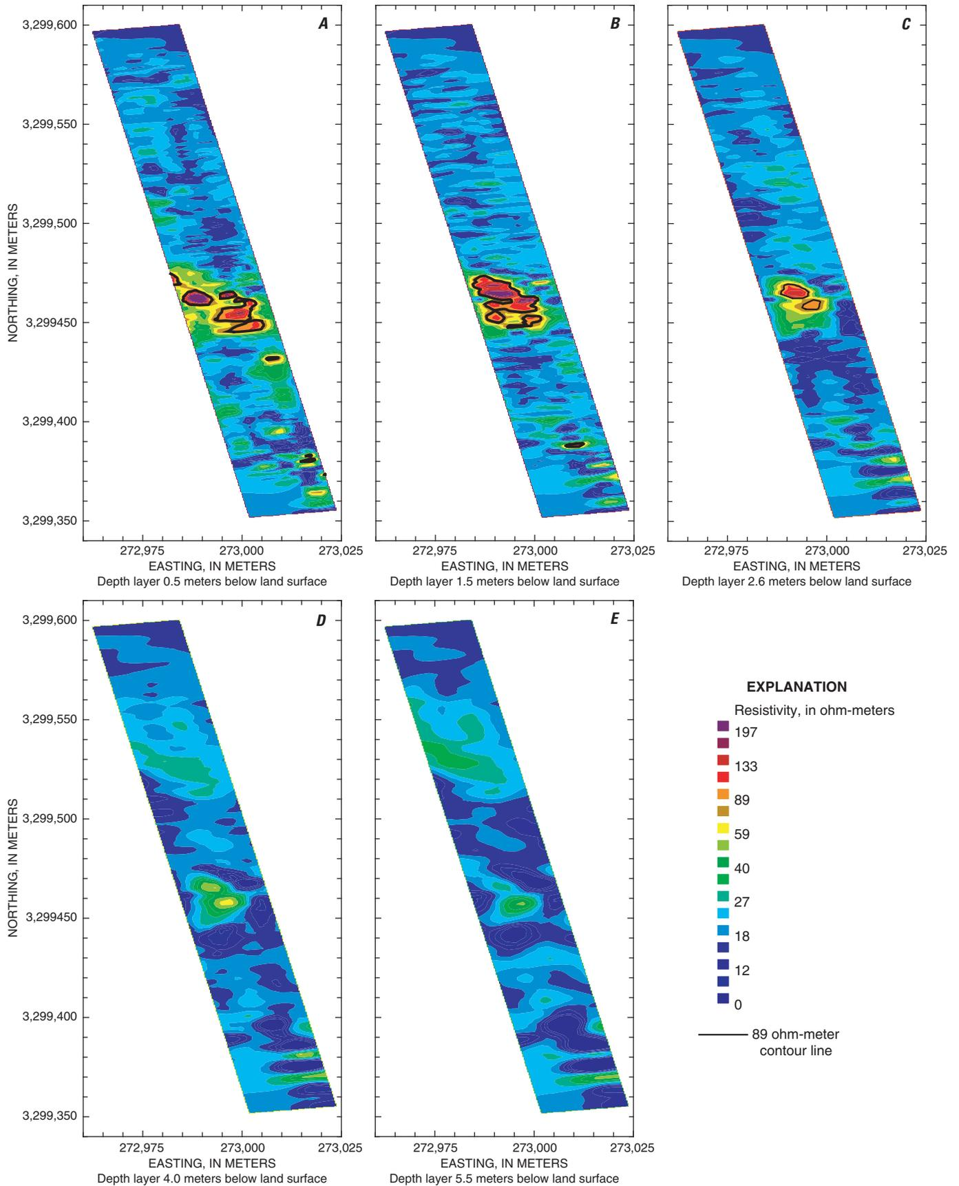
**Figure 5.** Two-dimensional plan view of depth layers showing the inversion results of capacitively coupled resistivity data from lines 1 through 7.
