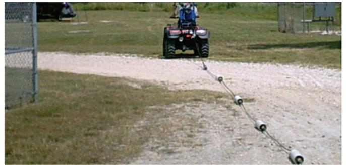
**Figure 3.** Photograph showing the Geometrics OhmMapper capacitively coupled resistivity system towed behind an all-terrain vehicle.
