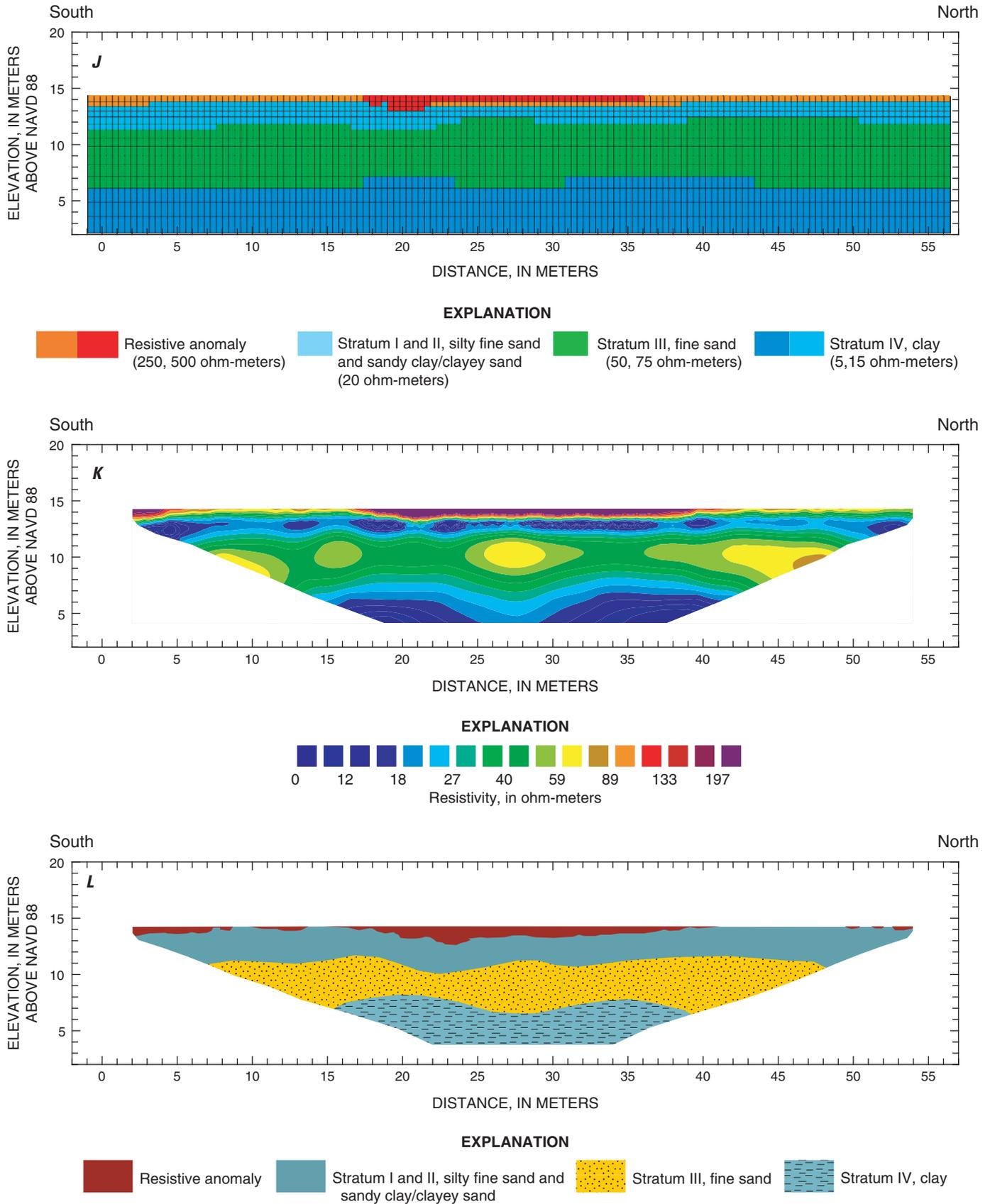
Figure 9. Section showing (J) forward model, (K) inversion result of forward model for direct-current resistivity line 2, and (L) interpretation of direct-current resistivity inversion results of line 11.—Continued
