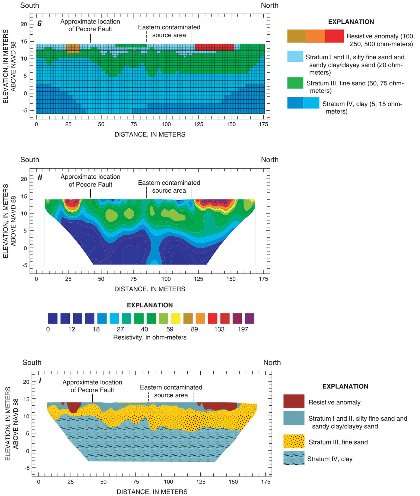
**Figure 9.** Section showing (G) forward model, (H) inversion result of forward model for direct-current resistivity line 6, and (I) interpretation of direct-current resistivity inversion results of line 6.—Continued
