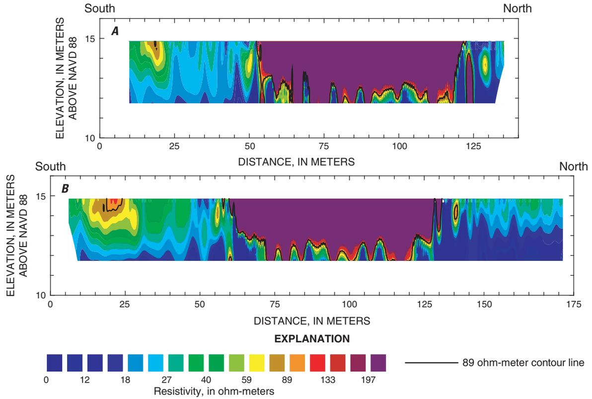
Figure 6. Sections showing inversion results of capacitively coupled resistivity data for (A) line 8 and (B) line 9.
