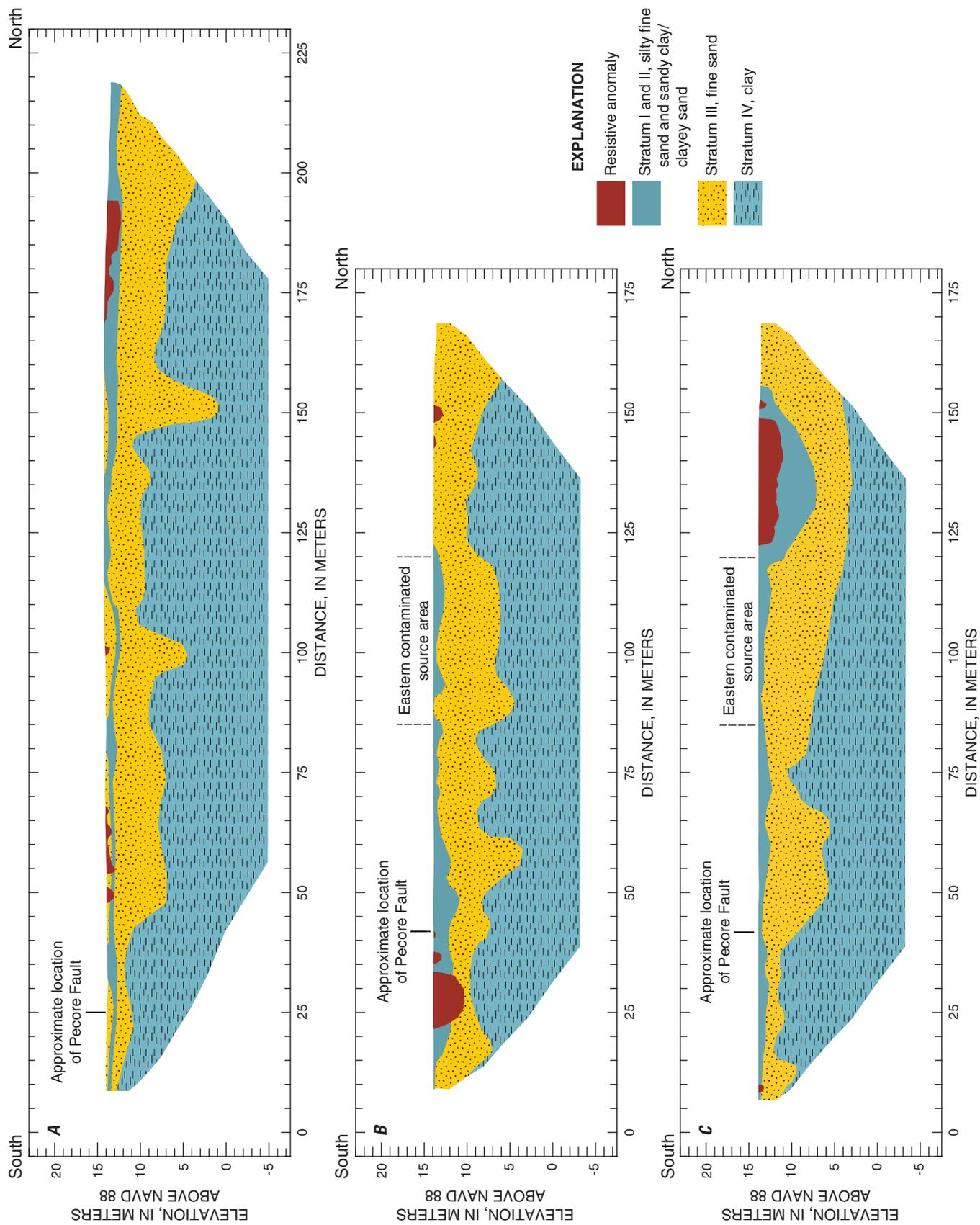
**Figure 10.** Sections showing interpretation of direct-current resistivity inversion results of (A) line 3, (B) line 5, and (C) line 7.
