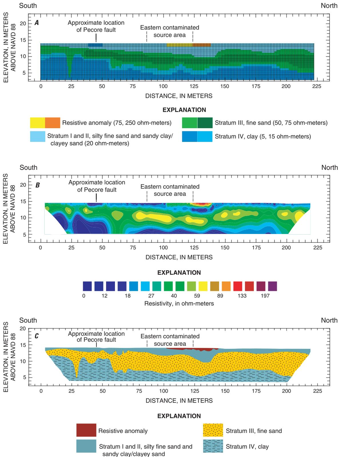
**Figure 9.** Sections showing (A) forward model, (B) inversion result of forward model for direct-current resistivity line 1, and (C) interpretation of direct-current resistivity inversion results of line 1.
