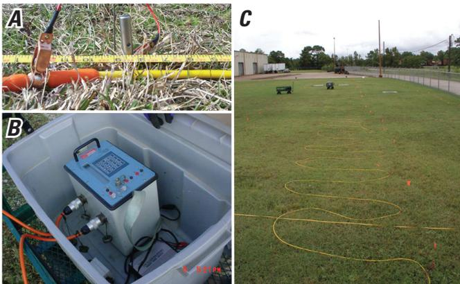
**Figure 4.** Photographs showing (A) a stainless steel electrode connected to the electrode takeout built into the multi-conductor cable, (B) IRIS Syscal R1 Plus resistivity meter connected to multi-conductor cables, and (C) direct-current resistivity equipment set up on survey line 12.
