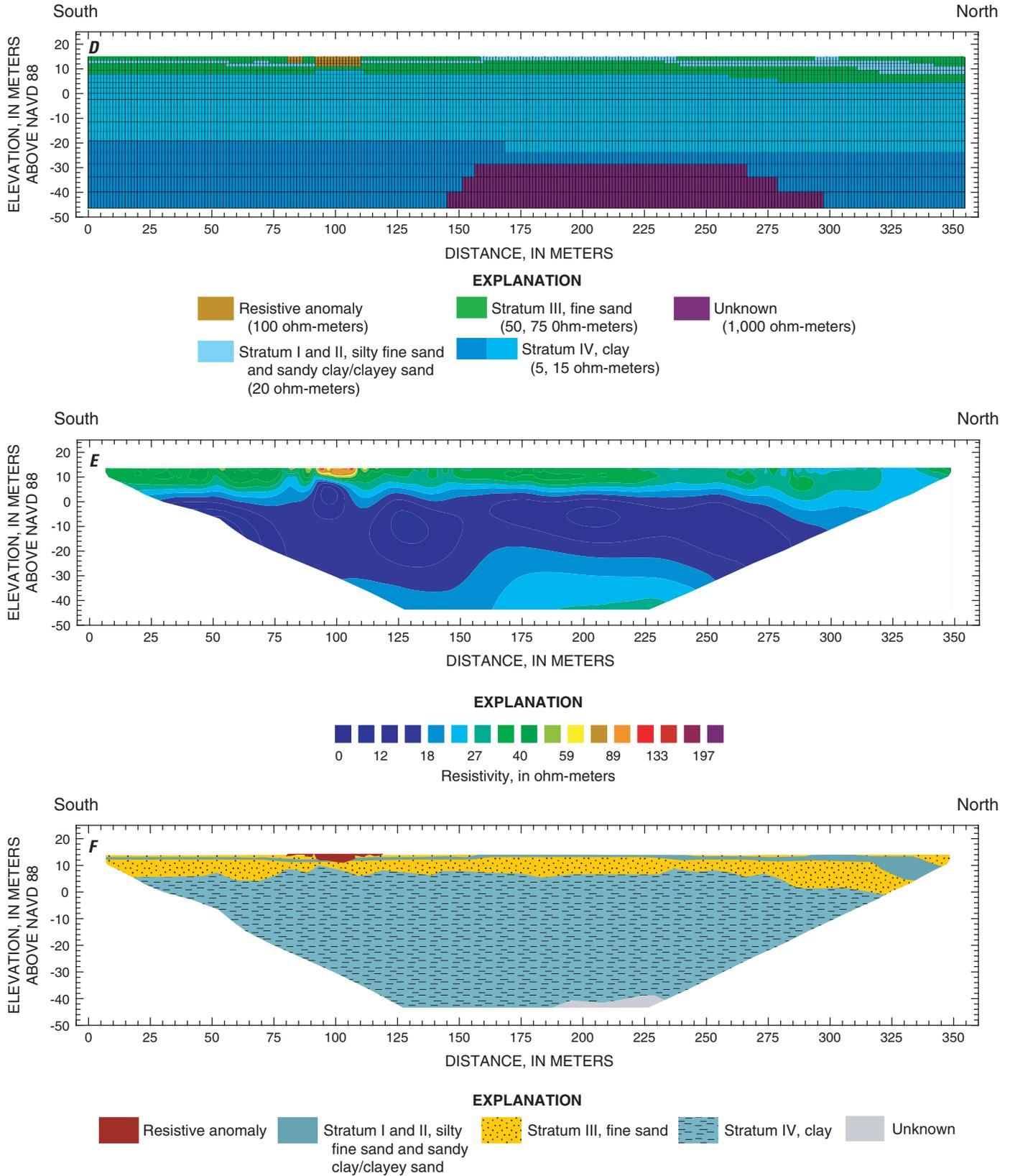
Figure 9. Section showing (D) forward model, (E) inversion result of forward model for direct-current resistivity line 2, and (F) interpretation of direct-current resistivity inversion results of line 2.—Continued
