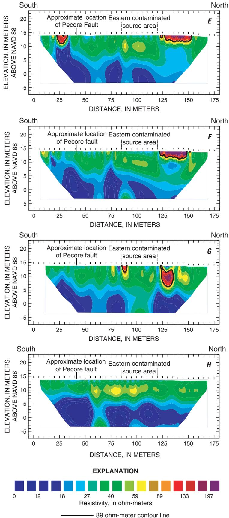
Figure 8. Sections showing inversion results of direct-current resistivity data for (E) line 6, (F) line 7, (G) line 8, and (H) line 9.—Continued
