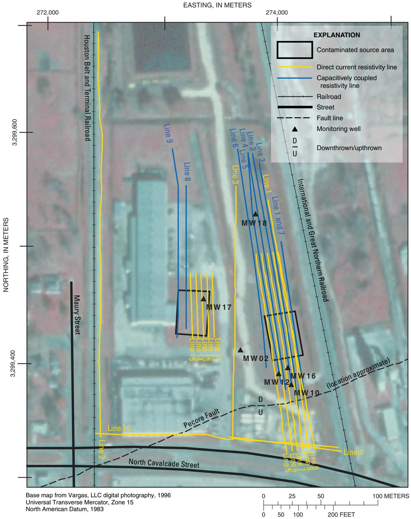
Figure 2. Map of the North Cavalcade Street site showing the direct current and capacitively coupled resistivity data locations, as well as the location of monitoring wells and infrastructure. Location of the contaminated source areas and the Pecore Fault were digitized from Camp Dresser & McGee (figure 2-4 and exhibit 2, 1987).
