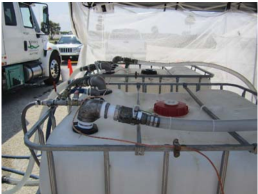
Bonding locations on mixing totes
