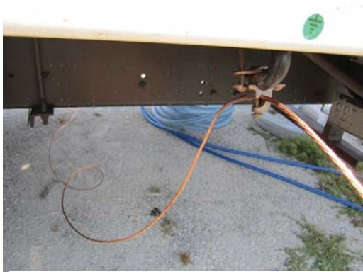
Bonding location on injection Rig
