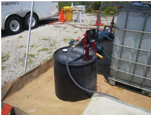
n Butyl Acetate drum pump in protective vapor shield
