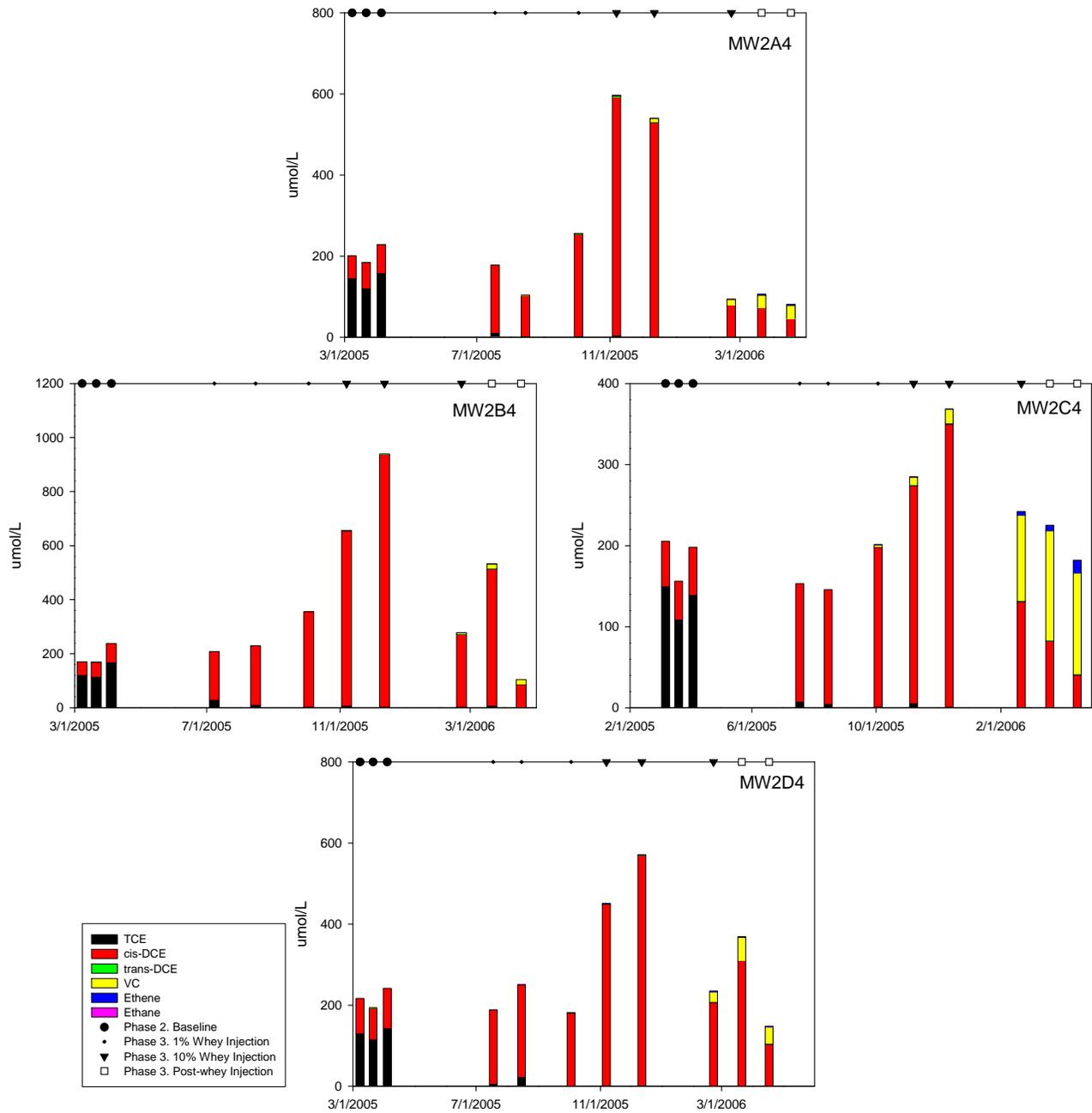
**Figure 9. Trends in Treatment Cell 2 port 4 contaminant molar mass and degradation products during demonstration.**
