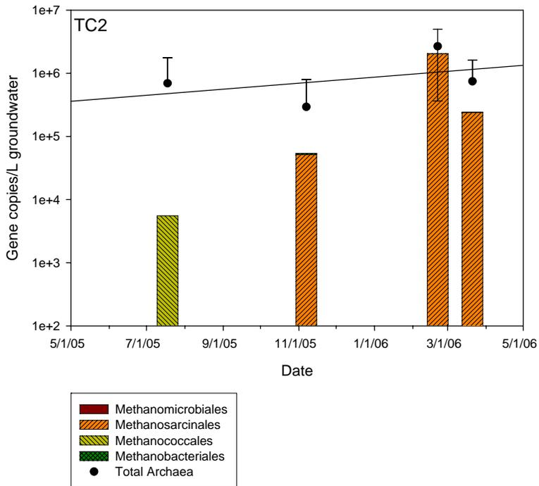
**Figure 5-29. Response of Methanogenic Populations (order level) Using qPCR During Phase 3 Operations, Values Represent the Mean of n=4 (Port 4 of each CMT well) Sampling Points for Each Treatment Cell.**
