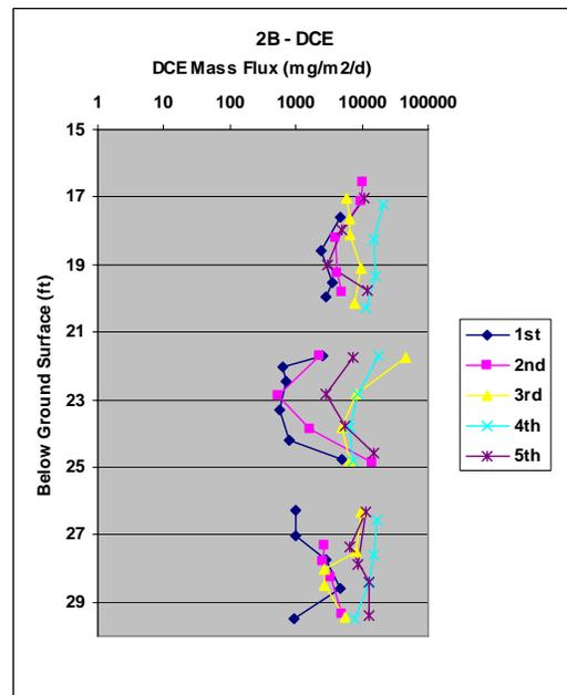
**Figure 5-15. PFM DCE Flux Profiles for 5 Deployment Periods.**
