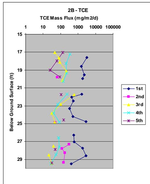
**Figure 5-14. PFM TCE Flux Profiles for 5 Deployment Periods.**
