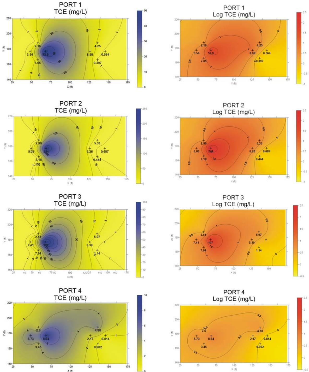
**Figure 5-6. Distribution of TCE in Groundwater Within Two Treatment Cells at Four CMT Depth Intervals: 13-14 ft bgs (Port 1), 18-19 ft bgs (Port 2), 23-24 ft bgs (Port 3), and 28-29 ft bgs (Port 4) During Phase 1 Sampling.**
