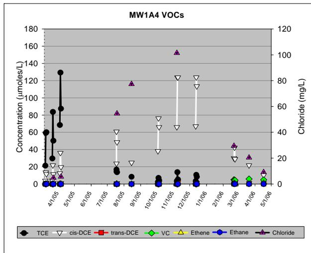
**Figure 5-10. Molar Mass Plots of TCE and Reductive Daughter Products During Phases 2 and 3 of the Demonstration at MWA in Treatment Cell 1. Vertical Lines Illustrate Samples Collected Before, During, and After a Recirculation or Injection Event.**
