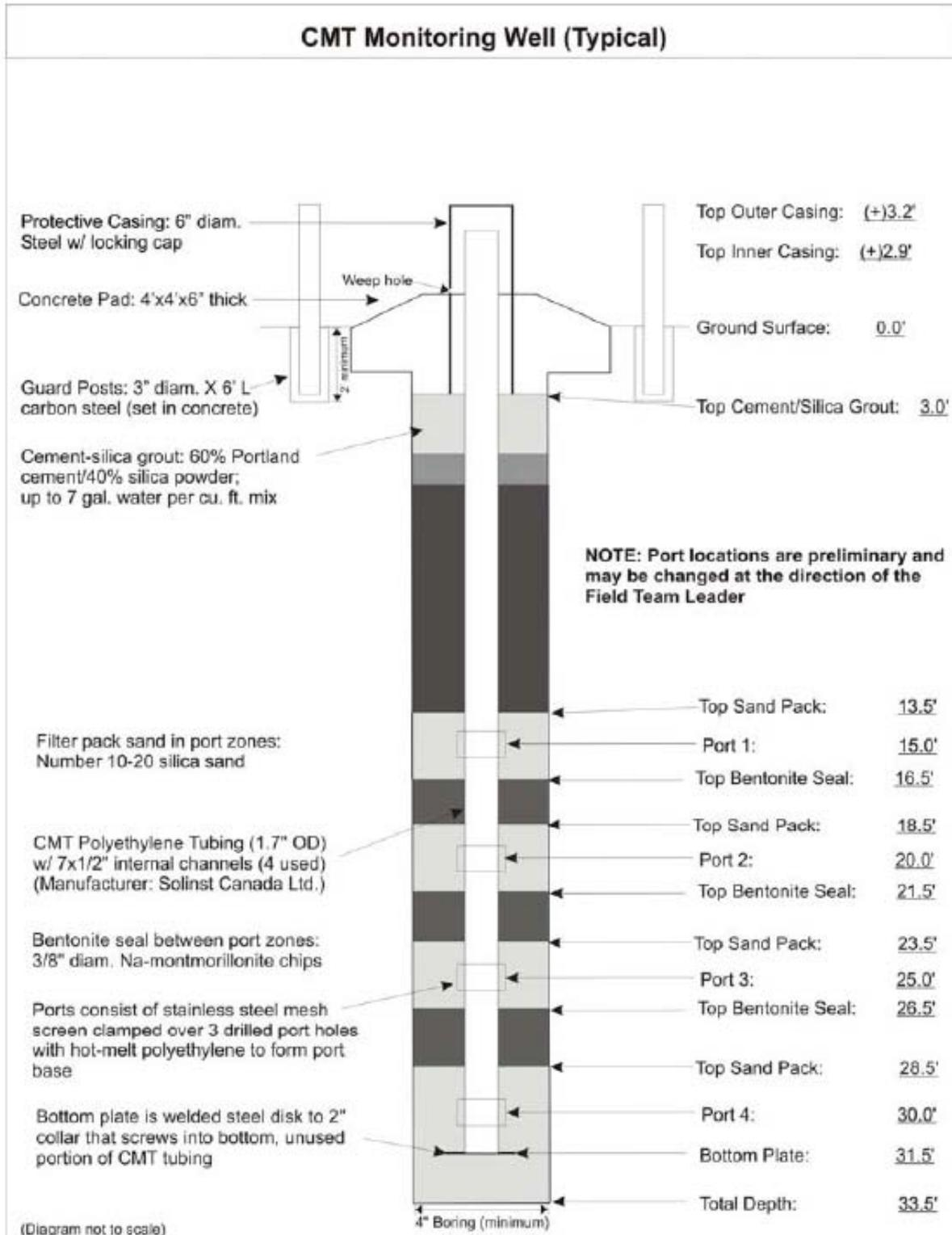
**Figure 2-1. Typical CMT Monitoring Well Configuration.**
