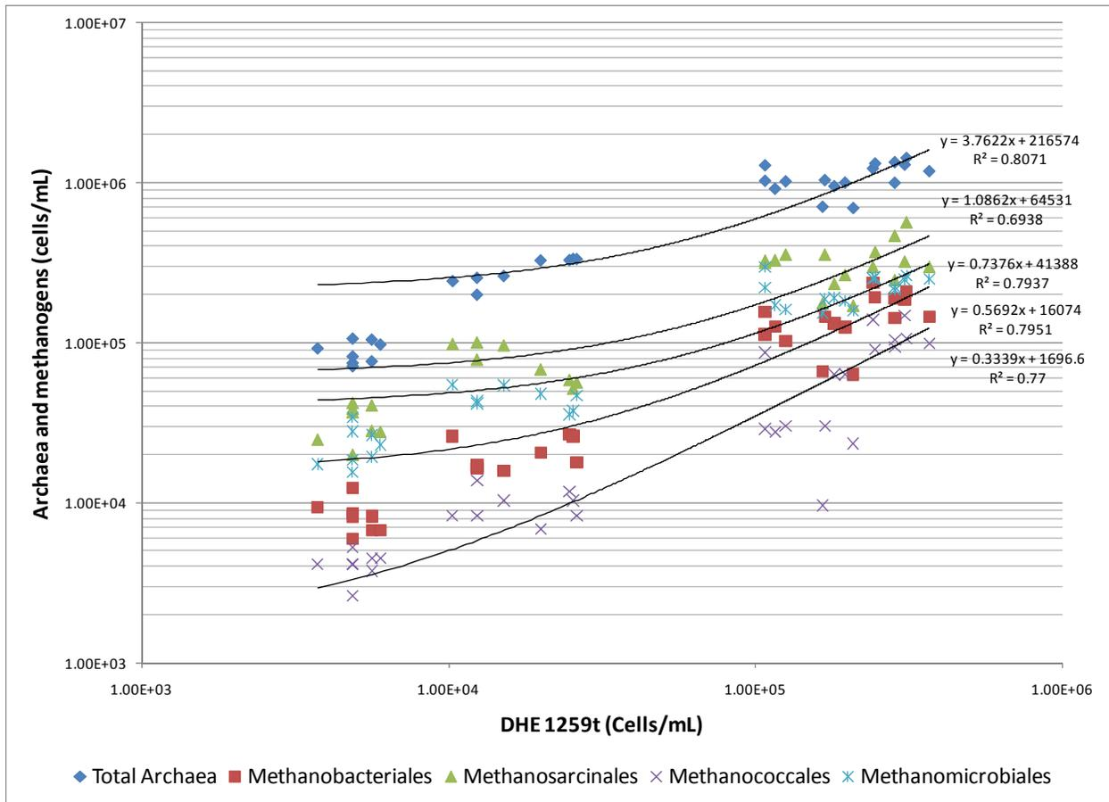
**Figure 5-32. Relationship Between Methanogenic Populations and DHC Using FISH During Phase 3 Operations, Values Represent the Mean of N=4 Sampling Points (Port 4 of Each CMT Well) for Each Treatment Cell.**
