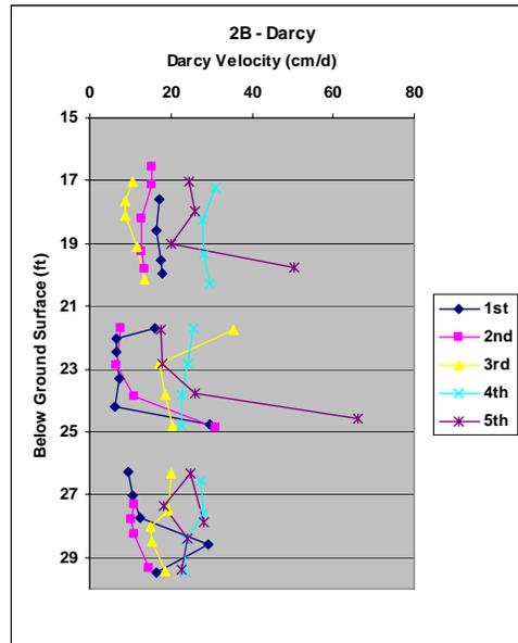
**Figure 5-16. PFM Darcy Velocity Profiles for 5 Deployment Periods.**
