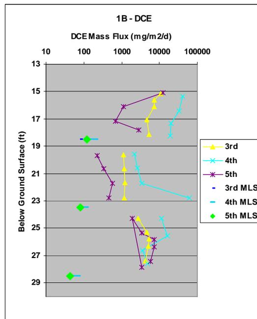
**Figure 5-18. PFM DCE Flux Profiles Compared to CMT MLS Based Calculated Mass Flux Using Average Hydraulic Conductivity and Gradient in Treatment Cell 1.**
