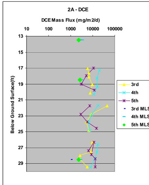
**Figure 5-19. PFM DCE Flux Profiles Compared to CMT MLS Based Calculated Mass Flux Using Average Hydraulic Conductivity and Gradient in Treatment Cell 2.**
