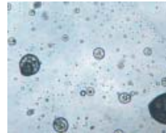
Figure 4: Nano-iron emulsion made with green dyed water dispersed in undyed water
