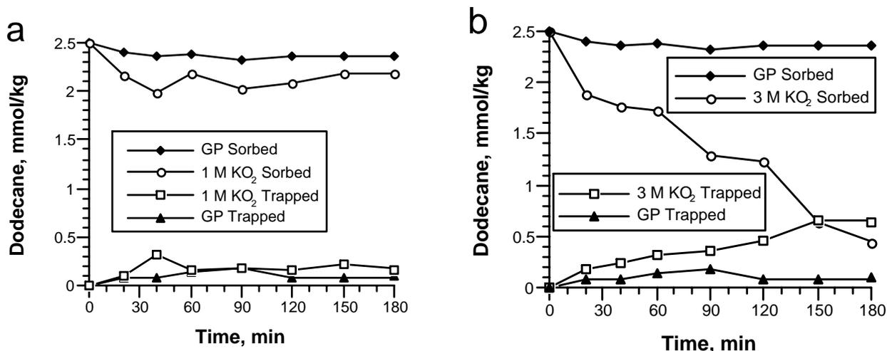
Figure 8.5.2-5. Desorption of dodecane using 1 M potassium superoxide to generate superoxide anion: a) 1 M KO<sub>2</sub>; b) 3 M KO<sub>2</sub> (experimental reactors: 50 g of silica sand spiked with dodecane at 2.5 mmol/kg sand; 0.1 M NaOH, 1 mM DTPA, and 1 M or 3 M KO<sub>2</sub>; 50 ml total volume at pH 14.0; control reactors: KO<sub>2</sub> substituted by deionized water; T = 4 ± 1 °C).
