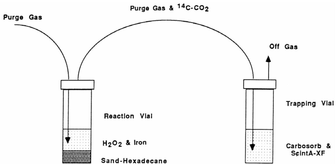
Figure 7.3.4-2. System for trapping  $^{14}\text{C-CO}_2$  evolved from  $^{14}\text{C}$ -hexadecane.
