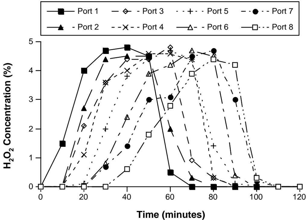
Figure 8.6.6-7. Decomposition of H<sub>2</sub>O<sub>2</sub> stabilized by 25 mM citrate in a column of manganese coated sand (MCS) at pH 7.
