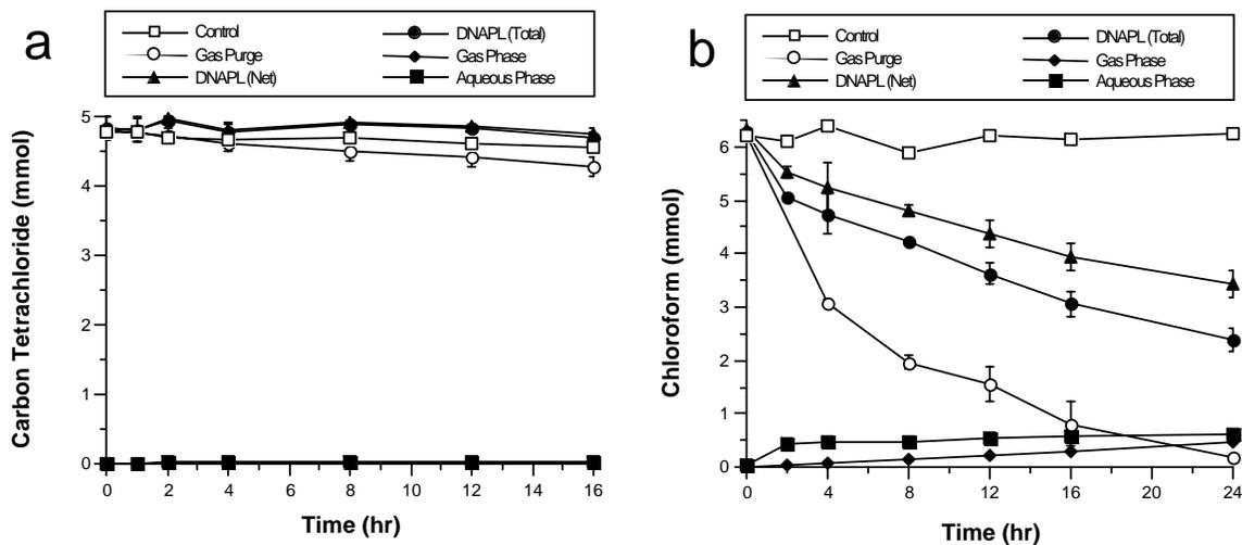
Figure 8.4.2-2. Destruction of (a) carbon tetrachloride and (b) chloroform DNAPLs by hydroxyl radical in standard Fenton's reagent (twenty-four 0.21 mL additions of 1 M hydrogen peroxide and 1 M iron (II)-citrate at pH 1.8 over 48 hr to 7 mL water and 0.5 mL of DNAPL).
