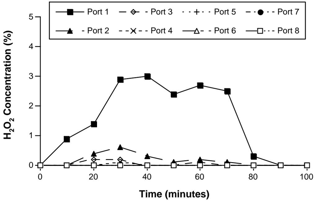
Figure 8.6.6-3. Decomposition of unstabilized H<sub>2</sub>O<sub>2</sub> in a column of iron coated sand (ICS) at pH 7.
