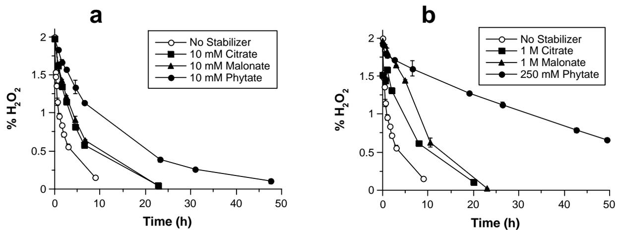
Figure 8.6.5-10. Decomposition of hydrogen peroxide in the Maine soil without stabilization or with addition of citrate, malonate, or phytate. (a) 10 mM stabilizer; (b) 1 M or 250 mM stabilizer
