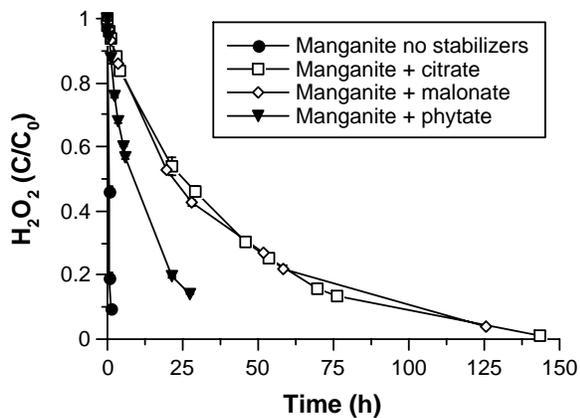
Figure 8.6.5-3. Decomposition of hydrogen peroxide in manganite slurries at pH 3 without stabilization or with addition of 10 mM citrate, malonate, or phytate
