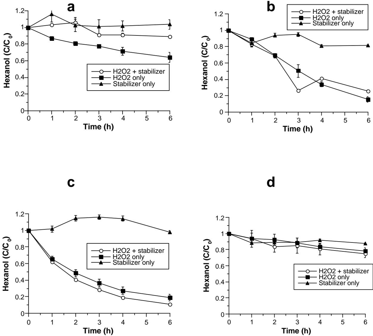
Figure 8.6.5-13. Relative activity of hydroxyl radical measured by hexanol oxidation in four soils with and without stabilization with 10 mM phytate. (a) Georgia soil; (b) Maine soil; (c) California soil; (d) Washington soil.
