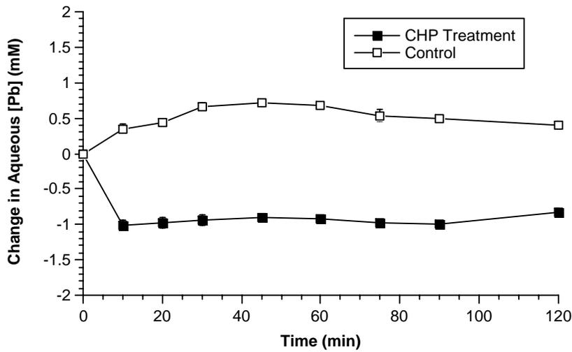
Figure 8.6.3-5. Effect of CHP at pH 7 on the mobility of lead sorbed to the Kamiak Butte soil. [Experimental conditions: 20 mL of 5 mM Pb exchanged onto 1 g Kamiak Butte soil; CHP reactions: 5 mM iron (III)-NTA chelate, and 1.5 M H<sub>2</sub>O<sub>2</sub>; 18 mL total reaction volume; T = 23±°C]
