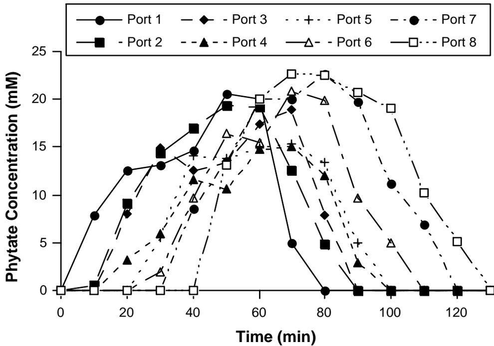
Figure 8.6.6-17. Concentration of phytate in each of eight ports over time in a column of iron coated sand (ICS) containing hexachlorobenzene (HCB) treated with H<sub>2</sub>O<sub>2</sub> stabilized by 25 mM phytate at pH 7.
