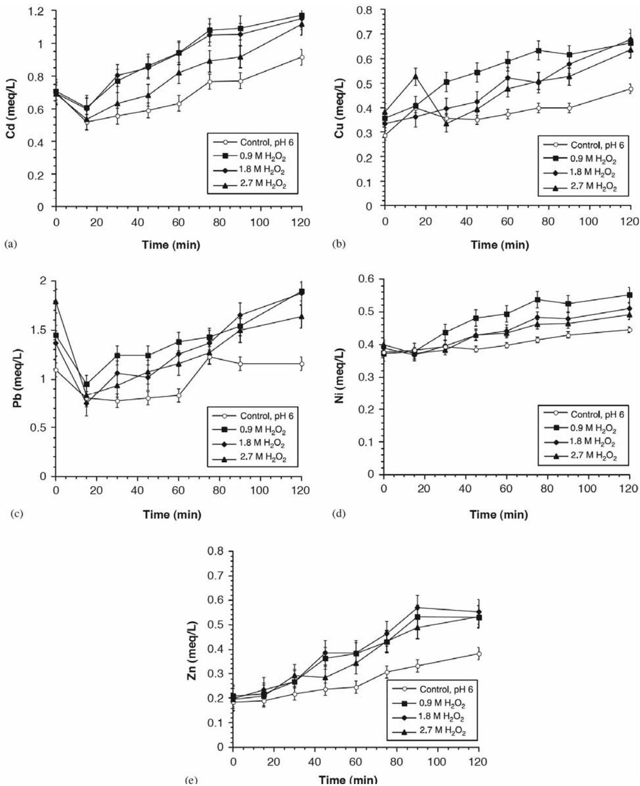
Figure 8.6.2-2. Change in metals mobility after treatment with NTA chelated iron (III) mediated CHP (pH 6) with varying H<sub>2</sub>O<sub>2</sub> concentrations (0 M, 0.9 M, 1.8 M, 2.7 M); a) cadmium; b) copper; c) lead; d) nickel; e) zinc
