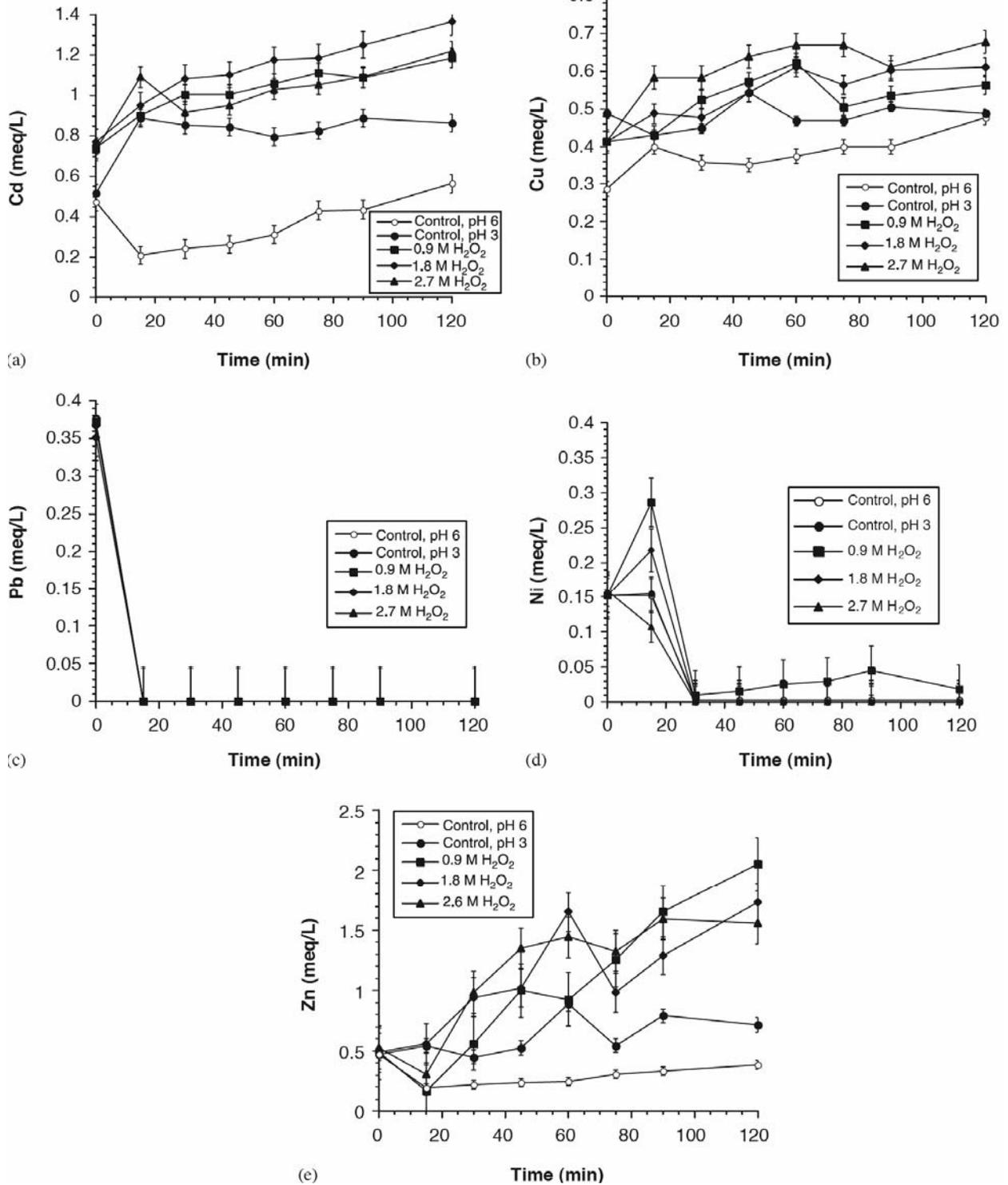
Figure 8.6.2-1. Change in metals mobility after treatment with iron (III) mediated CHP (pH 3) with varying  $H_2O_2$  concentrations (0 M, 0.9 M, 1.8 M, 2.7 M); a) cadmium; b) copper; c) lead; d) nickel; e) zinc
