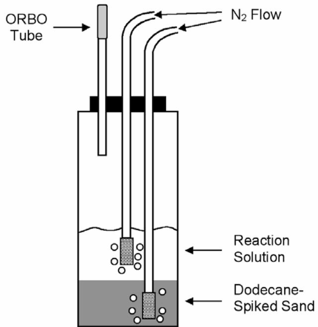
Figure 7.5.2-1. Experimental reactor used for desorption experiments.
