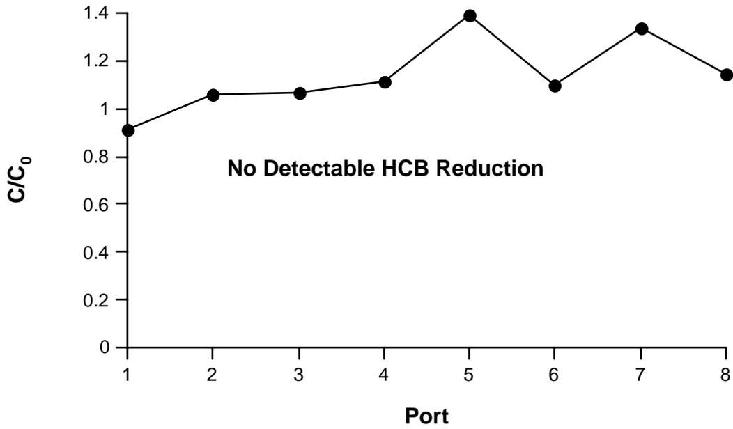
Figure 8.6.6-13. Relative concentration of hexachlorobenzene (HCB) in each of eight ports in a column of manganese coated sand (MCS) treated with H<sub>2</sub>O<sub>2</sub> stabilized by 25 mM phytate at pH 7.
