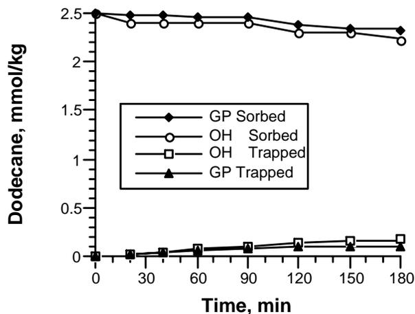
Figure 8.5.2-3. Desorption of dodecane using the standard Fenton's reaction optimized for the generation of hydroxyl radicals (experimental reactors: 50 g of silica sand spiked with dodecane at 2.5 mmol/kg sand; 5 mM Fe(III) with 0.1 ml of 100 mM H<sub>2</sub>O<sub>2</sub> added every 10 min over 180 min; 50 ml initial volume at pH 3.0; control reactors: H<sub>2</sub>O<sub>2</sub> substituted by deionized water; T = 20 ± 2°C).
