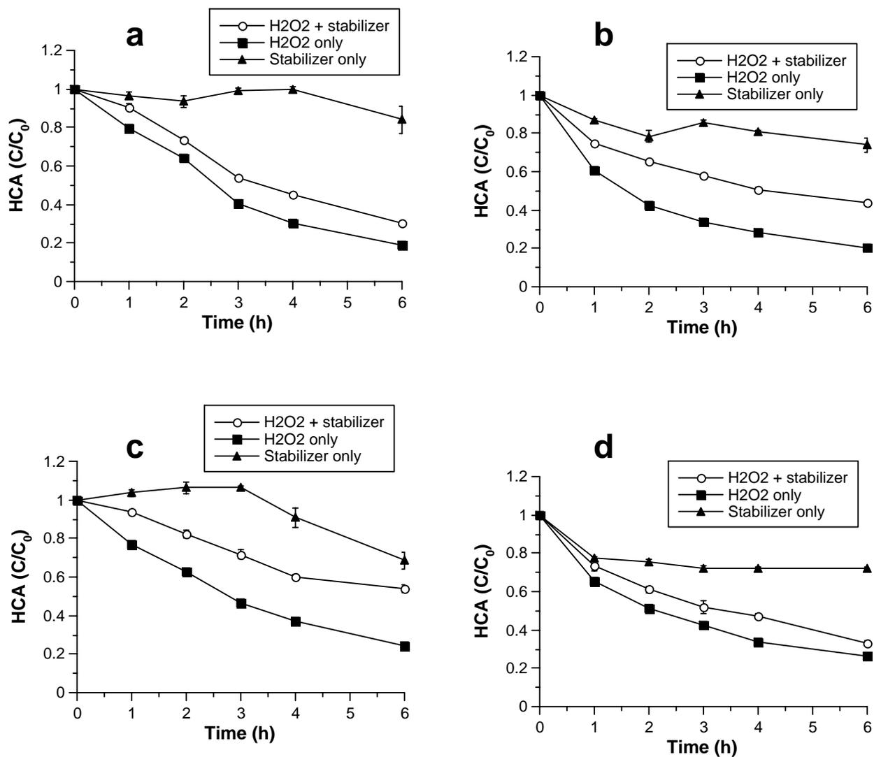
Figure 8.6.5-16. Relative activity of superoxide measured by hexachloroethane (HCA) destruction in four soils with and without stabilization with 10 mM phytate. (a) Georgia soil; (b) Maine soil; (c) California soil; (d) Washington soil.
