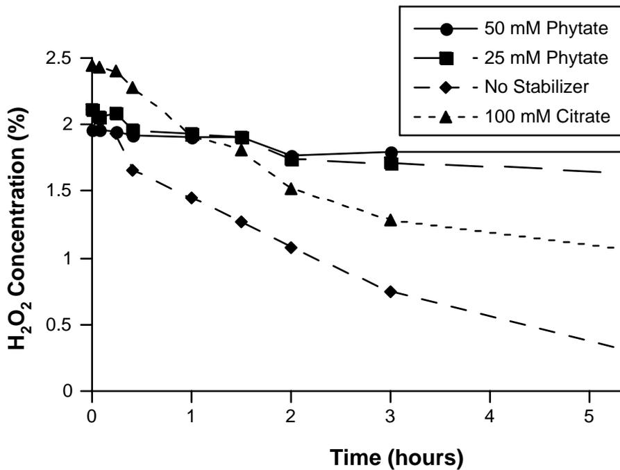
Figure 8.6.6-1. Rate of stabilized and unstabilized H<sub>2</sub>O<sub>2</sub> decomposition in a column of iron coated sand (ICS).
