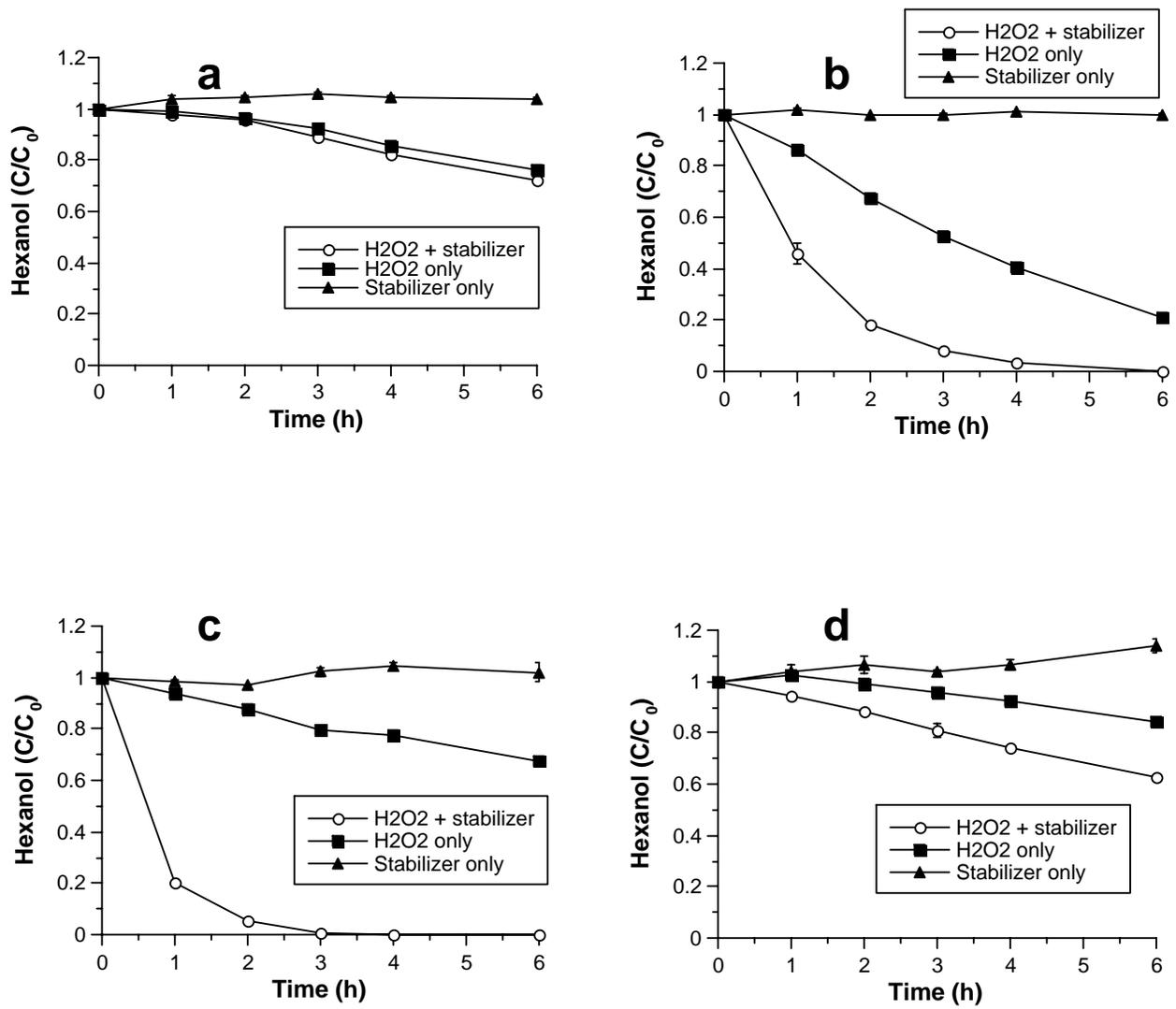
Figure 8.6.5-15. Relative activity of hydroxyl radical measured by hexanol oxidation in four soils with and without stabilization with 10 mM malonate. (a) Georgia soil; (b) Maine soil; (c) California soil; (d) Washington soil.
