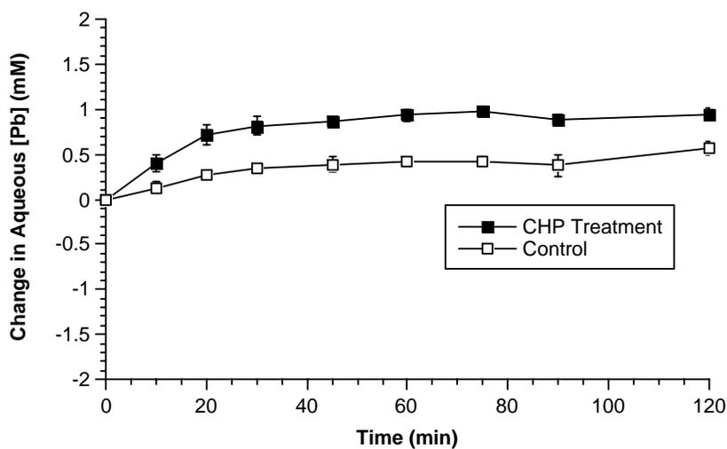
Figure 8.6.3-3. Effect of CHP at pH 3 on the mobility of lead sorbed to the Colorado soil. [Experimental conditions: 20 mL of 5 mM Pb exchanged onto 1 g Colorado soil; CHP reactions: 5 mM iron (III), and 1.5 M H<sub>2</sub>O<sub>2</sub>; 18 mL total reaction volume; T = 23±°C]
