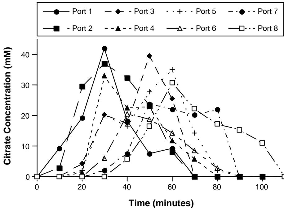
Figure 8.6.6-15. Concentration of citrate in each of eight ports over time in a column of manganese coated sand (MCS) containing hexachlorobenzene (HCB) treated with  $H_2O_2$  stabilized by 25 mM citrate at pH 7.
