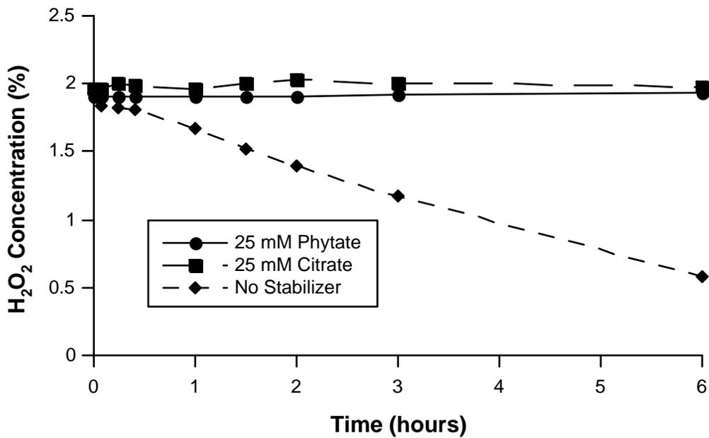
Figure 8.6.6-2. Rate of stabilized and unstabilized H<sub>2</sub>O<sub>2</sub> decomposition in a column of manganese coated sand (MCS).
