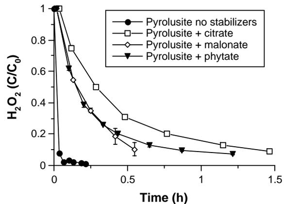
Figure 8.6.5-4. Decomposition of hydrogen peroxide in pyrolusite slurries at pH 3 without stabilization or with addition of 10 mM citrate, malonate, or phytate
