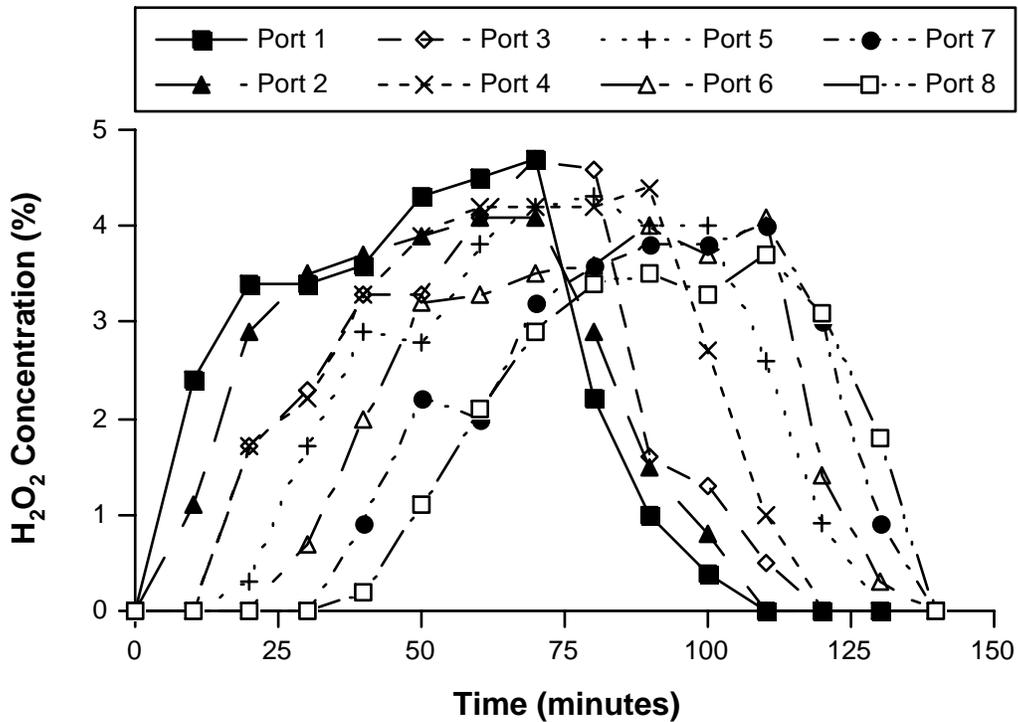
Figure 8.6.6-5, Decomposition of unstabilized H<sub>2</sub>O<sub>2</sub> in a column of manganese coated sand (MCS) at pH 7.
