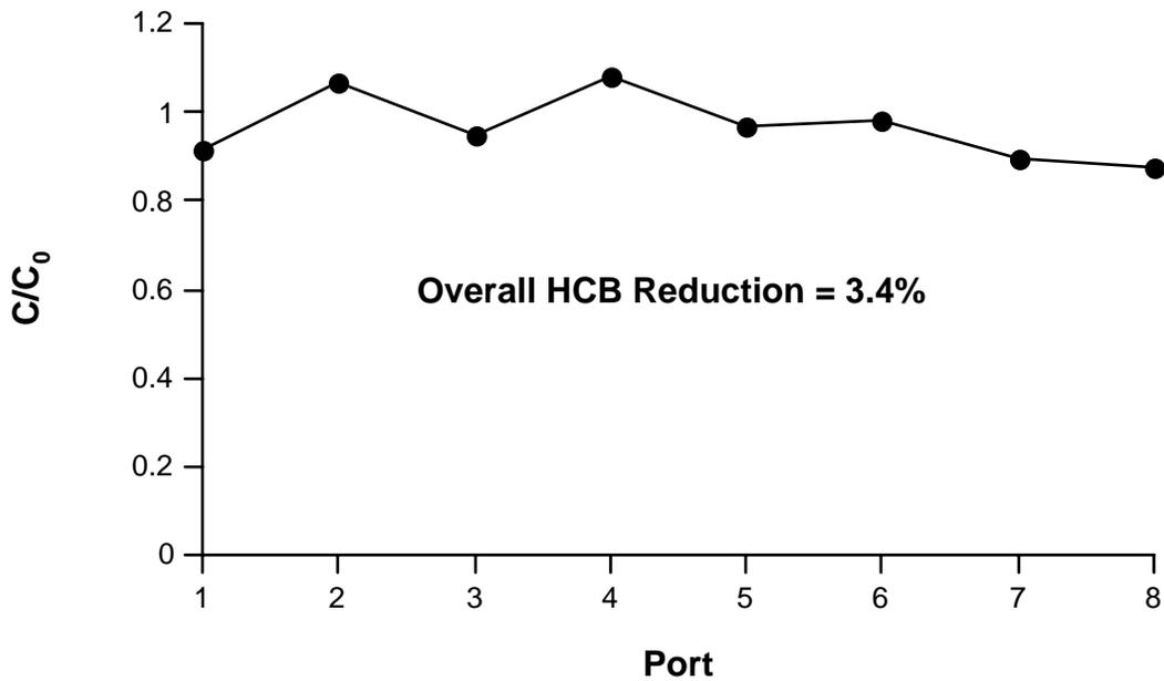
Figure 8.6.6-10. Relative concentration of hexachlorobenzene (HCB) in each of eight ports in a column of manganese coated sand (MCS) treated with unstabilized  $H_2O_2$  at pH 3.
