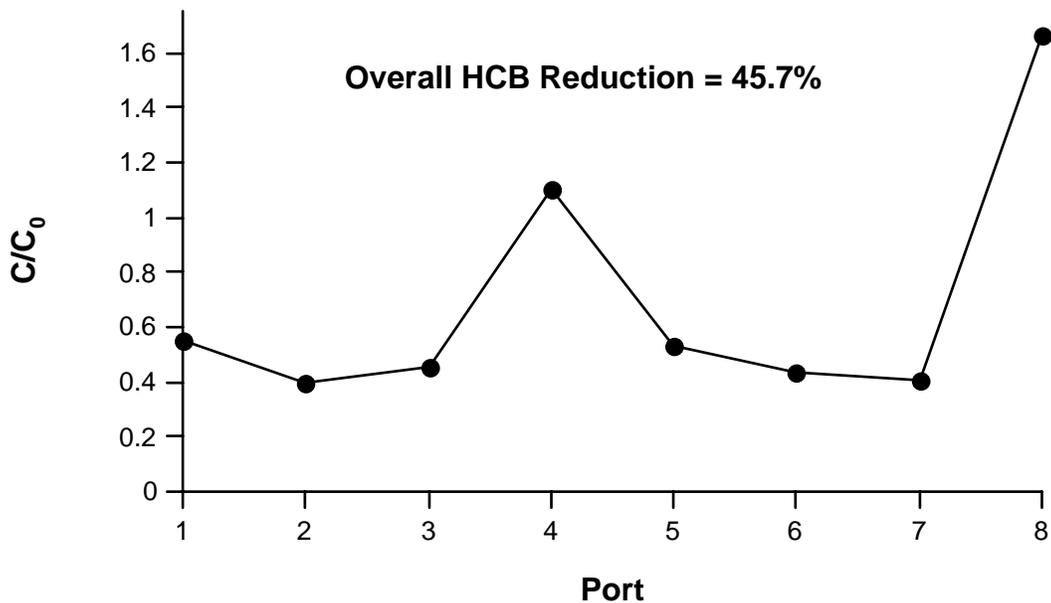
Figure 8.6.6-11. Relative concentration of hexachlorobenzene (HCB) in each of eight ports in a column of manganese coated sand (MCS) treated with unstabilized  $H_2O_2$  at pH 7.
