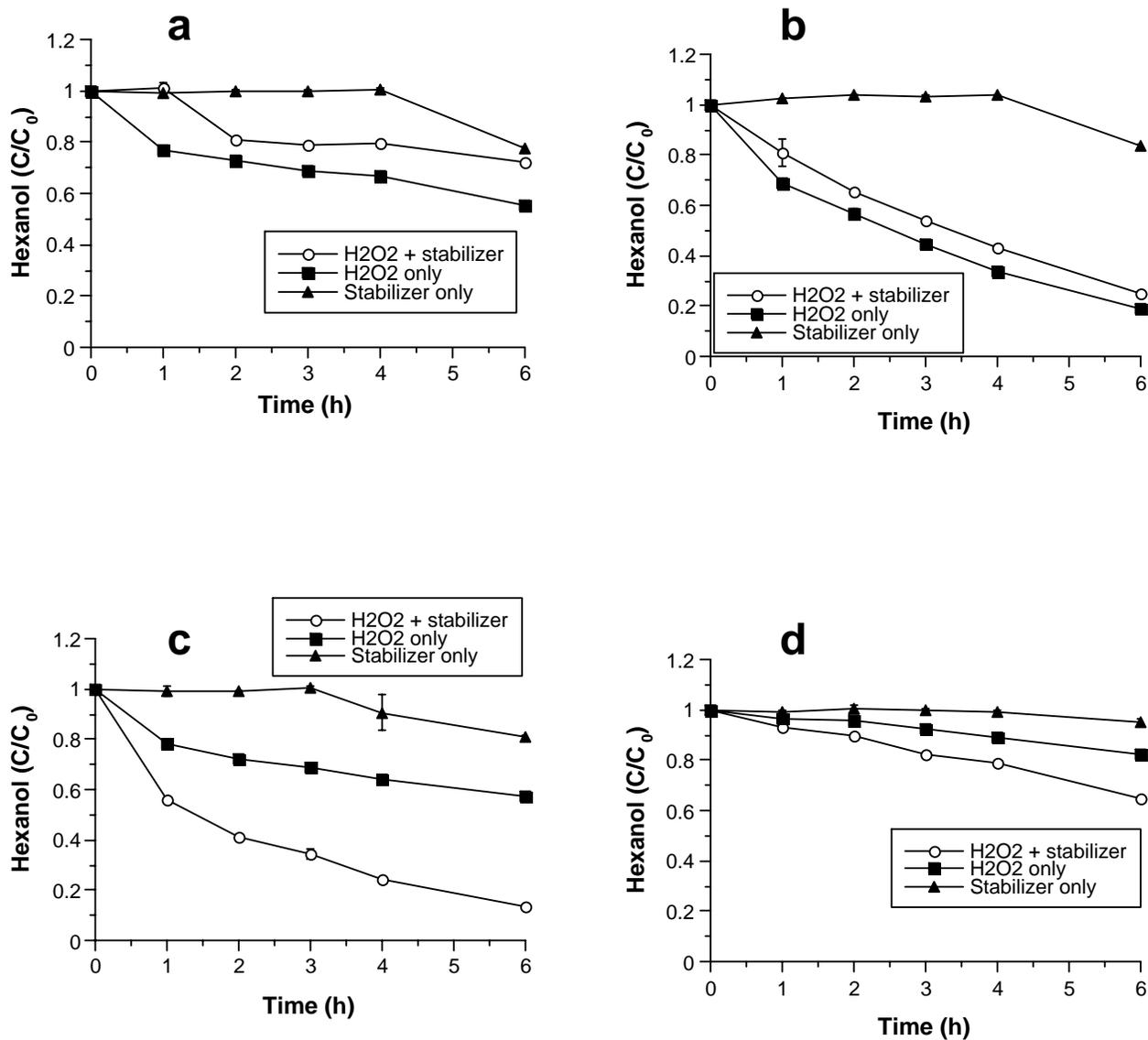
Figure 8.6.5-14. Relative activity of hydroxyl radical measured by hexanol oxidation in four soils with and without stabilization with 10 mM citrate. (a) Georgia soil; (b) Maine soil; (c) California soil; (d) Washington soil.
