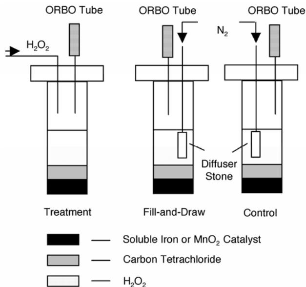
Figure 7.4.1-1. Schematic drawing of the experimental setup for the study of DNAPL destruction using soluble iron- or MnO<sub>2</sub>-catalyzed CHP reactions.
