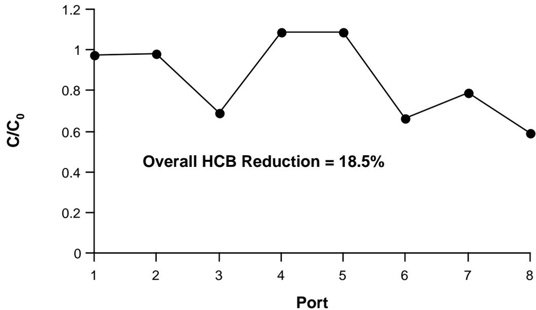
Figure 8.6.6-8. Relative concentration of hexachlorobenzene (HCB) in each of eight ports in a column of iron coated sand (ICS) treated with unstabilized H<sub>2</sub>O<sub>2</sub> at pH 3.
