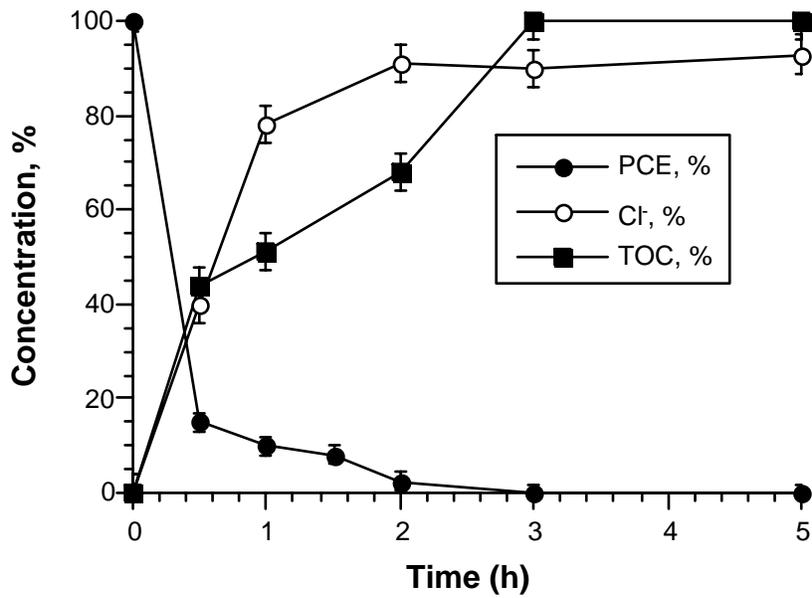
Figure 8.3.2-1. Perchloroethylene degradation by CHP over time. Initial PCE concentration: 1000 mg/kg sand. The TOC (CO<sub>2</sub>) and Cl<sup>-</sup> concentrations are expressed as the equivalent amount of PCE.
