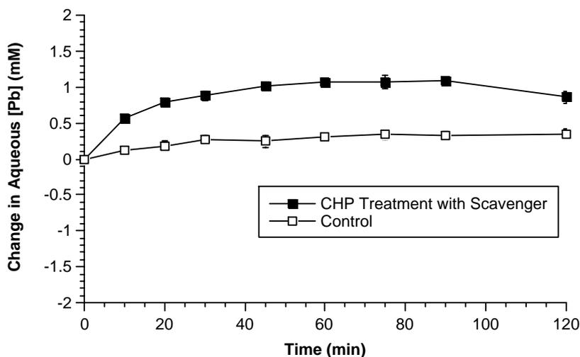
Figure 8.6.3-7. Effect of hydroxyl radical scavenging on the mobility of lead sorbed to Hanford soil during CHP treatment at pH 3. [Experimental conditions: 20 mL of 3 mM Pb exchanged onto 1 g Hanford soil; CHP reactions: 5 mM iron (III), 1.5 M H<sub>2</sub>O<sub>2</sub> and 1.3 M isopropanol; 19.9 mL total reaction volume; T = 23±°C]
