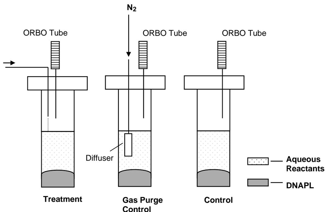
Figure 7.4.2-1. Experimental apparatus for evaluating the destruction of TCE and PCE DNAPLs.
