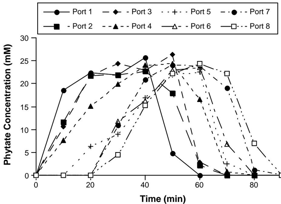
Figure 8.6.6-16. Concentration of phytate in each of eight ports over time in a column of manganese coated sand (MCS) containing hexachlorobenzene (HCB) treated with  $H_2O_2$  stabilized by 25 mM phytate at pH 7.
