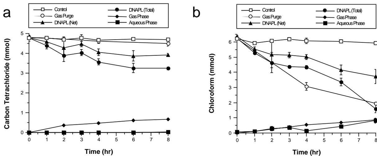
Figure 8.4.2-5. Destruction of (a) carbon tetrachloride and (b) chloroform DNAPLs in a potassium superoxide-based superoxide system with the cosolvent acetone (2 M potassium superoxide and 1 M acetone at pH 14.0).
