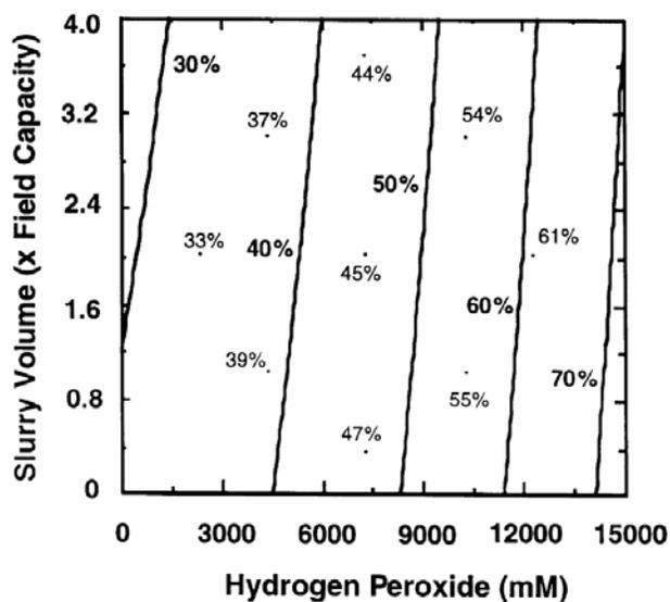
Figure 8.3.3-1. Response surface for the mineralization of  $^{14}\text{C}$ -BaP as a function of  $\text{H}_2\text{O}_2$  concentration and slurry volume in silica sand catalyzed by 6.6 mM iron (II). Isoconcentration lines represent the per cent BaP recovered as  $^{14}\text{C}$ - $\text{CO}_2$  described by equation 5. The field capacity of the silica sand = 0.31 ml/g.
