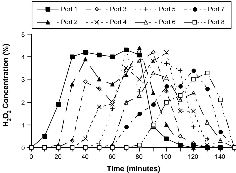
Figure 8.6.6-4. Decomposition of H<sub>2</sub>O<sub>2</sub> stabilized by 25 mM phytate in a column of iron coated sand (ICS) at pH 7.
