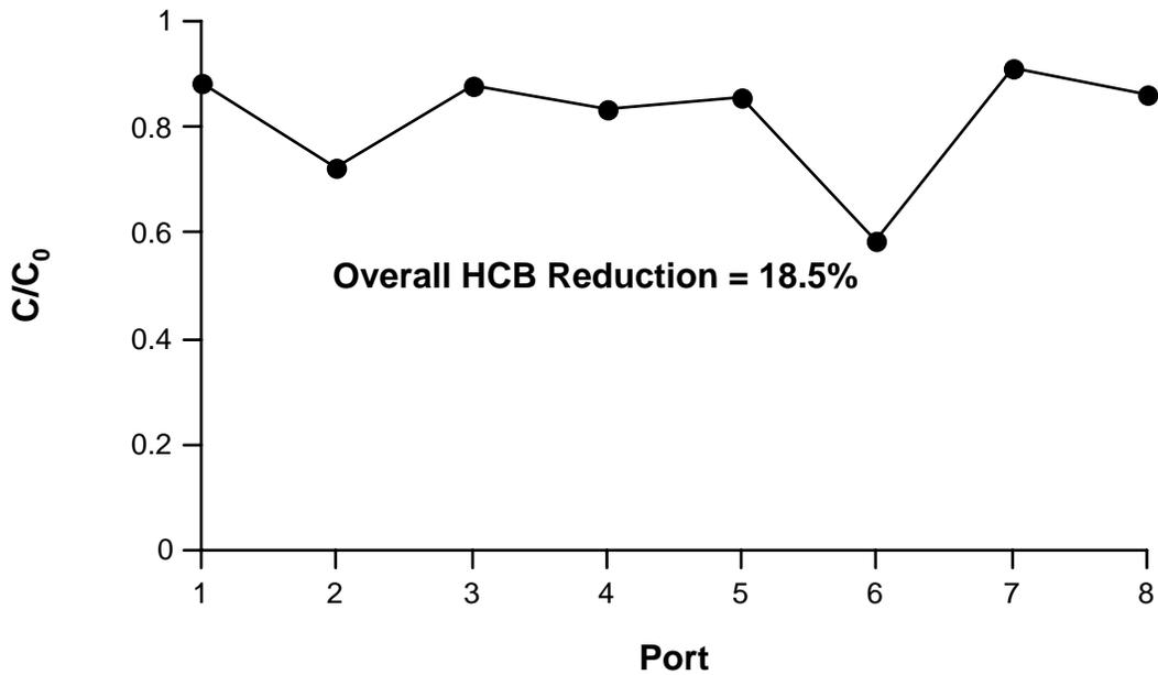
Figure 8.6.6-14. Relative concentration of hexachlorobenzene (HCB) in each of eight ports in a column of iron coated sand (ICS) treated with H<sub>2</sub>O<sub>2</sub> stabilized by 25 mM phytate at pH 7.
