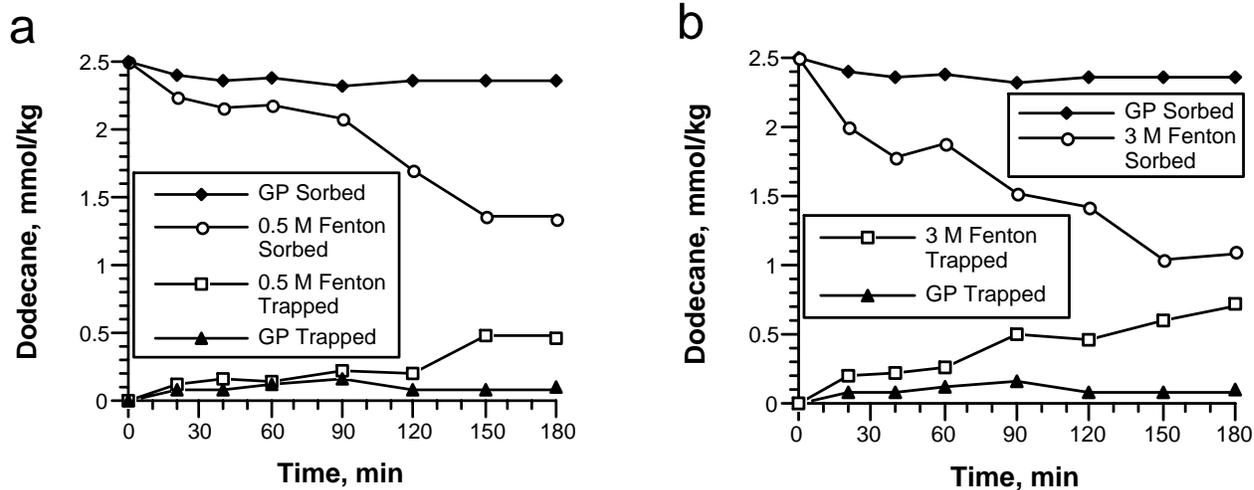
Figure 8.5.2-2. Desorption of dodecane by a CHP reaction: a) 0.5 M H<sub>2</sub>O<sub>2</sub>; b) 3 M H<sub>2</sub>O<sub>2</sub> (experimental reactors: 50 g of silica sand spiked with dodecane at 2.5 mmol/kg sand; 5 mM Fe(III) and 0.5 M or 3 M H<sub>2</sub>O<sub>2</sub>; 50 ml total volume at pH 3.0; control reactors: H<sub>2</sub>O<sub>2</sub> substituted by deionized water; T = 20 ± 2°C).
