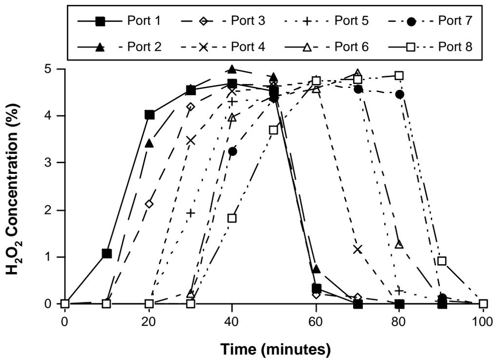
Figure 8.6.6-6. Decomposition of H<sub>2</sub>O<sub>2</sub> stabilized by 25 mM phytate in a column of manganese coated sand (MCS) at pH 7.
