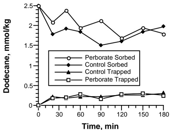
Figure 8.5.2-4. Linear regression of desorption of dodecane using sodium perborate to generate hydroperoxide anion (experimental reactors: 50 g of silica sand spiked with dodecane at 2.5 mmol/kg sand; 150 mM sodium perborate; 50 ml total volume at pH 10.0; control reactors: sodium perborate substituted by deionized water; T = 20 ± 2°C).
