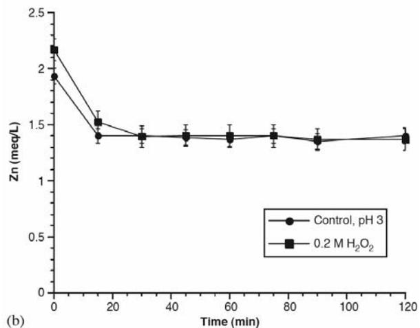
Figure 8.6.2-3. Change in metals mobility after treatment with iron (III) mediated CHP (pH 3) using 0.2 M H<sub>2</sub>O<sub>2</sub>; a) nickel; b) zinc
