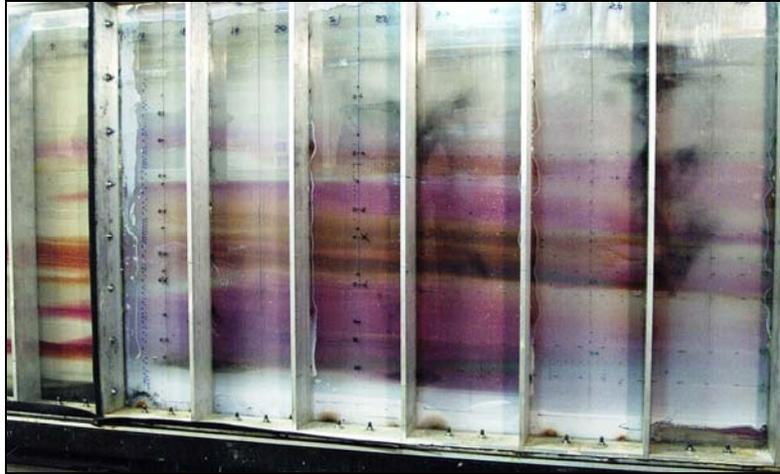
Figure 3.92. Oxidation during ISCO Low Heterogeneity Experiment
