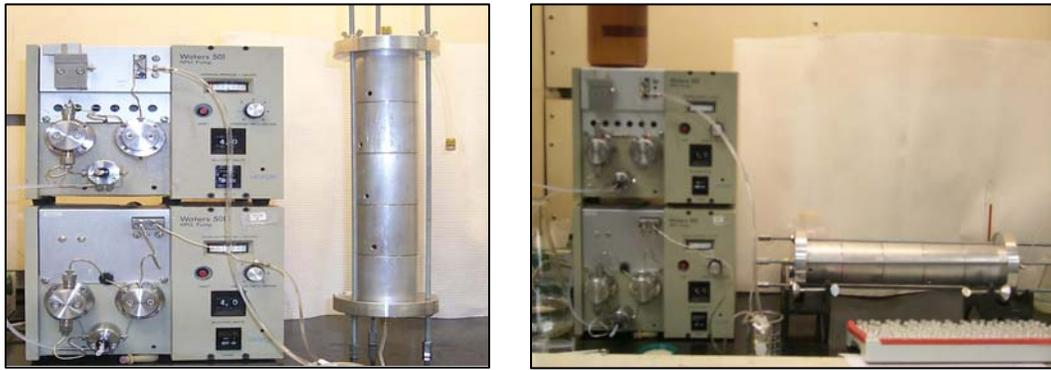
Figure 3.38. Setup for Column Experiments with Surfactants
