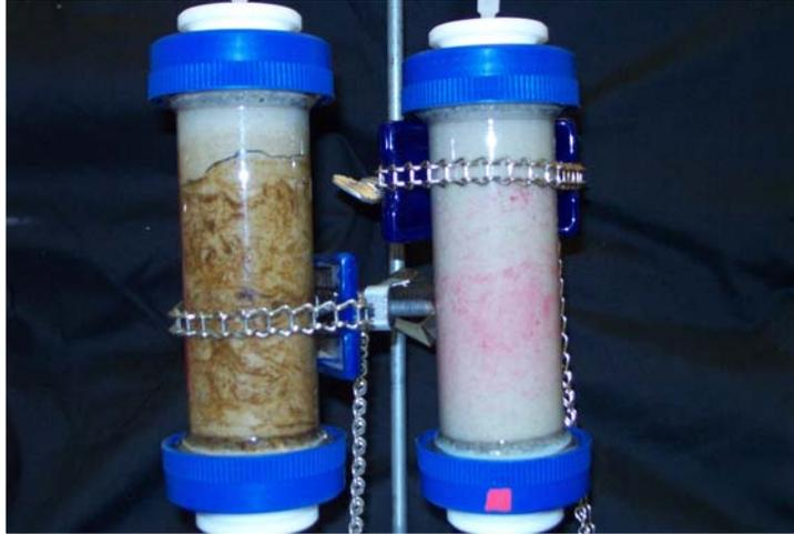
Figure 3.8. Columns for Partition Tracer Tests with Surfactant Treatment (pure TCE DNAPL, dyed at right and field DNAPL at left)
