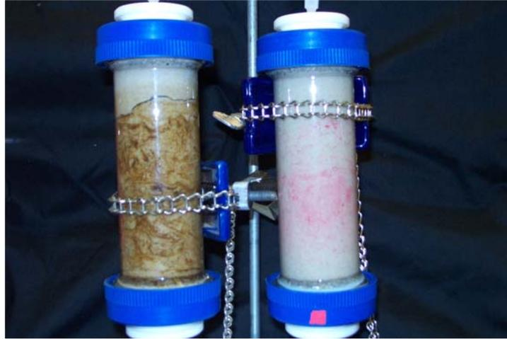
Figure 3.42. Setup for Column Experiments with SEAR Comparing Mass Transfer from Pure TCE-DNAPL and a Field DNAPL
