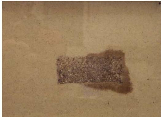
Figure 3.46. Remobilization of Field DNAPL during Surfactant Flushing
