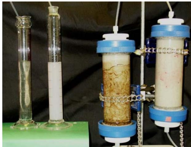
Figure 3.43. Difference in Column Effluents During Surfactant Flushing for Field DNAPL (Left Volumetric Cylinder) and Pure TCE-DNAPL (Right Volumetric Cylinder)
