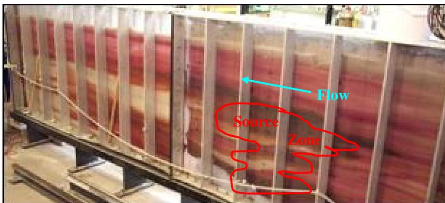
Figure 3.91. Oxidation during ISCO High Heterogeneity Experiment
