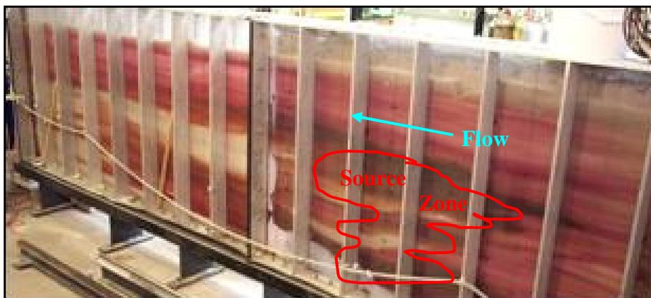
Figure A1.16. Large-Scale Tank during Chemical Oxidation.
