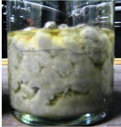
Photo 1. Example Design Mix – 300g of AquaBlok+ORGANOCLAY 4060 Blend Sample (120g of Active Organoclay), 3wks After Addition of 185ml Motor Oil.
