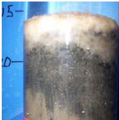
**Figure 5-15. Core sample after treatment. Artificial Sediment is the Light-Colored Material** (Petsonk et al., 2005)
