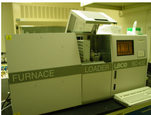
Figure 2. LECO SC-432 for the analysis of total sulfur in coal and coal combustion by-products.
