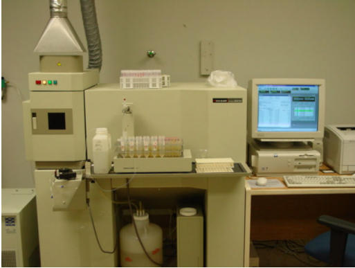
Figure 3. Perkin-Elmer's Optima 3300DV ICP-AES for multi-element analysis of coal ash and coal combustion by-products.
