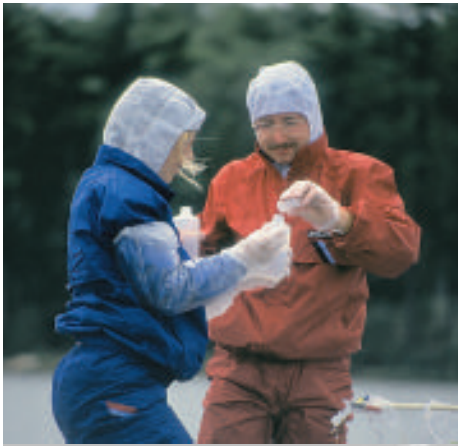
Figure 3. Because there is actually very little mercury in most natural waters, scientists have to use extreme measures when sampling for mercury to avoid sample contamination from their hands and clothing. This entails the use of lint-free suits, plastic gloves, hoods, and stringently cleaned sampling equipment.
