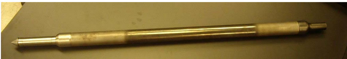
Figure D-1b. Modified Geoprobe® Groundwater Profiler – Assembled.
