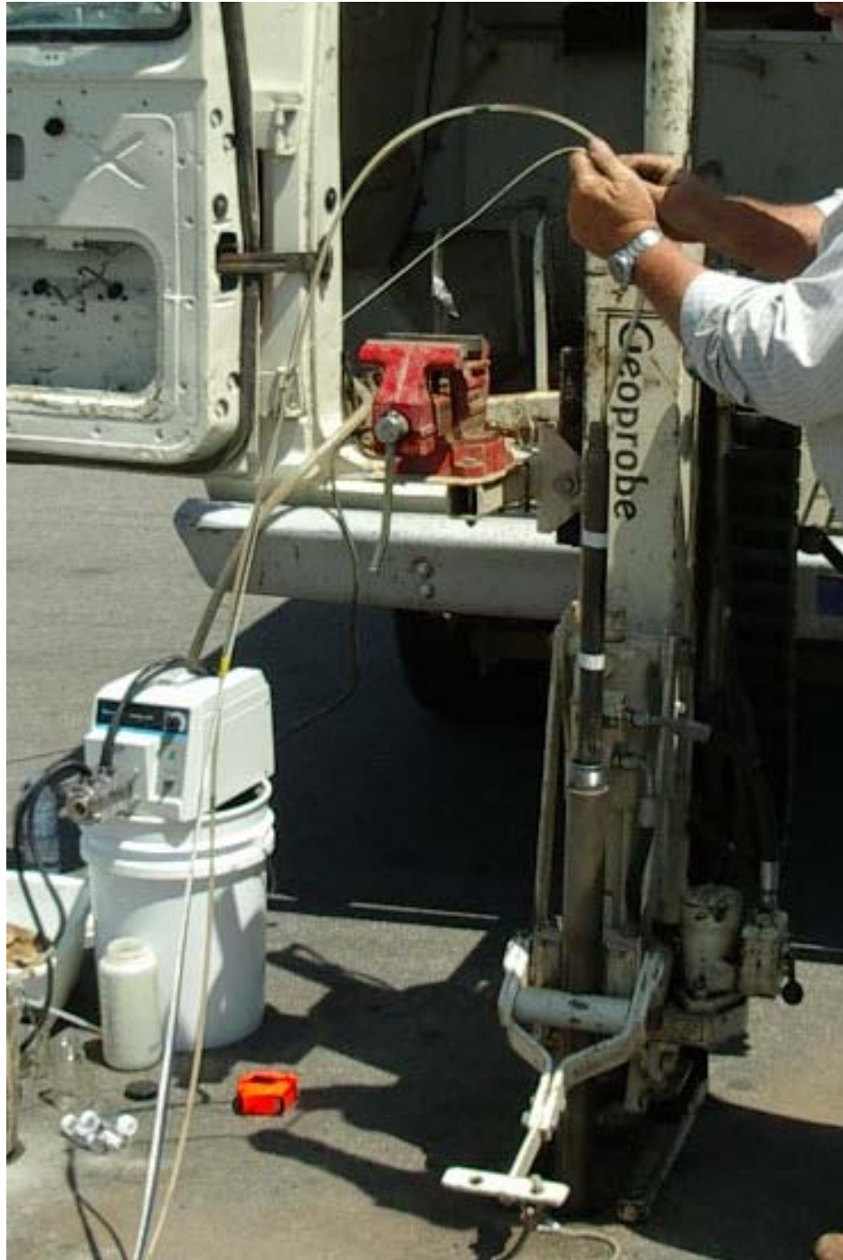
Figure D-6. Groundwater sampling with Modified Geoprobe® Groundwater Profiler.
