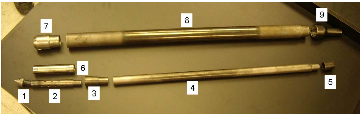
Figure D-1a. Modified Geoprobe® Groundwater Profiler - Components.
