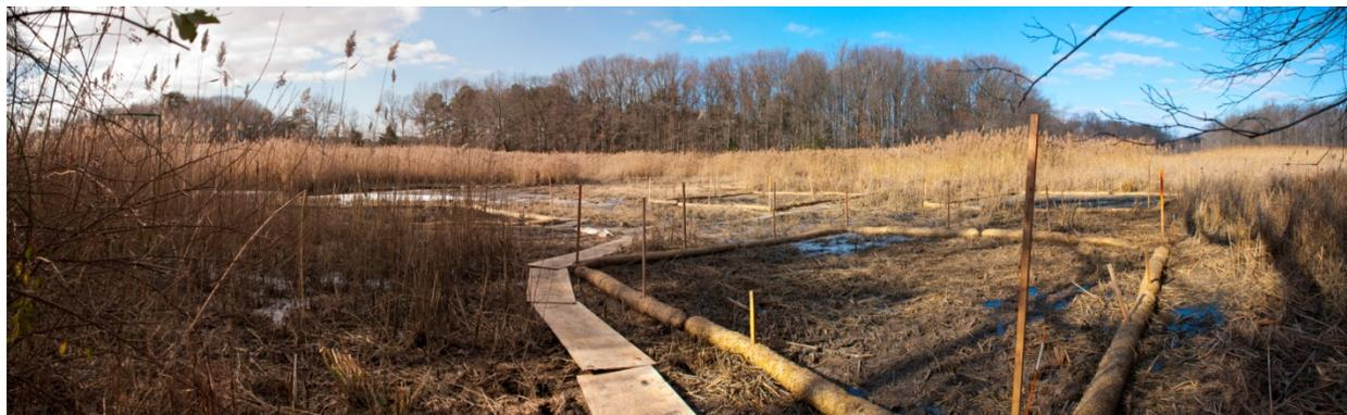
**Figure 7. Cleared test plots, staked sediment control products, and temporary walkways.**
