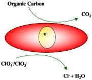
contaminated water in the underground reactive zone. Because perchlorate reduction has been shown to occur anaerobically, initial research into the use of *in situ* bioremediation as a means of treating perchlorate-contaminated groundwater has focused on developing and optimizing anaerobic bioremediation.
