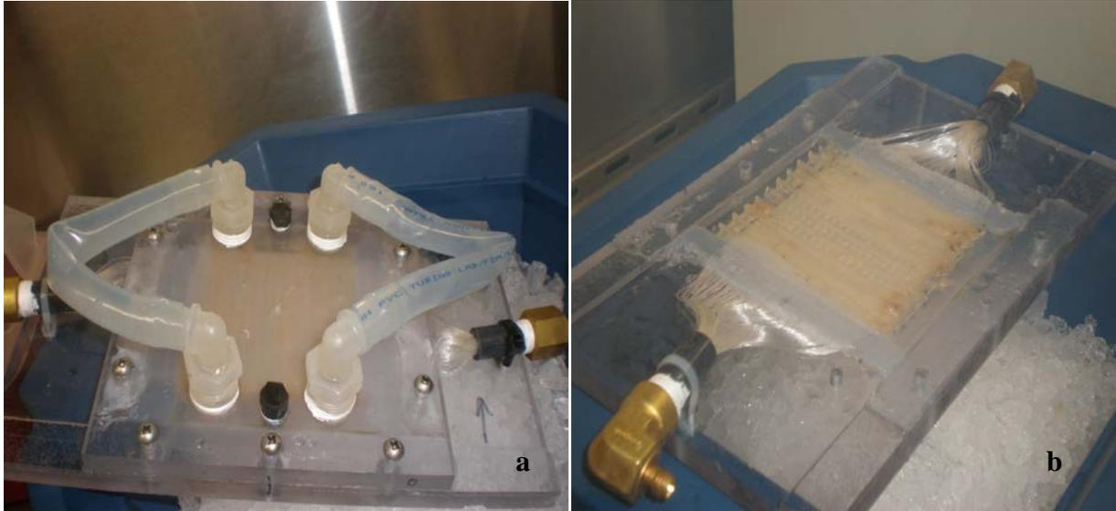
**Figure 1a** Side reactor shipped to ASU. **1b** Biomass development on the surface of fibers in the side reactor.
