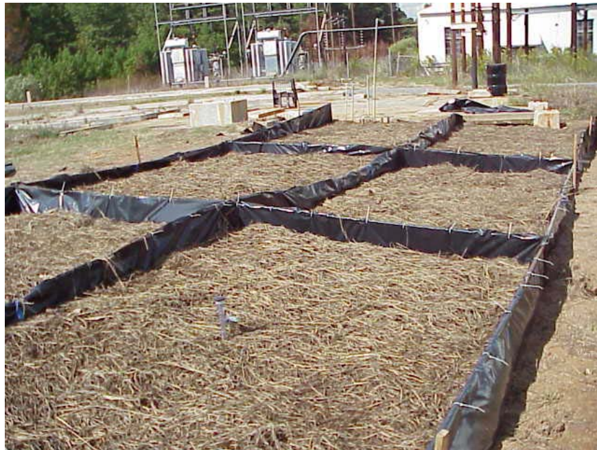
Figure 8. Tensiometers installed in the pilot scale treatment plots.
