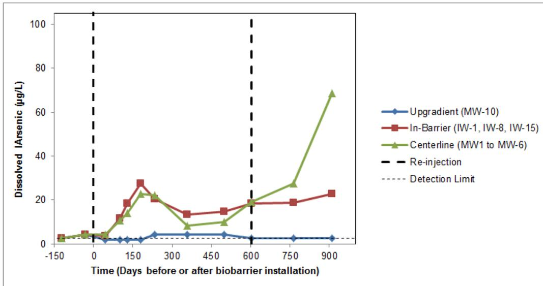
**Figure 5.23. Dissolved Arsenic (As) Concentrations over Time.**
