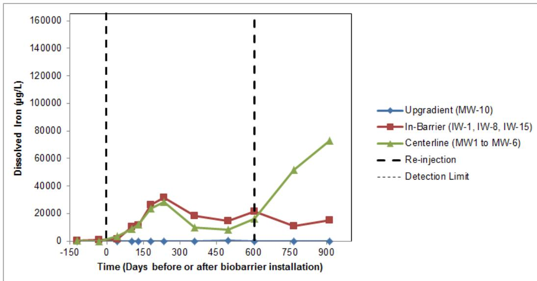
**Figure 5.21. Dissolved Iron (Fe) Concentrations over Time.**
