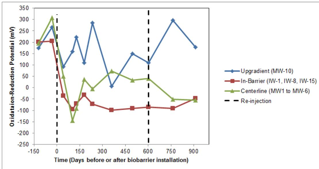
**Figure 5.9. ORP over Time in the Demonstration Plot.**
