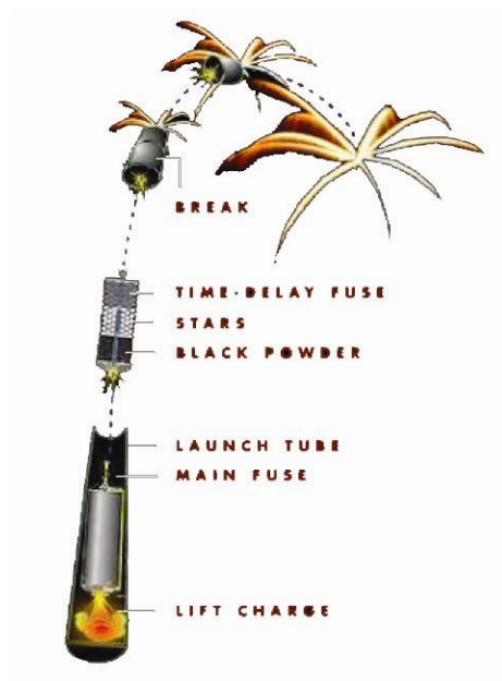
Figure 3-1: Display Firework Schematic
