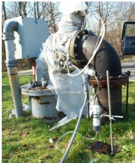
Figure 7.2. Sample collection setup for \text{ClO}_4^- from a public supply well on Long Island, New York.
