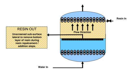
Figure 5a. Schematic of vessel for ESTCP demonstration project. Normal operation.
