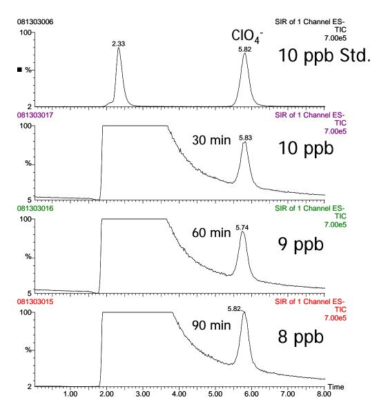
**Figure 8.** Separation of a 10 ppb perchlorate standard and three effluent samples (different collection times) that contain low ppb perchlorate levels in the presence of sulfate.
