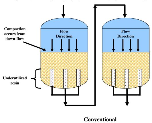
Figure 2. Typical Lead-Lag Carbon Vessel design
