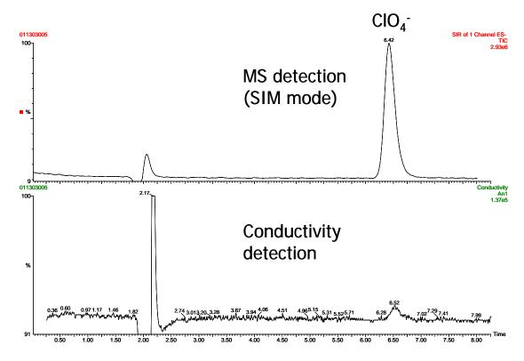
**Figure 3.** Separation of a 0.5 ppm perchlorate standard by mass spectrometry (top) and conductivity (bottom) detection modes.
