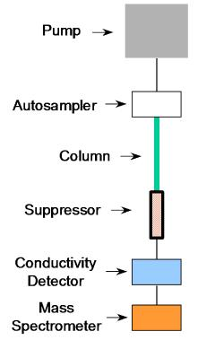
**Figure 1.** Schematic of IC/MS system.
