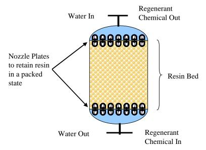
Figure 4. Typical Packed-Bed Ion Exchange Vessel.
