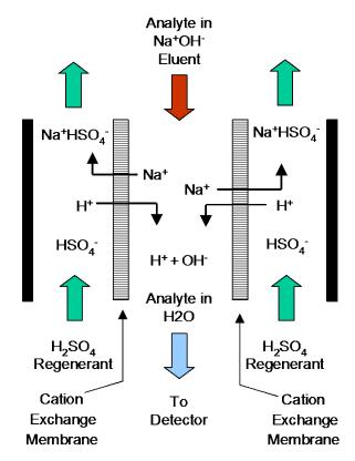
**Figure 2.** Schematic of suppressor used in anion exchange chromatography.
