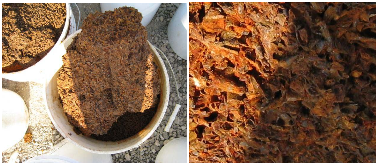
Figure 7. Pictures of large blocks (left) of ZVI taken out of the reactor when it was dismantled showing the solid structure of the ZVI bed, and close view (right) of ZVI showing the deposits of iron corrosion products and quasi total loss of porosity.
