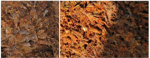
**Figure 5.13** Close views of ZVI taken out of the reactor when it was dismantled showing the heavy deposits of iron corrosion products and quasi total loss of porosity.
