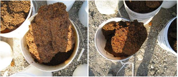
**Figure 5.12** Pictures of large blocks of ZVI taken out of the reactor when it was dismantled showing the solid structure of the ZVI bed.
