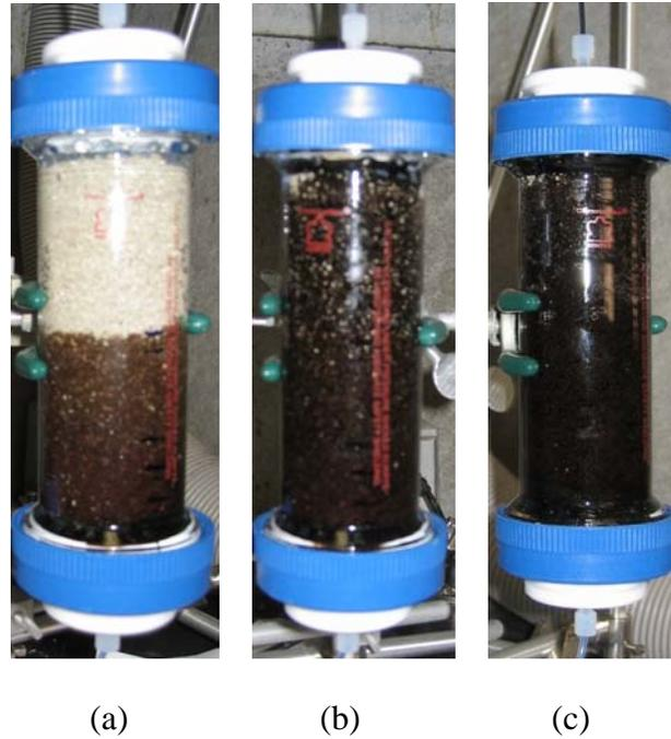
Figure 4. Intermittent pumping of FWDA-LNAPL through the 15 cm column with ET-1. (a) first 60 ml NAPL (b) more NAPL after 2.5 hr-waiting period just before breakthrough (c) more NAPL after 5 d-waiting period until breakthrough.
