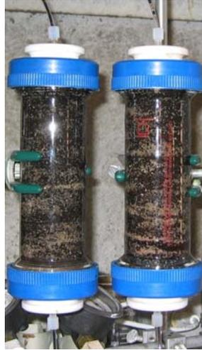
Figure 9. NAPL migration in the column with PM-200 and sand mixture (1:10): FWDA-LNAPL(right), TFA-DNAPL (left)
