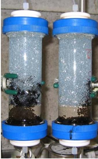
Figure 8. NAPL migration in the column with 2 cm PM-200 and 12 cm glass beads: TFA-DNAPL (left) and FWDA-LNAPL (right)
