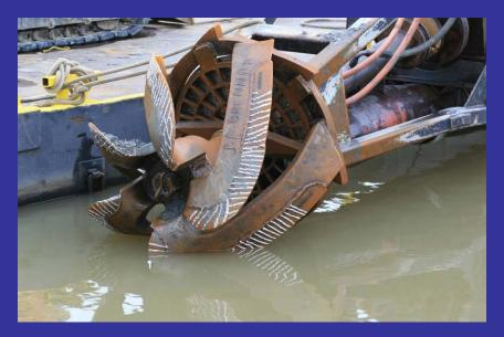
Solution: Gatling Plate and Shear Bar
